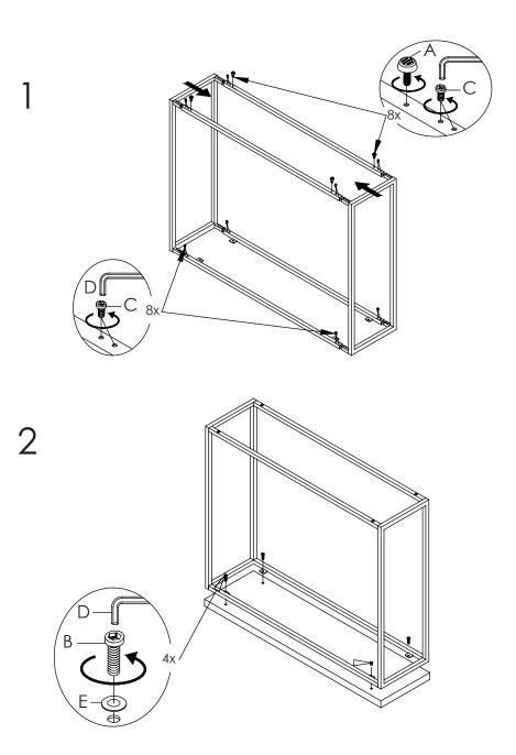
During assembly, hand tighten screws only. When all screws are in place, then tighten completely.
