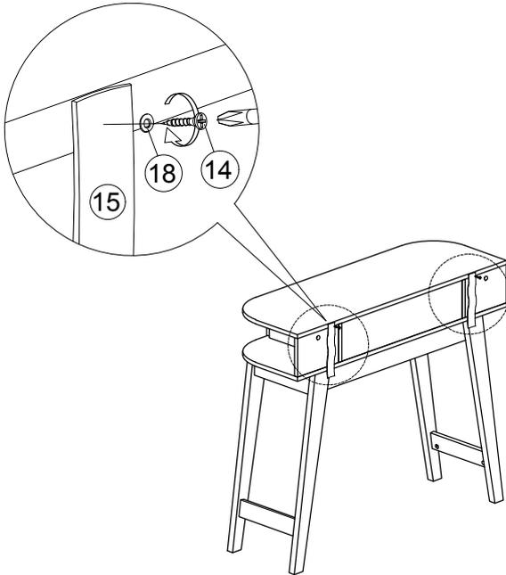
4. Add safety strap (15), washer (18) using 3.5x16mm screw (14) to back of cabinet.
