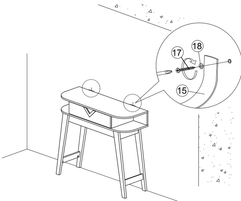
5. Finally, attach safety strap (15) and washer (18) using 4x30mm screw (17) to the wall.
