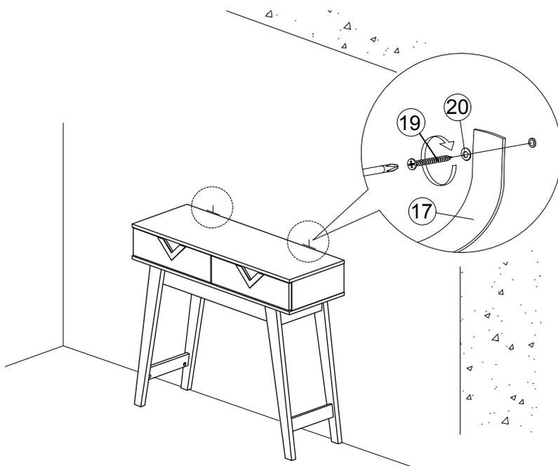
5. Finally, attach safety strap (17) and washer (20) using 4x30mm screw (19) to the wall.
