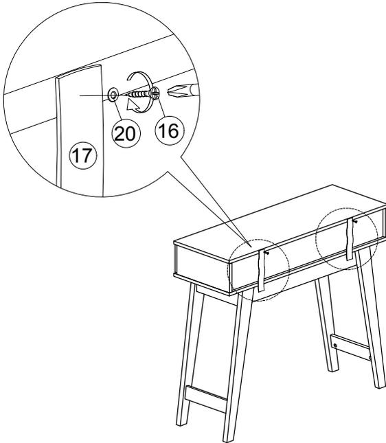
4. Add safety strap (17), washer (20) using 3.5x16mm screw (16) to back of cabinet.
