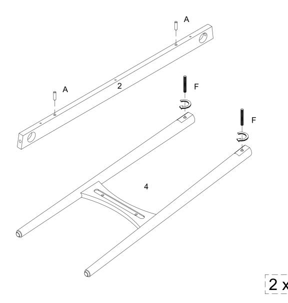
Insert wooden dowel (A) into part (2) and secure bolt (F) into part (4) as per diagram.
