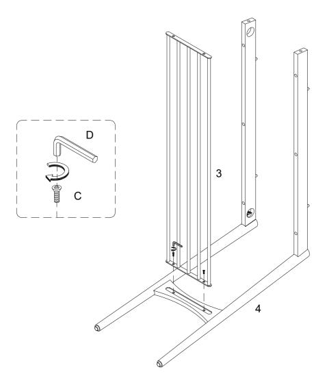
Using bolt (C) attach part (3) to part (4) with Hex key (D) as per diagram. Note:Do not fully tighten all bolts.
