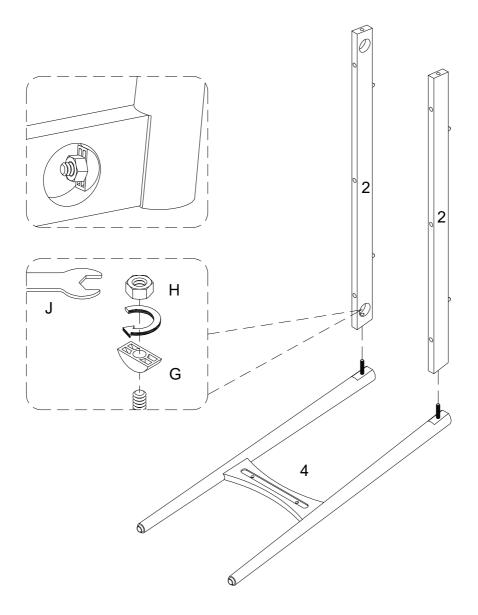
Using washer (G) and Nut (H) secure part (2) into part (4) with Wrench (J) as per diagram.
