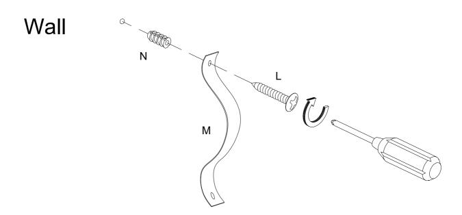
Using screw (L) attach Velcro strap (M) into Nut (N) to wall with Philips head screwdriver as per diagram.
