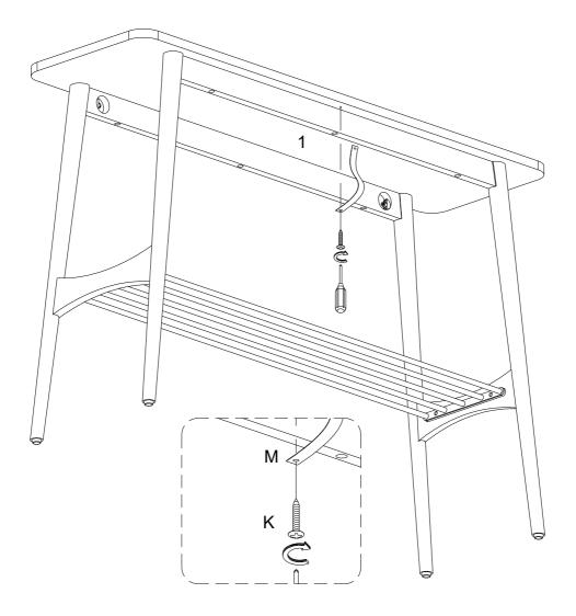
Using screw (K) attach Velcro strap (M) into part (1) with Philips head screwdriver as per diagram.
