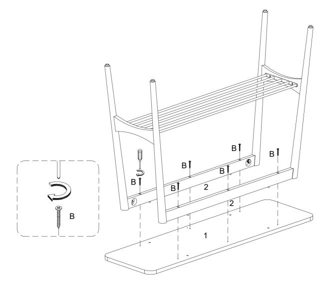
Using Flat head screw(B) secure part (2) to part (1) with Philips head screwdriver as per diagram. Note: Fully tighten all bolts.
