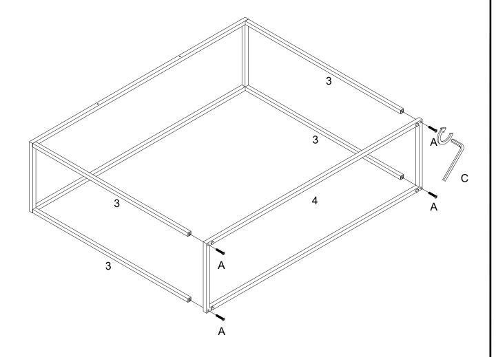
Using Bolts (A) attach part (4) to part (3) with hex key (C) as per diagram. Note: Fully tighten all the bolts .
