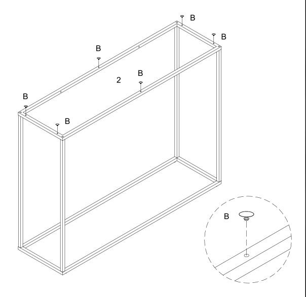
Secure Rubber suction cups (B) into part (2) as per diagram.
