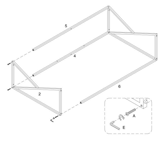
Using bolt (A) attach part (2) to parts (4,5,6) with Hex key (E) as per diagram.
