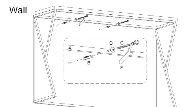
Using screw (C) insert Flat washer (D) attach part (4) into Nut (B) to wall with Wrench (F) as per diagram.
