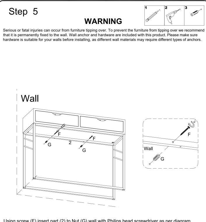
Using screw (F) insert part (2) to Nut (G) wall with Philips head screwdriver as per diagram.
