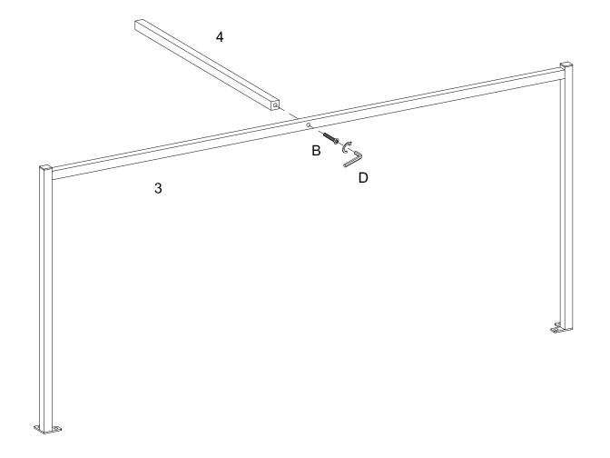
Using bolt (B) attach part (3) to part (4) with Hex key (D) as per diagram. Note: Please do not fully tighten all bolts.
