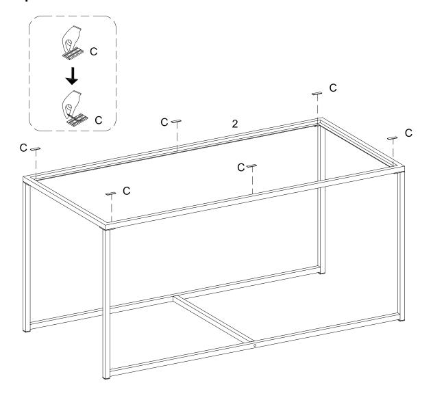
Tear off the glass pad (C) and place on the top of metal frame as per diagram.
