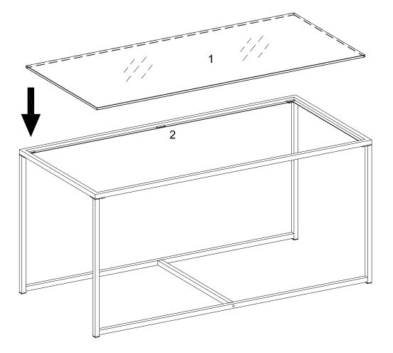
Place part (1) on the top of part (2) carefully as per diagram.
