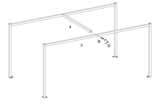
Using bolt (B) attach part (3) to part (4) with Hex key (D) as per diagram.
