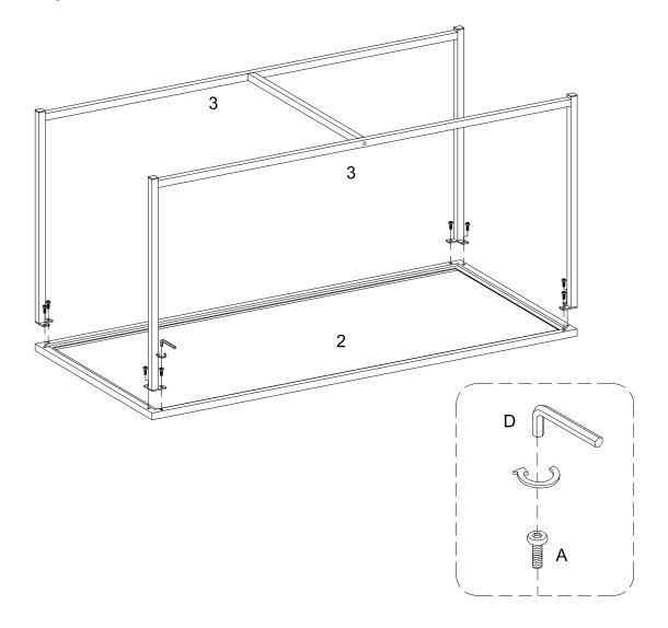
Using bolt (A) attach part (3) to part (2) with Hex key (D) as per diagram. Note: Fully tighten all bolts.
