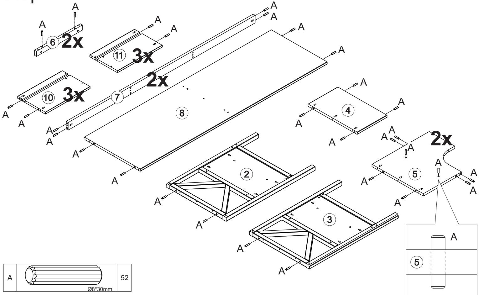
Insert Wooden dowel (A) into part (2), (3), (4), (5), (6), (7), (8), (10) and (11).
