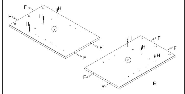
Insert wood dowels (F) into parts (2,3).
