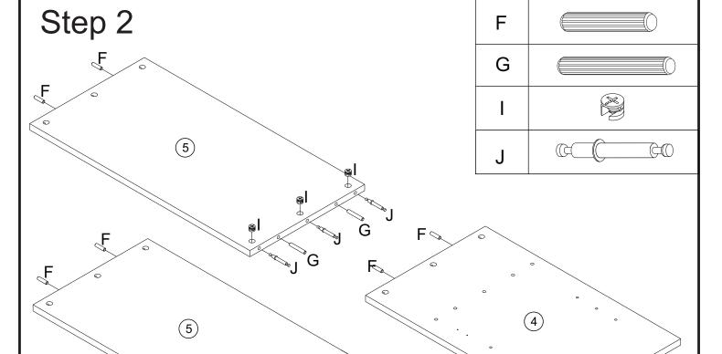
Insert wood dowels (F) into parts (5,4).
