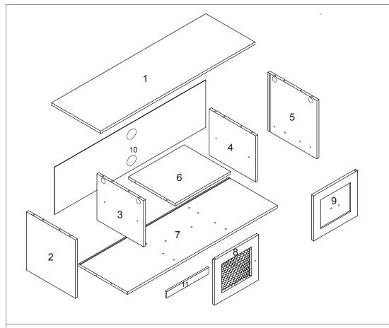
Attach piece 7 to piece 11 using wooden dowels (F), screw (C), insert hardware parts (O) into piece 11.
