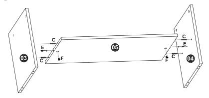
• Connect the Shelf (05) into the Left Side Panel (03) and Partition (04) using dowels (C) and the cam lock hardware (E + F).
