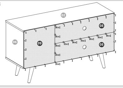
• Connect Back Panels (08) and (09) with nails (I). At the joining surfaces, use metallic plates (H) and nails (I).
