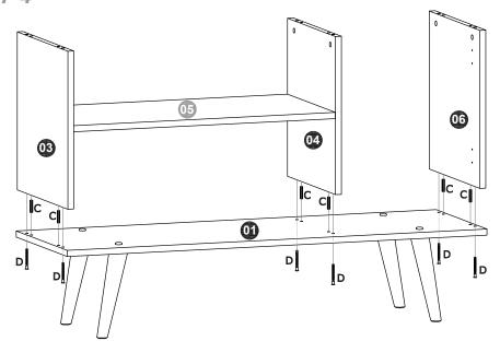
• Connect Side Panels (03) and (06) and Partition (04) into the Base (01) with dowels (C) and bolts (D).
