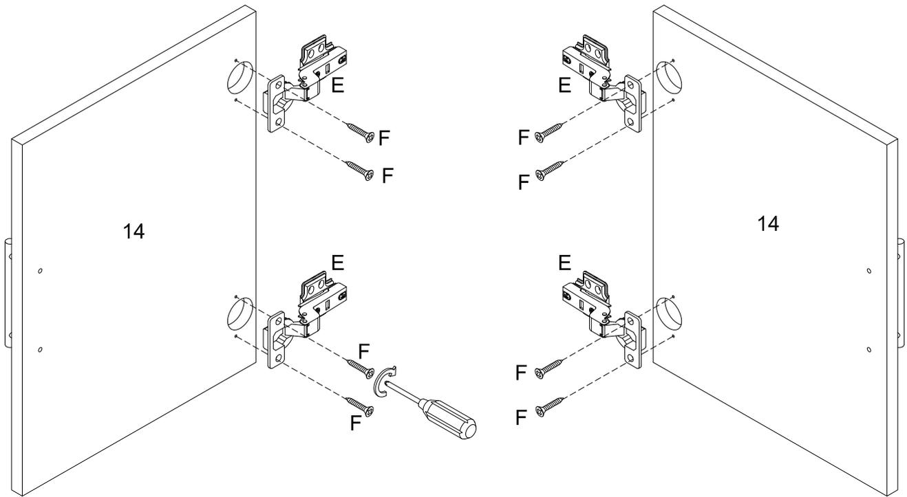
Using screw (F) attach Europe hinge (E) into part (14) with Philips head screwdriver as per diagram.
