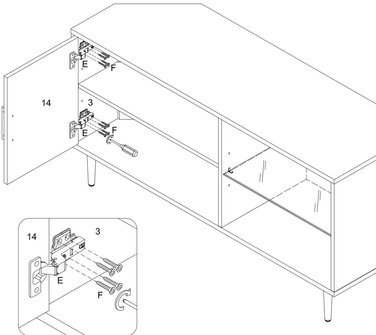
Using screw (F) attach Europe (E) into part (3) with Philips head screwdriver as per diagram.
