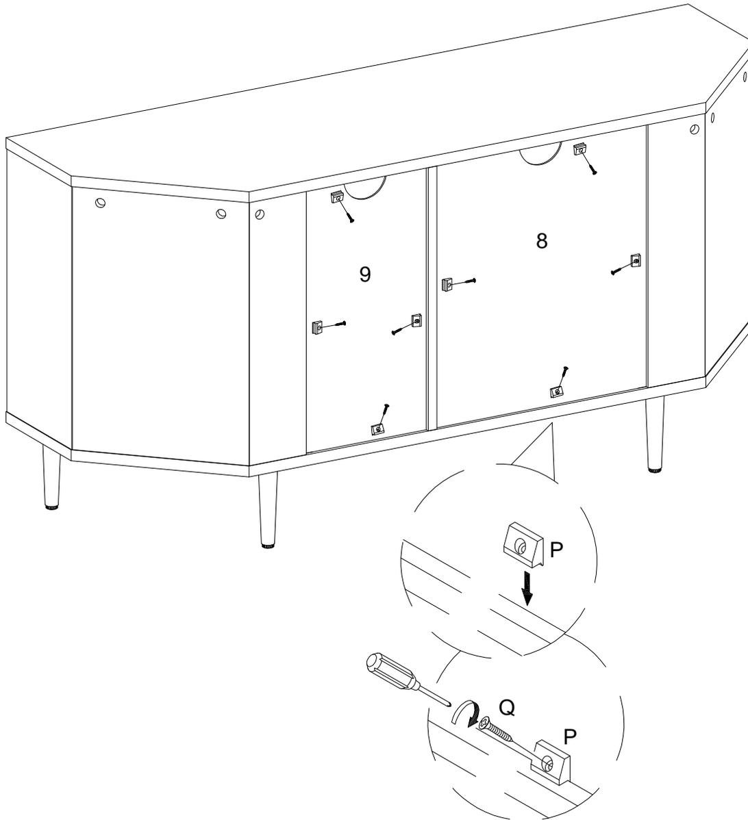
Using screw (Q) secure plastic wedge (P) to fix parts (8,9) with Philips head screwdriver as per diagram .
