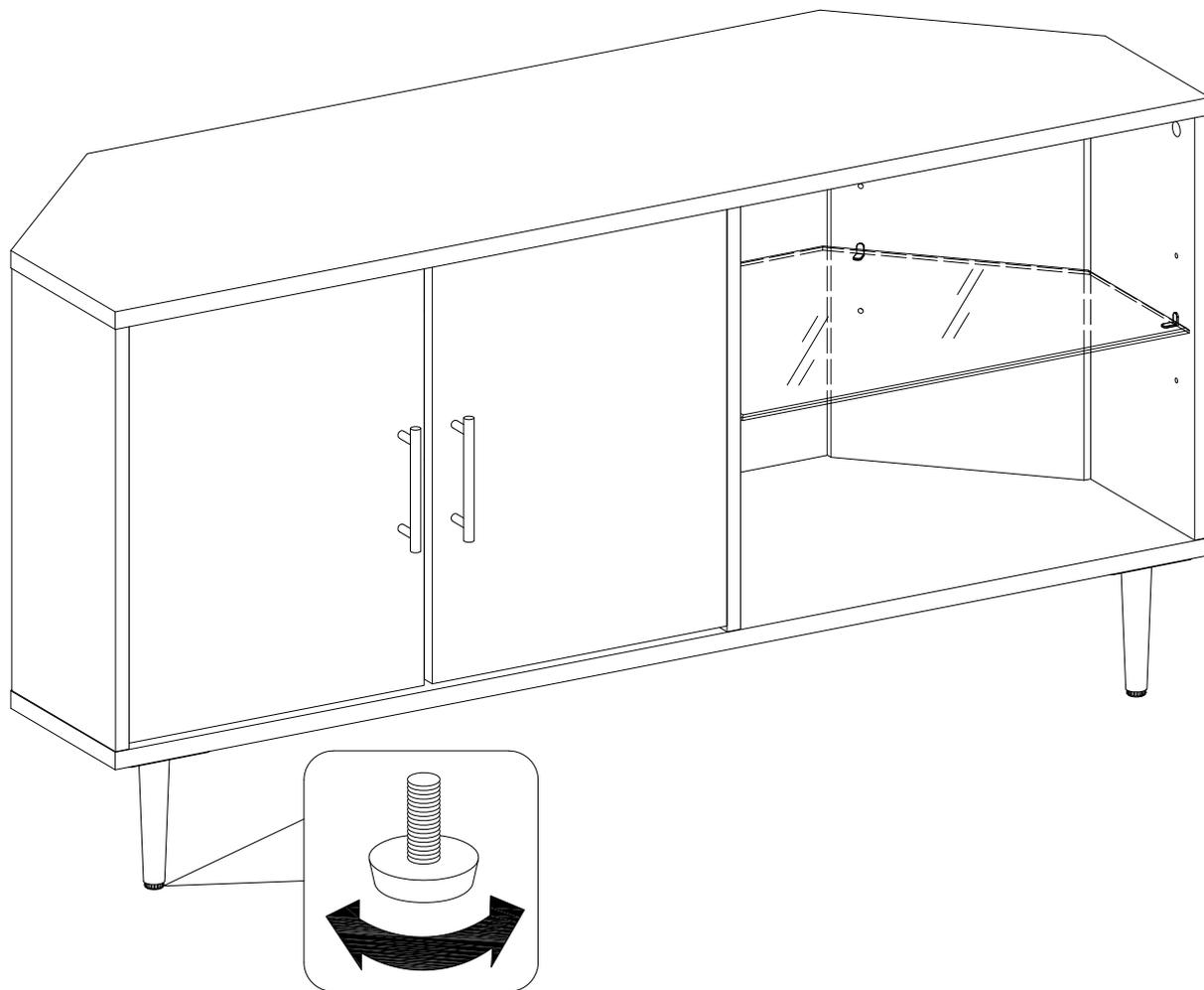
Position the assembled unit at the deaired location. If necessary adjust the floor levelers at the bottom of legs to level the unit .
