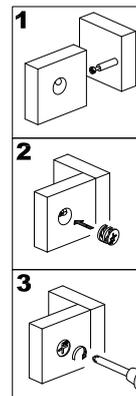
Using cam lock(C) secure part (1) to parts (3,4,5,6,7,10,11) with Philips head screwdriver as per diagram. Please make sure parts (8,9) into the groove of part (1).
