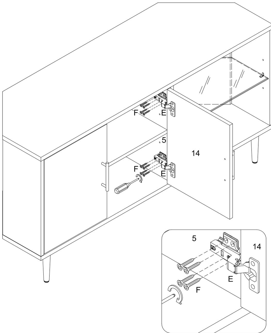
Using screw (F) attach Europe (E) into part (5) with Philips head screwdriver as per diagram. Close and open the doors to make sure they are shut correctly .If necessary ,adjust the screws (F) for a good fit .
