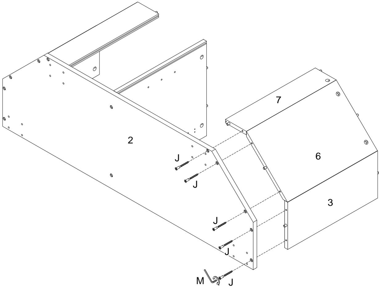
Using screw (J) attach part (2) into parts (3,6,7) with hex key (M) as per diagram.
