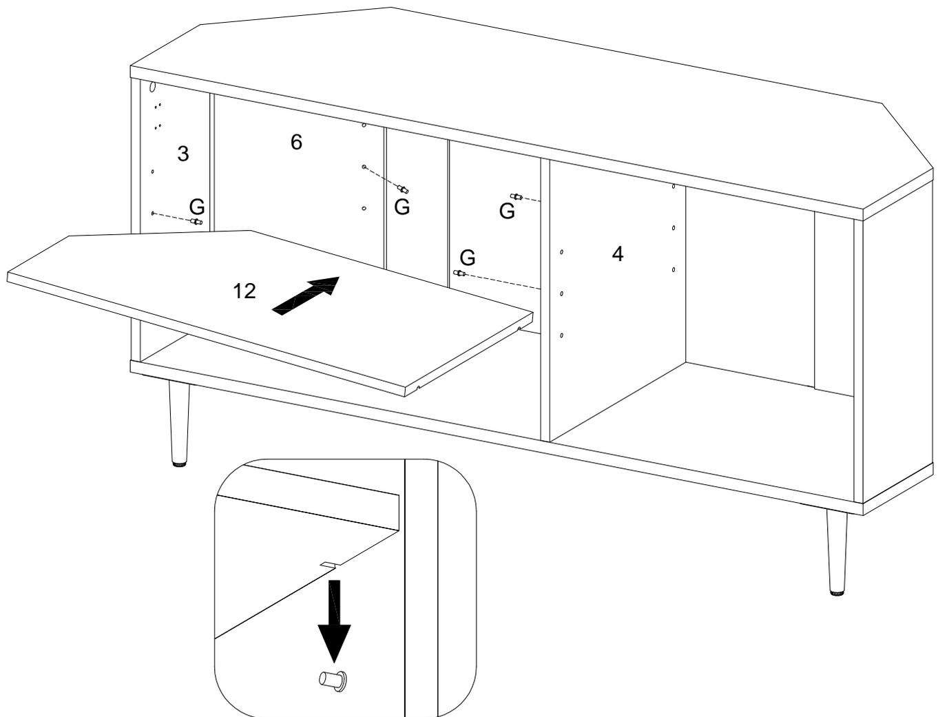
Insert shelf support pin (G) into parts (3,4,6) as per diagram. Make sure you place the four shelf support pins (G) in the same level. So the shelf is not titled .Put part (12) into unit as per diagram. Tilt and rest the adjustable shelf(12) onto the shelf support pins .
