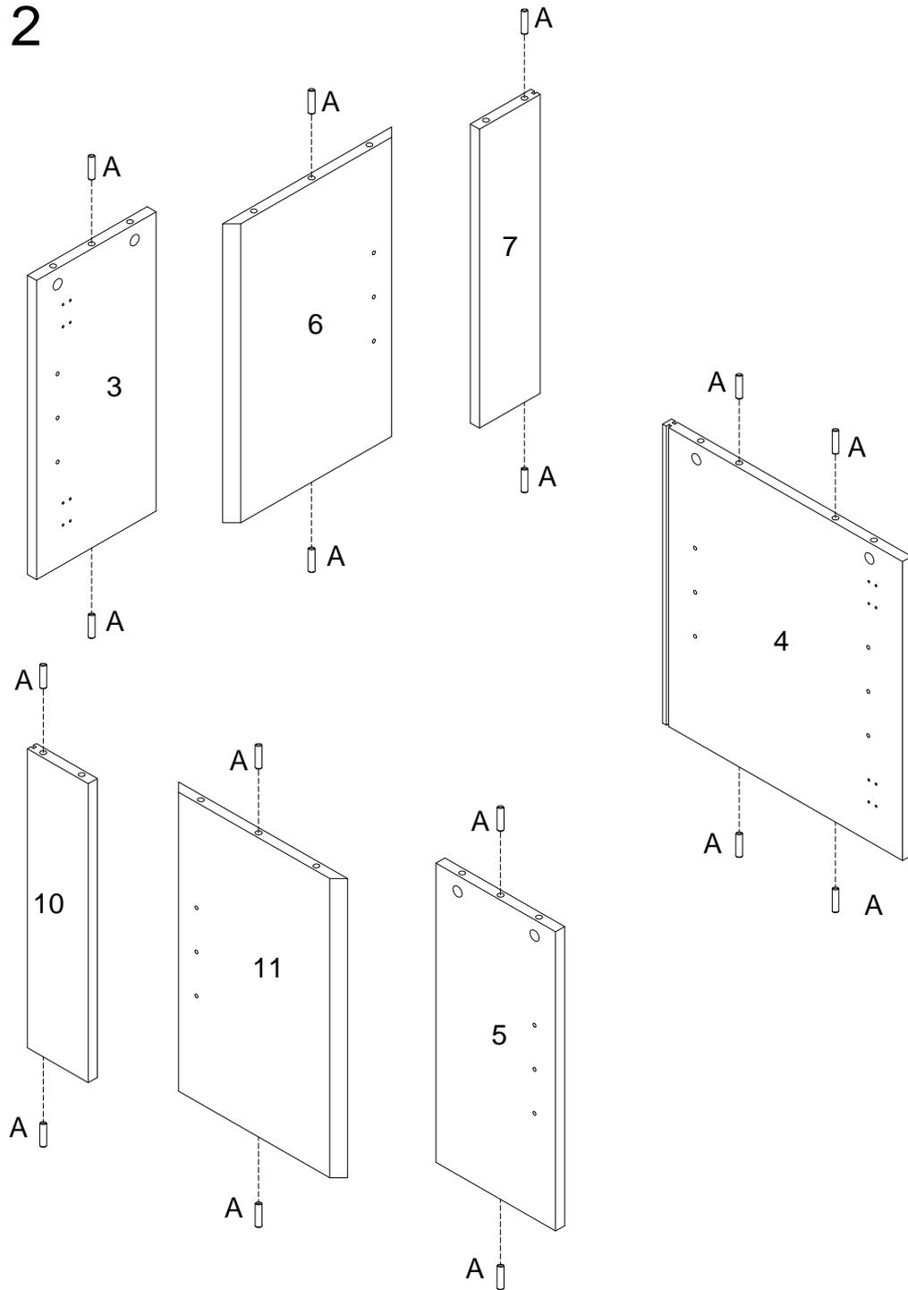
Insert wooden dowel (A) into parts (3,4,5,6,7,10,11) as per diagram.
