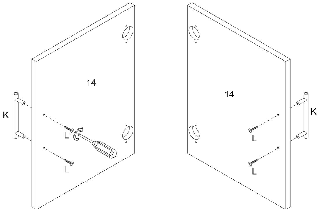
Using screw (L) attach handle (K) into part (14) with Philips head screwdriver as per diagram.
