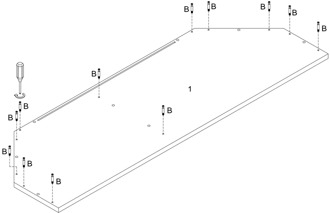
Using cam bolts (B) secure part (1) with Philips head screwdriver as per diagram.
