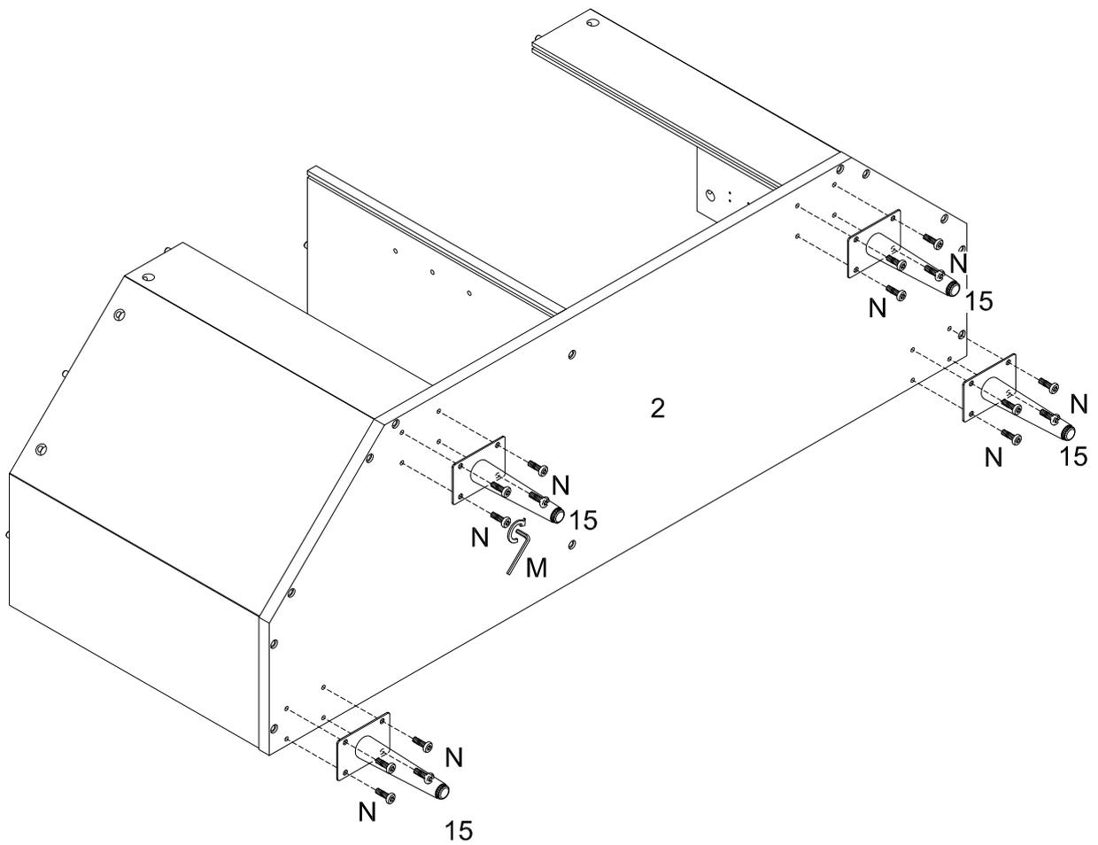
Using bolt (N) attach part (15) to part (2) with hex key (M) as per diagram.
