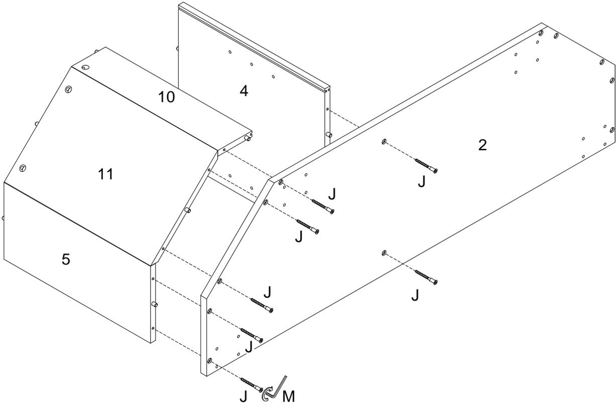
Using screw (J) attach part (2) into parts (4,5,10,11) with hex key (M) as per diagram.
