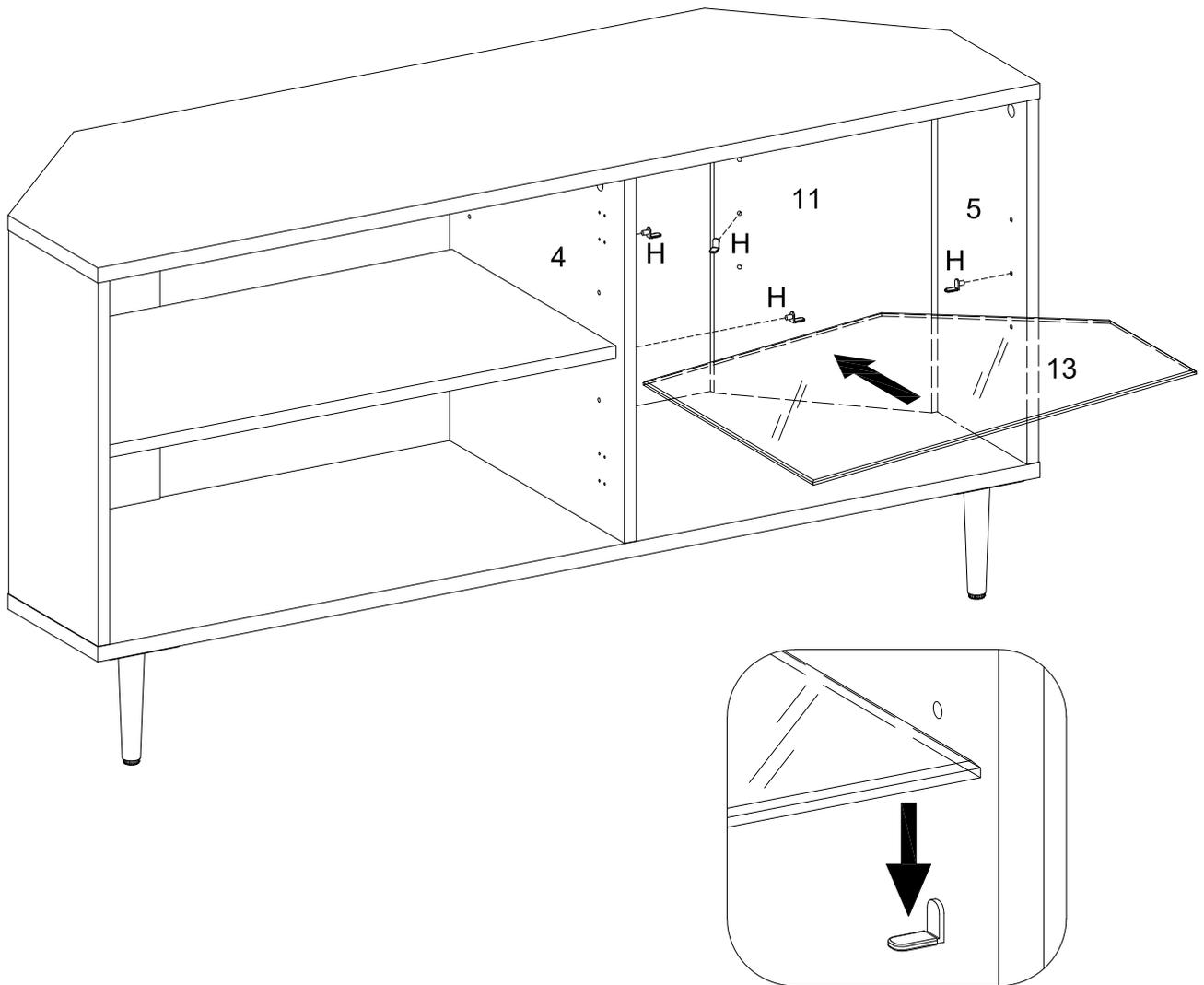
Insert L shape shelf support pins (H) into parts (4,5,11) as per diagram .Make sure you place the four shelf support pins (H) in the same level .so the shelf is not titled. Put glass shelf (13) into the unit as per diagram. Titled and rest the adjustable glass shelf (13) onto the shelf support pins as per diagram .
