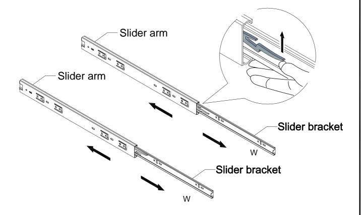
Pick up the slider arm (W) and separate the slide Runner for the following Steps. Extend the Slide .Runner all the way forward,press the plastic release lever of the alider arm up and pull the Slide Runner Complete out .
