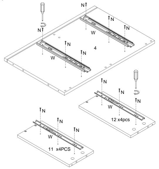
Using screw (N) attach slider (W) into parts (4,11,12) with Philips head screwdriver as per diagram.
