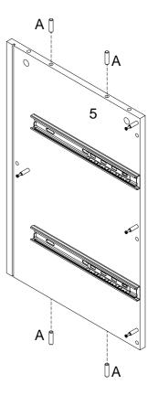
Insert wooden dowel (A) into parts (3,4,5) as per diagram.
