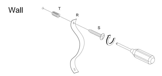
Using screw (S) attach plastic strap (R) into nut (T) to wall with Philips head screwdriver as per diagram.
