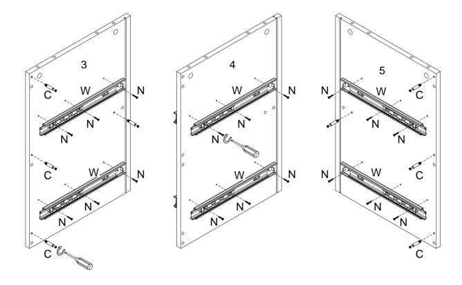
Using Cam bolt (C) secure parts (3,5) ,then using screw (N) attach slider(W) into parts (3,4,5) with Philips head screwdriver as per diagram.
