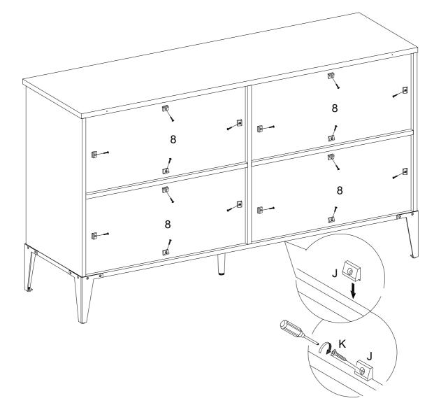
Using screw (K) secure plastic wedge (J) to part (8) with Philips head screwdriver as per diagram.
