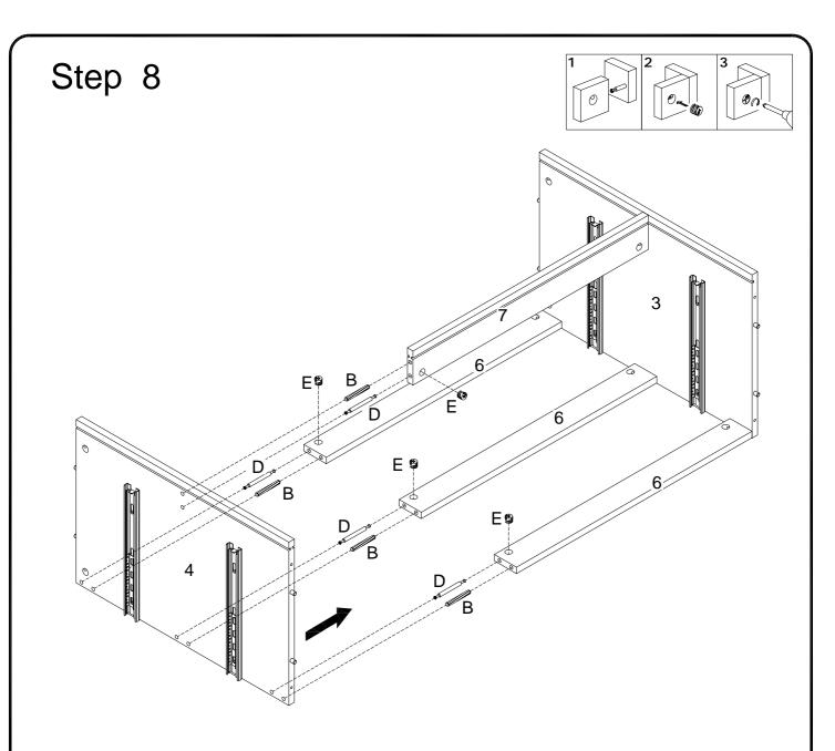
Insert wooden dowel (B) and cam bolt (D) into parts (6,7) first, then insert partition board (4) to parts (6,7), then insert and secure cam lock (E) to parts (6,7) to lock it.
