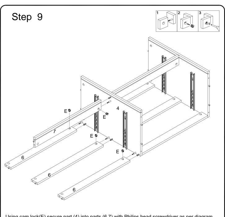
Using cam lock(E) secure part (4) into parts (6,7) with Philips head screwdriver as per diagram.
