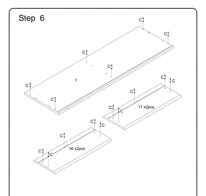
Secure cam bolt (C) into parts (1,16,17) with Philips head screwdriver as per diagram.
