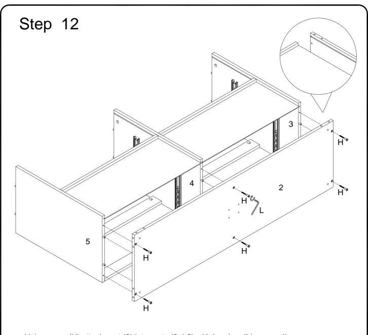
Using screw(H) attach part (2) into parts (3,4,5) with hex key (L) as per diagram.
