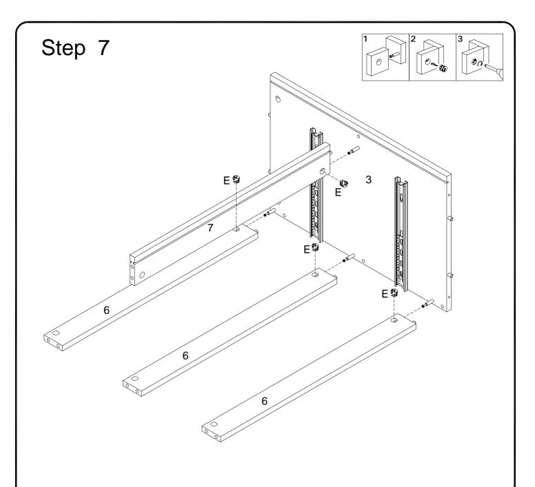
Using cam lock(E) secure parts (6,7) into part (3) with Philips head screwdriver as per diagram.
