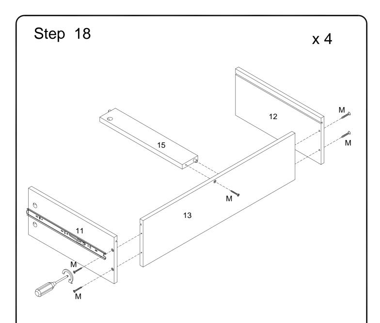
Using screw (M) attach parts (11,12,15) into part (13) with Philips head screwdriver as per diagram.
