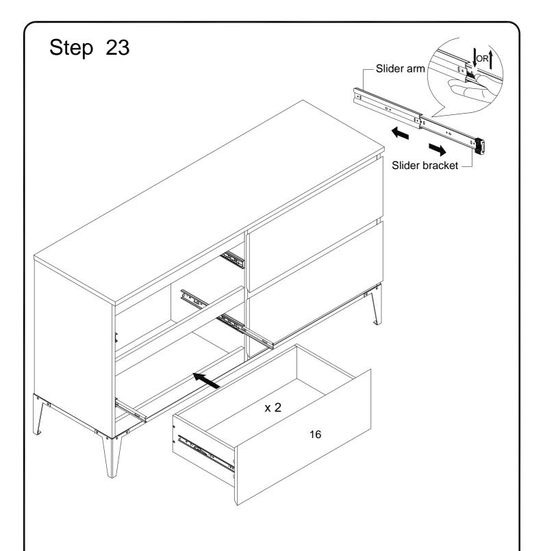
Insert the assembled drawer (16) into the unit frame, extend the Ball Bearing Slide Tracks on the pedestal Side Panel all the way forward .Then align the Slide Runners on the assembled drawers with the Slide Tracks and push the drawer carefully inside until it stops.
