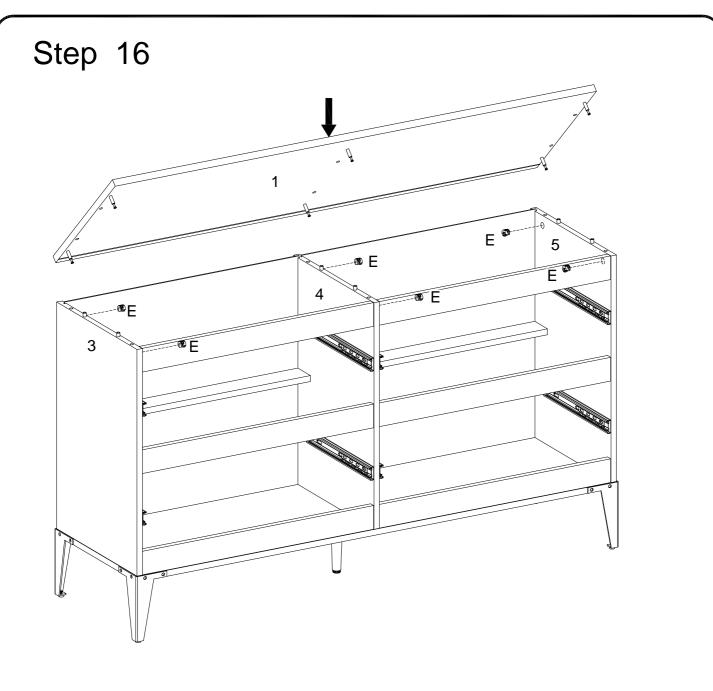
Using cam lock(E) secure part (1) to parts (3,4,5) with Philips head screwdriver as per diagram.
