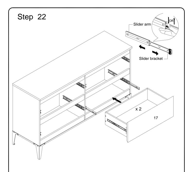
Insert the assembled drawer (17) into the unit frame, extend the Ball Bearing Slide Tracks on the pedestal Side Panel all the way forward .Then align the Slide Runners on the assembled drawers with the Slide Tracks and push the drawer carefully inside until it stops.
