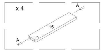
Insert wooden dowel (A) into parts (6,7,15) as per diagram.
