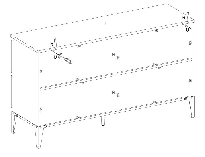
Using screw (U) attach plastic strap (R) into part (1) with Philips head screwdriver as per diagram.
