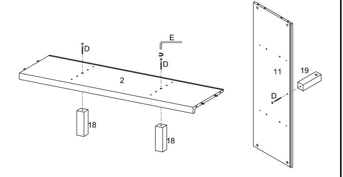
Use wrench (E) to secure leg (18) to bottom panel (2) with bolt (D), and secure part (19) to shelf (11).
