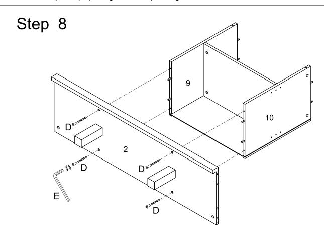
Use wrench (E) to secure bottom panel (2) to side panel (9,10) with bolt (D).
