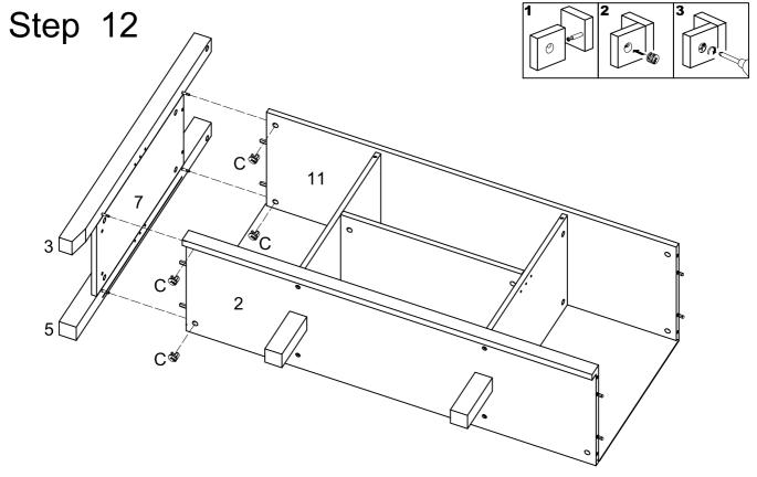
Insert bottom panel (2) and shelf (11) into side panel (7) and part (3,5), then insert and secure cam lock (C) to bottom panel (2) and shelf (11) to lock it.
