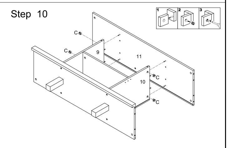
Insert side panel (9,10) into shelf (11), then insert and secure cam lock (C) to side panel (9,10) to lock it.
