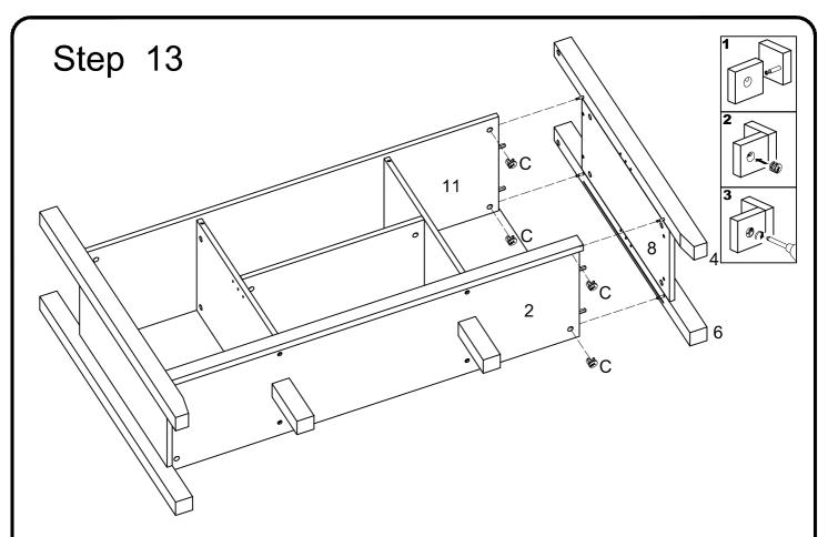
Insert bottom panel (2) and shelf (11) into side panel (8) and part (4,6), then insert and secure cam lock (C) to bottom panel (2) and shelf (11) to lock it.
