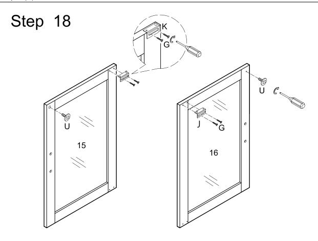
Secure bolt (U) to door (15,16), door hinge (J) to door (16) and door hinge (K) to door (15) with screw (G).
