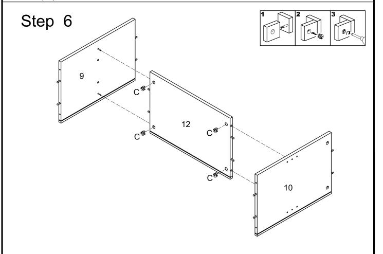
Insert shelf (12) into side panel (9,10), then insert and secure cam lock (C) to shelf (12) to lock it.
