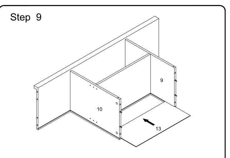
Slide back panel (13) into grooves as per diagram.
