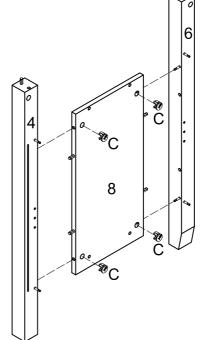
Insert side panel (7,8) into part (3,4,5,6), then insert and secure cam lock (C) to side panel (7,8) to lock it.
