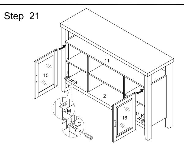
Insert door hinge (J,K) into panel hole as per diagram. Slide door (15,16) onto door hinge (J,K) as shown in diagram and secure it with screw (G).
