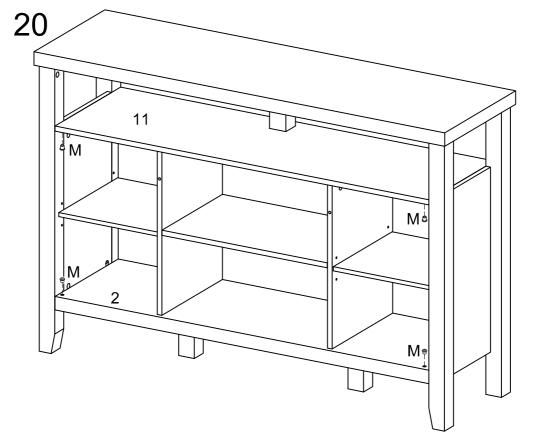
Place plastic pivot (M) over holes as per diagram.
