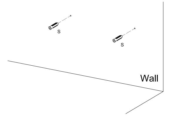
Place unit in desired location and mark the wall for anchor location. Insert plug (S) into wall as per diagram.
