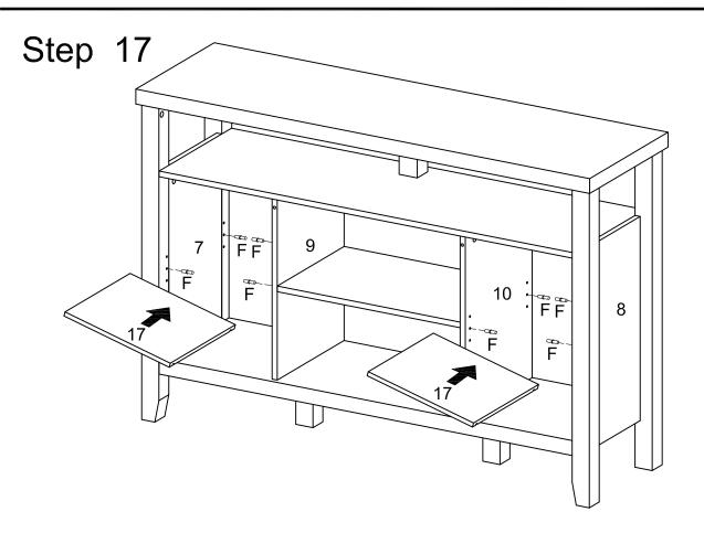
Insert shelf support pin (F) into side panel (7,8,9,10), then place shelf (17) on top of support pin (F).
