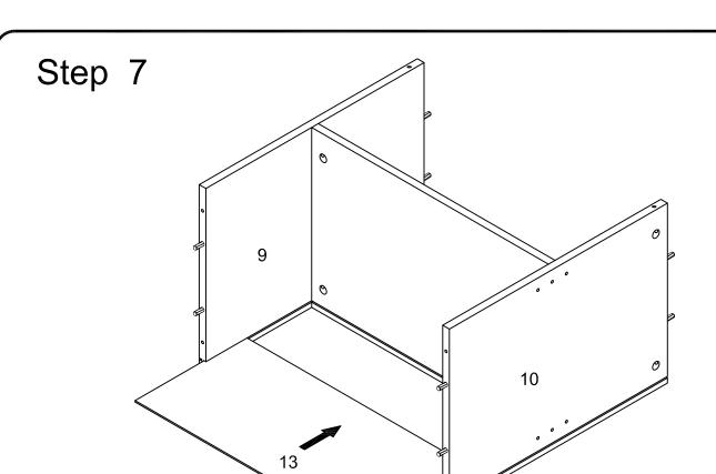
Slide back panel (13) into grooves as per diagram.
