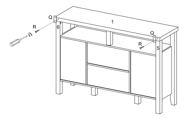
Secure flat plate (Q) to as shown in diagram with screw (R).
