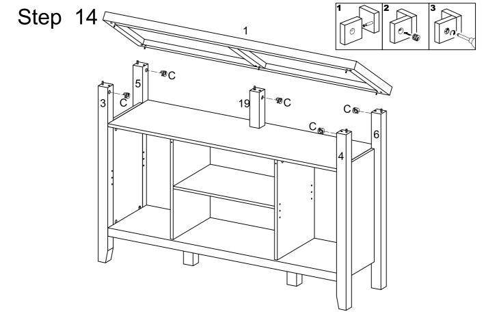
Insert top panel (1) into part (3,4,5,6,19), then insert and secure cam lock (C) to part (3,4,5,6,19) to lock it.
