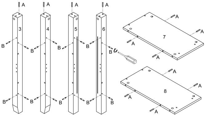
Insert wooden dowel (A) to part (3,4,5,6), and side panel (7,8). Secure cam bolt (B) to part (3,4,5,6).
