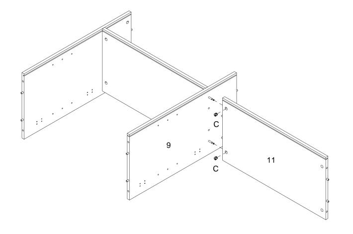
Using cam lock (C) secure part (11) to part (9) with Philips head screwdriver as per diagram .
