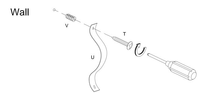
Insert screw (T) into plastic strap (U) to nut (V) secure with Philips head screwdriver as per diagram
