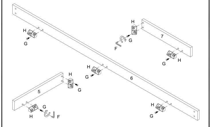
Using bolt (G) secure plastic wedge (H) to parts (5,6,7) with hex key (F) as per diagram.
