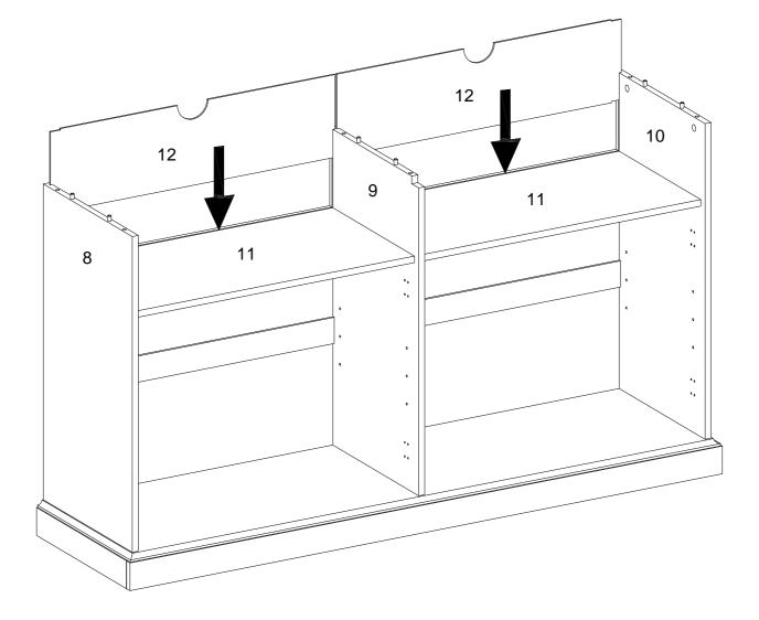
Insert part (12) to parts (8,9,10,11) as per diagram.
