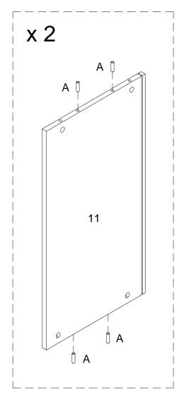
Insert wooden dowel (A) to part (8,10,11), then using cam bolt (B) secure part (8,10,11) with Philips head screwdriver as per diagram .
