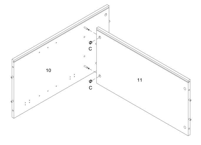
Using cam lock (C) secure part (11) to part (10) with Philips head screwdriver as per diagram .
