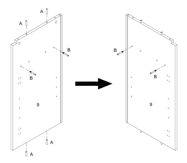
Insert wooden dowel (A) and cam bolt (B) to part (9) as per diagram .
