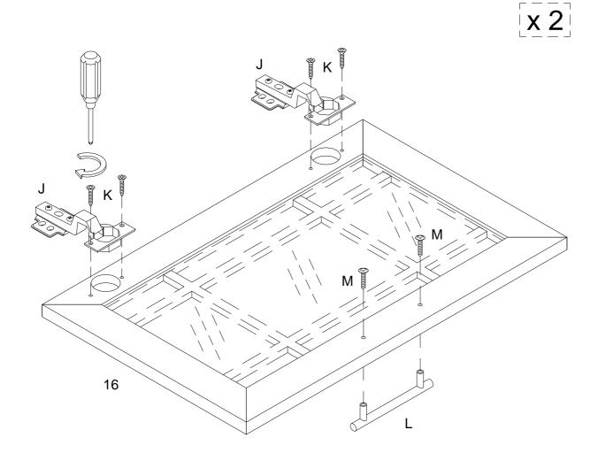
Using screw (K) secure west hinge (J) to part (16), then using bolt (M) secure part (17) to knob (L) with Philips head screwdriver as per diagram.
