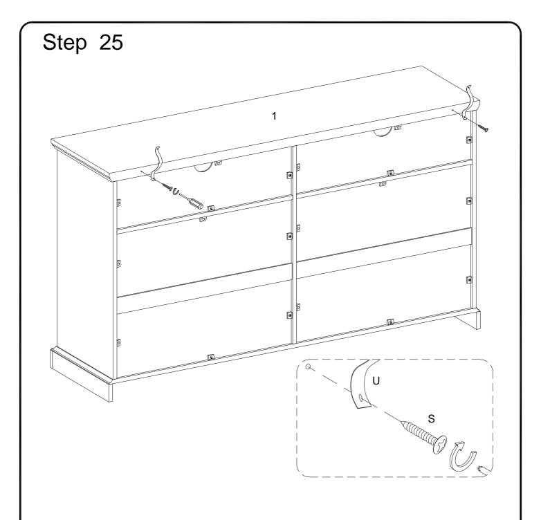
Insert screw (S) into plastic strap (U) to part (1) with Philips head screwdriver as per diagram .
