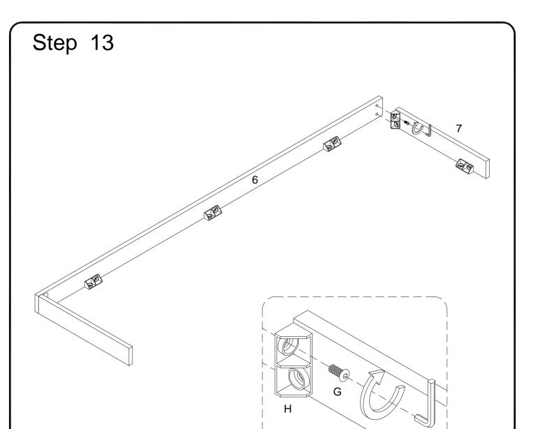
Using bolt (G) secure plastic wedge (H) to parts (6,7) with hex key (F) as per diagram.
