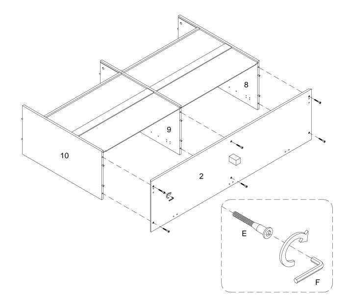
Using screw (E) secure part (2) to part (8,9,10) with hex key (F) as per diagram.
