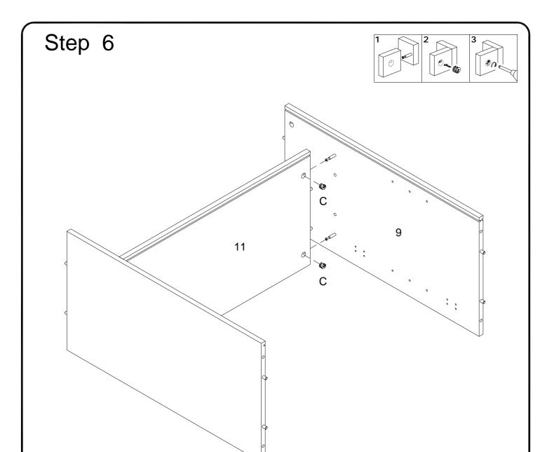
Using cam lock (C) secure part (11) to part (9) with Philips head screwdriver as per diagram .
