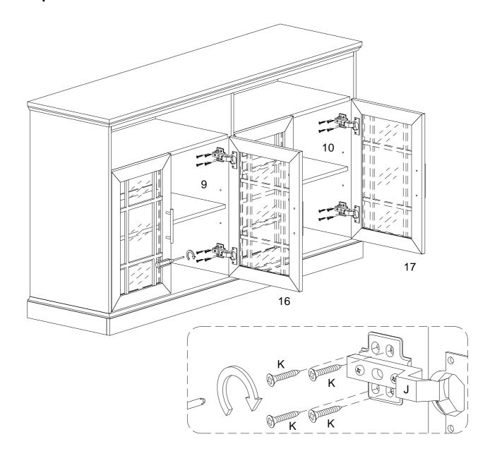
Using screw (K) secure west hinge (J) into part (9,10,16,17) with Philips head screwdriver as per diagram.
