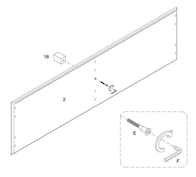
Using screw (E) secure part (2) to part (18) with hex key (F) as per diagram .
