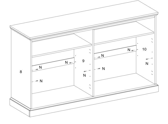
Insert shelf support pin (N) to parts (8,9,10) as per diagram .
