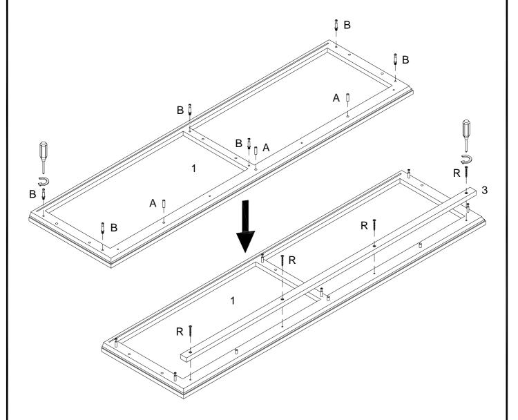
Using wooden dowel (A) and cam bolt (B) to part (1) secure with Philips head screwdriver . then using screw (R) secure part (3) to part (1) with Philips head screwdriver as per diagram .
