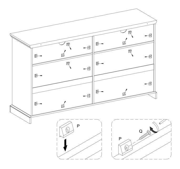
Using screw (Q) secure plastic wedge (P) to case with Philips head screwdriver as per diagram.
