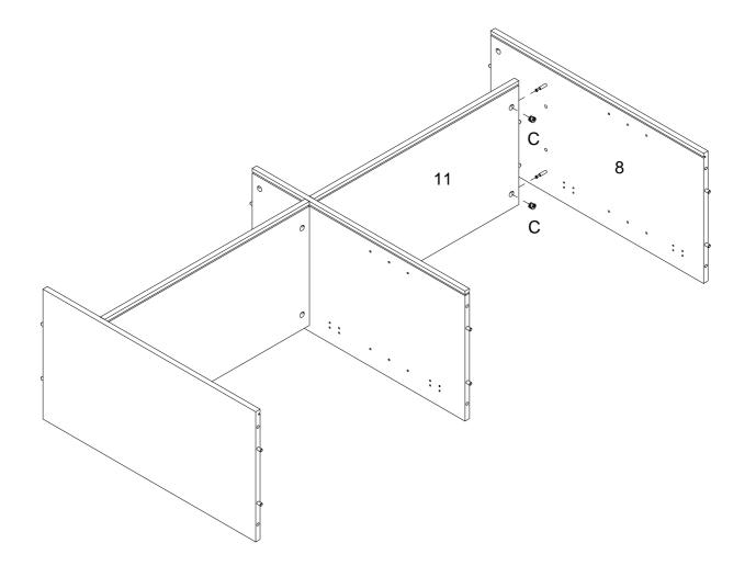
Using cam lock (C) secure part (11) to part (8) with Philips head screwdriver as per diagram .
