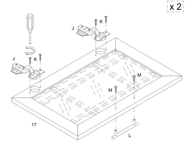
Using screw (K) secure west hinge (J) to part (17), then using bolt (M) secure part (17) to knob (L) with Philips head screwdriver as per diagram.
