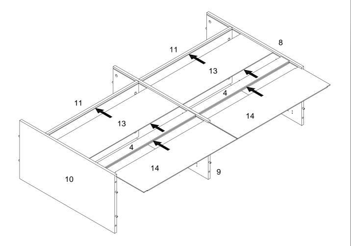
Insert parts (13,14) to part (4,8,9,10,11) as per diagram.
