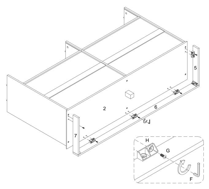
Using bolt (G) secure plastic wedge (H) to parts (2,5,6,7) with hex key (F) as per diagram.
