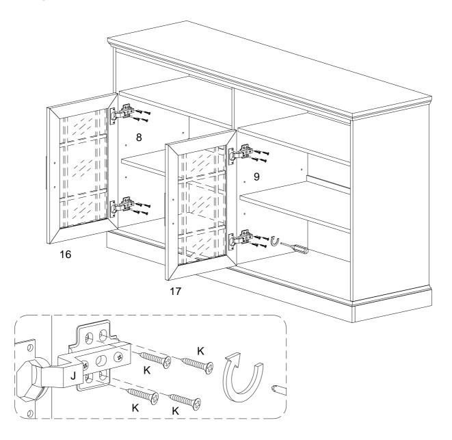
Using screw (K) secure west hinge (J) into part (8,9,16,17) with Philips head screwdriver as per diagram.
