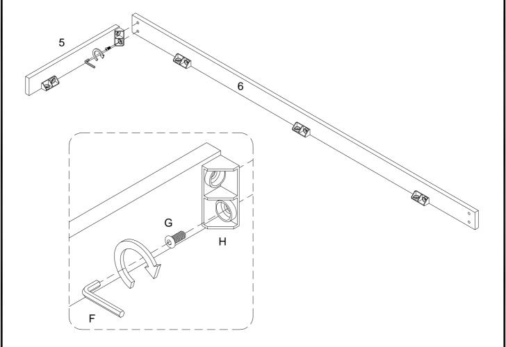
Using bolt (G) secure plastic wedge (H) to parts (5,6) with hex key (F) as per diagram.
