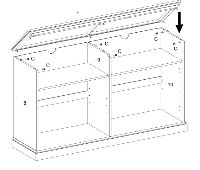
Put part (1) cover to parts (8,9,10) and using cam lock (C) secure with Philips head screwdriver as per diagram.
