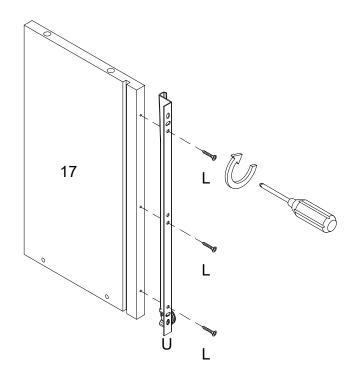
Using screw (L) attach part (S) to part (16), part (U) to part (17) with Philips head screwdriver as per diagram.
