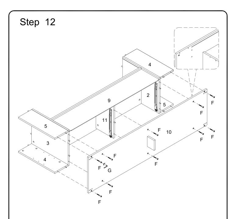
Using bolt (F) attach part (10) to parts (2,3,4,5,11) with hex key (G) as per diagram.
