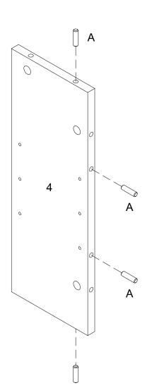
Insert wooden dowel (A) into parts (4,5) as per diagram.
