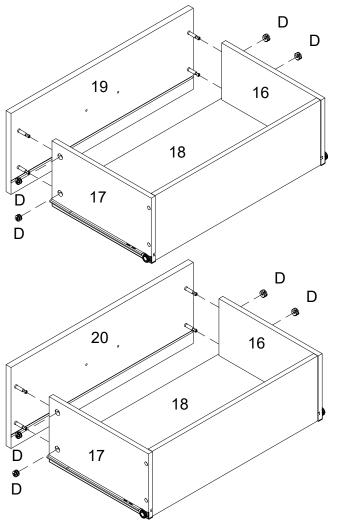
Using cam lock(D) secure parts (19,20) to parts (16,17) with Philips head screwdriver as per diagram.
