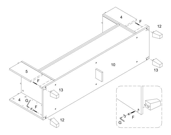
Using bolt (F) attach part (10) to parts (12,13) with hex key (G) as per diagram.
