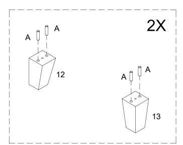
Insert wooden dowel (A) into parts (11,12,13) as per diagram.
