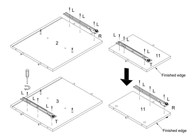
Using screw (L) attach part (R) to parts (2,11), part (T) to parts (3,11) with Philips head screwdriver as per diagram.
