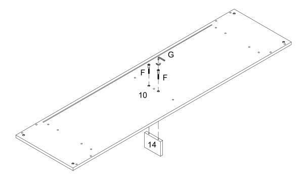
Using screw (F) attach part (10) into part (14) with hex key (G) as per diagram.
