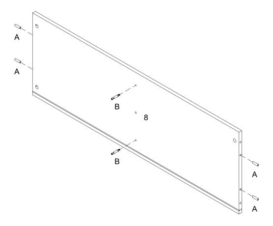
Insert wooden dowel (A) into part (8), then secure cam bolt (B) into part (8) with Philips head screwdriver as per diagram.
