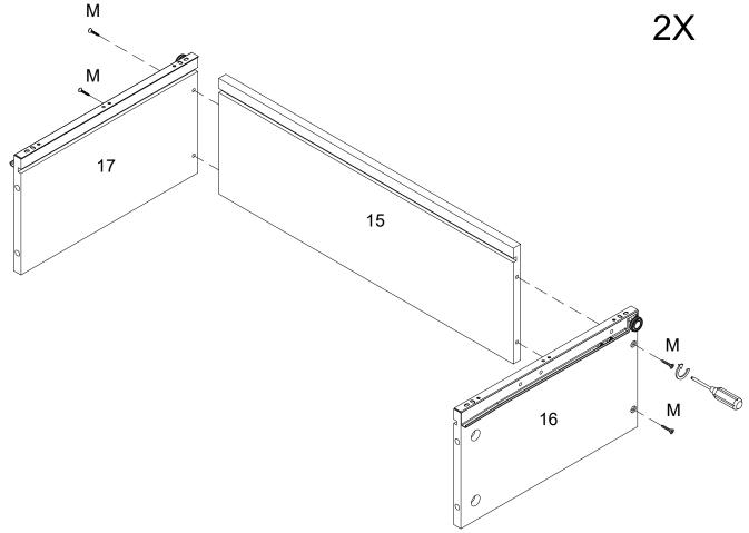
Using screw (M) attach parts (16,17) to part (15) with Philips head screwdriver as per diagram.
