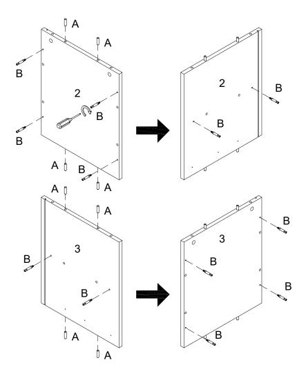
Insert wooden dowel (A) into parts (2,3) ,then secure cam bolt (B) into parts (2,3) with Philips head screwdriver as per diagram.
