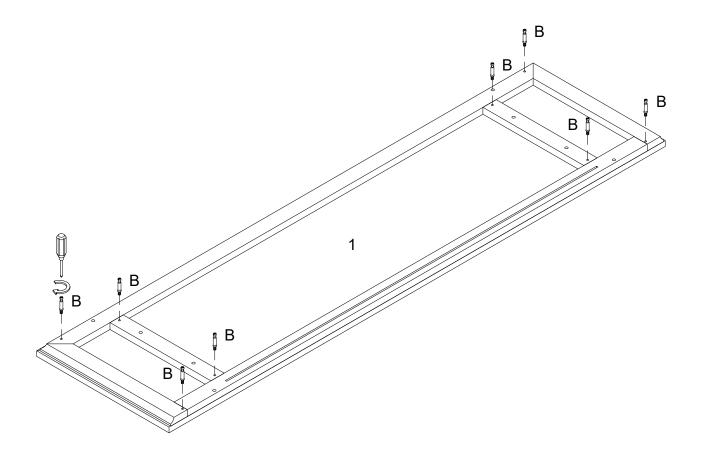
Secure cam bolt (B) into part (1) with Philips head screwdriver as per diagram.
