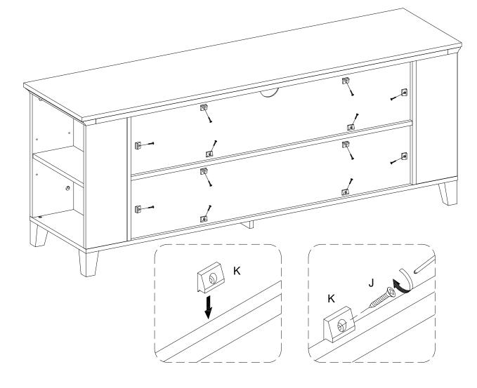
Using screw (J) secure plastic wedge (K) with Philips head screwdriver as per diagram.
