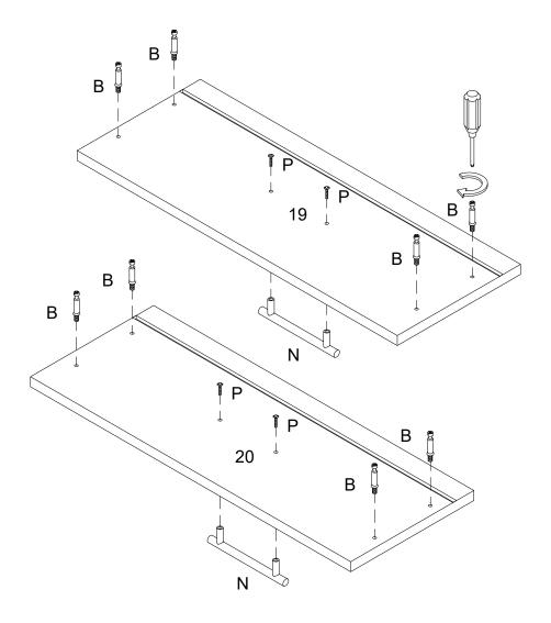
Secure cam bolt (B) into parts (19,20), then using handle bolt (P) secure handle (N) to parts (19,20) with Philips head screwdriver as per diagram.
