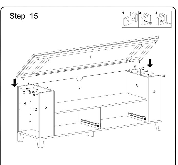
Using cam lock(C) secure part (1) to parts (2,3,4,5) with Philips head screwdriver as per diagram.
