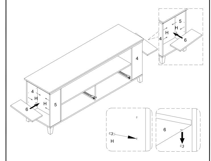
Insert shelf support pin (H) into parts (4,5) as per diagram. Make sure you place the four shelf support pins (H) in the same level. So the shelf is not titled .Put part (6) into unit as per diagram. Tilt and rest the adjustable shelf (6) onto the shelf support pins .
