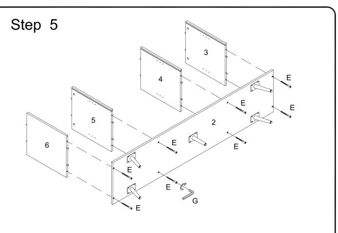
Attach part (3,4,5,6) to part (2) using bolt (E) with hex key (G)
