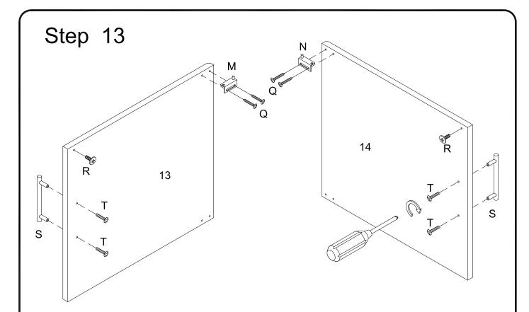
Attach handle (S) to part (13,14) using handle bolt (T) with screwdriver. Attach door hinge (M,N) to part (13,14) using screw (Q) with screwdriver. Attach bolt (R) to part (13,14) with screwdriver.
