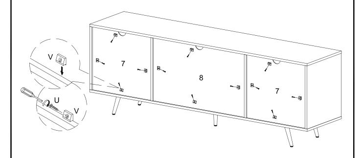
Attach plastic wedge (V) to part (7,8) using screw (U) with screwdriver.
