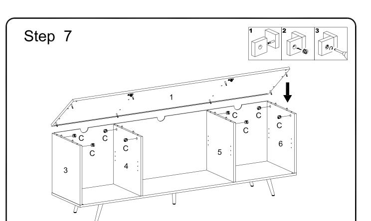
Attach part (1) to part (3,4,5,6), then insert and secure cam lock (C) to part (3,4,5,6) to lock it
