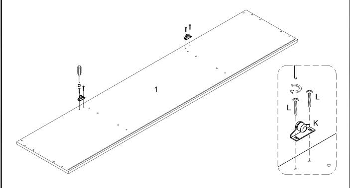
Attach door stopper (K) to part (1) using screw (L) with screwdrivers.
