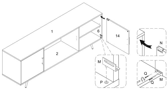
Insert top door hinge(N) into plastic pivot (P) on part (1), then slide the door (14) into the bottom hinge (M). Secure door by tightening door hinge (M) using screws (Q) with equal pressure.
