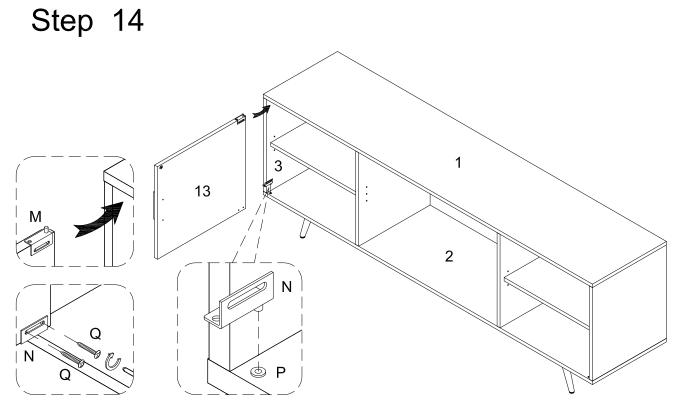
Insert top door hinge (M) into plastic pivot (P) on part (1), then slide the door (13) into bottom hinge (N). Secure door by tightening door hinge (N) using screws (Q) with equal pressure.
