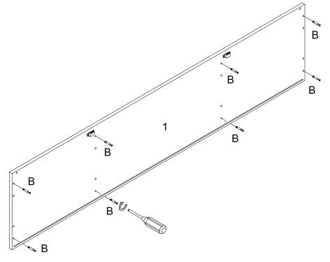
Attach cam bolt (B) to part (1) with screwdriver.
