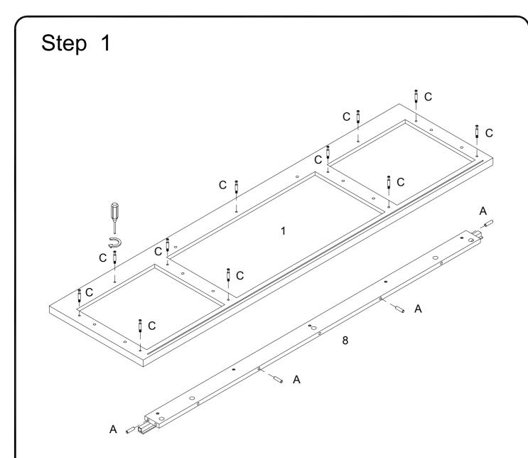
Insert wooden dowel (A) to part (8) ,using cam bolt (C) secure part (1) with Philips head screwdriver as per diagram.
