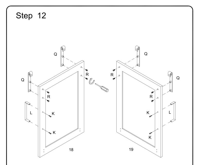
Using bolt (K) secure handle (L) into parts (18,19),and using bolt (R) secure pulley (Q) to parts (18,19) with Philips head screwdriver as per diagram.
