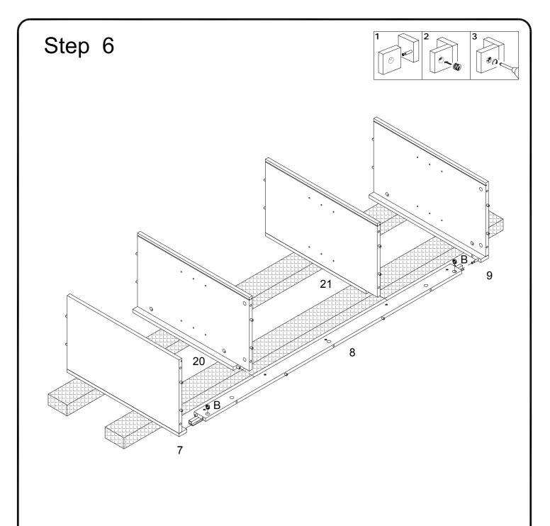
Using cam lock (B) secure part (8) to parts (7,9,20,21) with Philips head screwdriver as per diagram.
