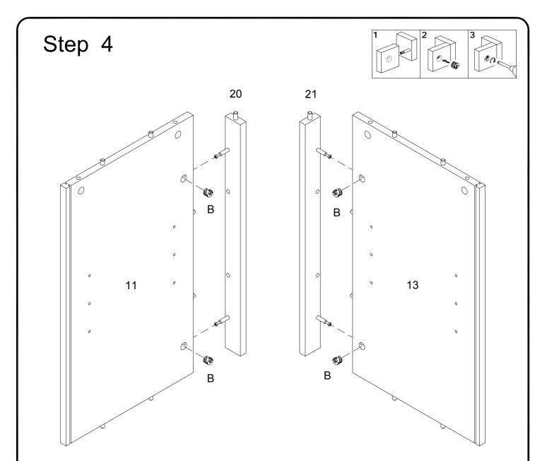
Using cam lock (B) secure parts (11,13) to parts (20,21) with Philips head screwdriver as per diagram.
