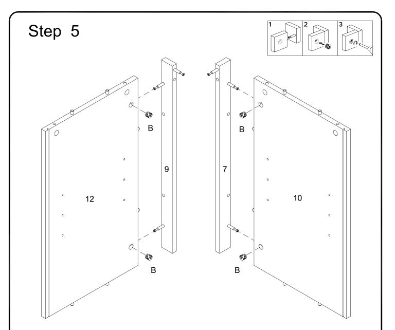
Using cam lock (B) secure parts (7,9) to parts (10,12) with Philips head screwdriver as per diagram.
