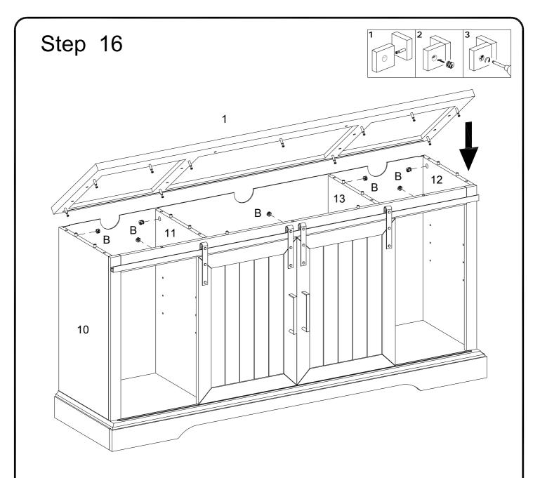
Using cam lock (B) secure part (1) into parts (10,11,12,13) with Philips head screwdriver as per diagram.
