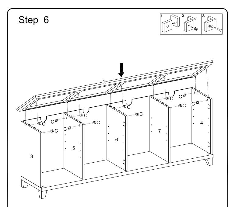
Using cam lock (C) insert part (3,4,5,6,7) to part (1) on the top secure with Philips head screwdriver as per diagram.
