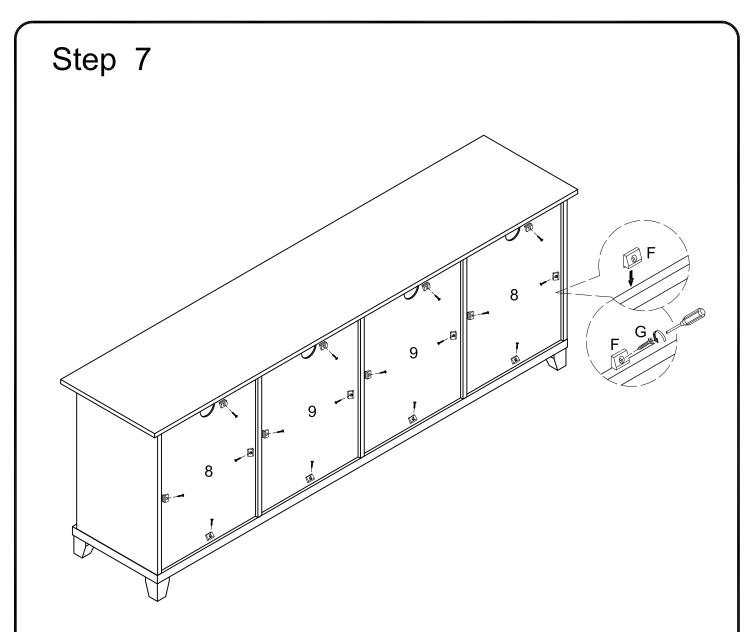
Using screw (G) insert plastic wedge to parts (8,9) with Philips head screwdriver as per diagram.
