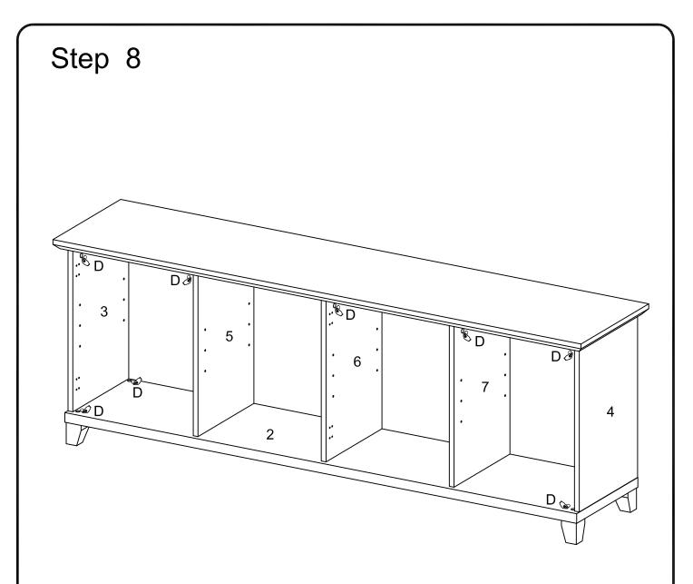
Place sticker (D) cover the hole on parts (2,3,4,5,6,7) as per diagram.
