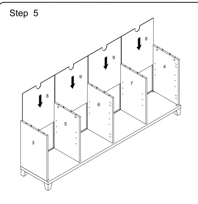
Put parts (8,9) to parts (3,4,5,6,7) as per diagram.
