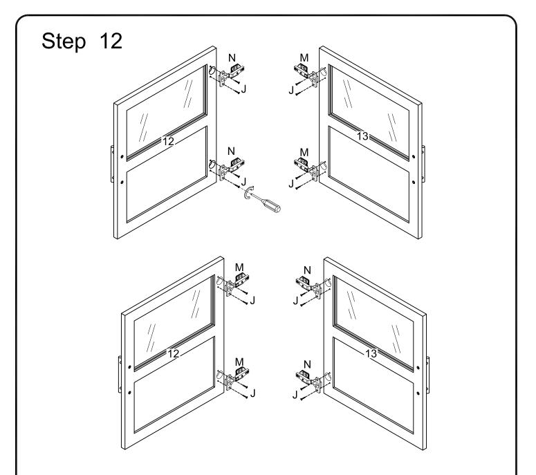
Using bolt (J) secure hinge (M,N) to parts (12,13) with Philips head screwdriver as per dia gram.
