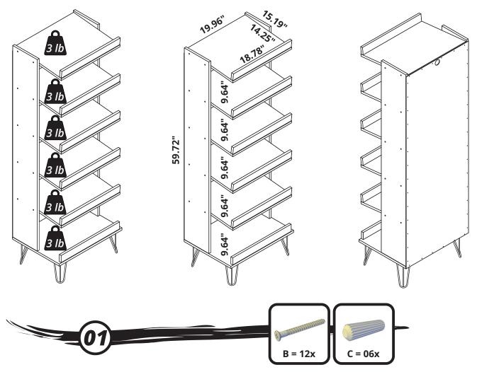
Connect the part (03) onto the parts (01, 02) with the hardware (B + C).
