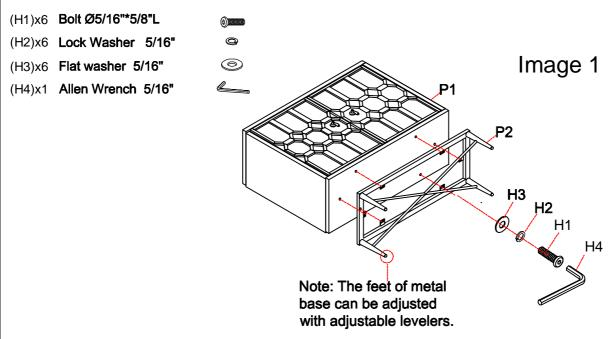
Step 2. Securely tighten all bolts, then turn the assembled cabinet to an upright position. Assembly is complete. Failure to follow these instructions may cause the bolts to misalign during assembly.
