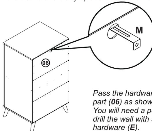
Pass the hardware (M) through the hole of the part (06) as shown in the figure.
