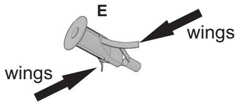
*\*Press the hardware (E) to put in the hole that you drilled in the wall.*
