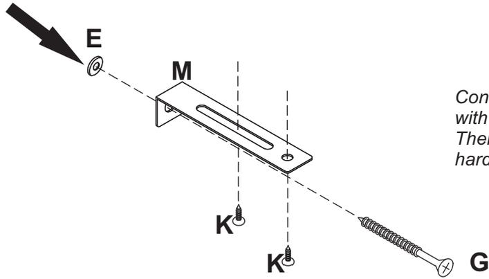
*Connect the hardware (M) onto the wall with the hardware (G).
