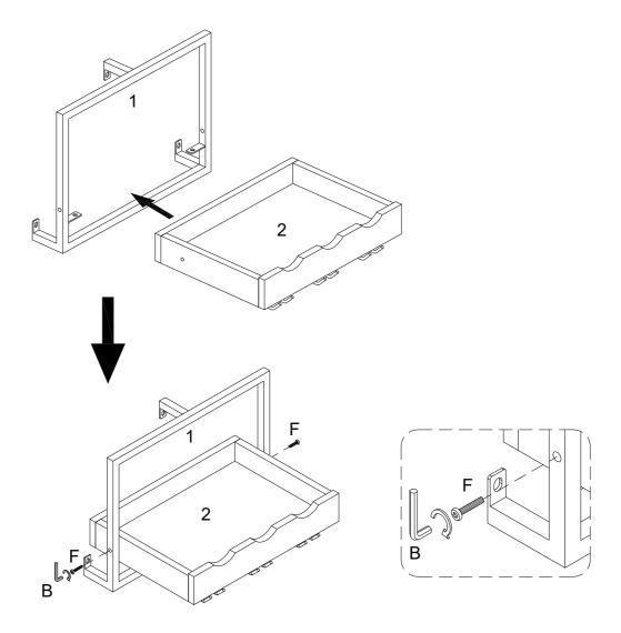
Using Bolt (F) attach part (1) to part (2) with Hex Key (B) as per diagram.
