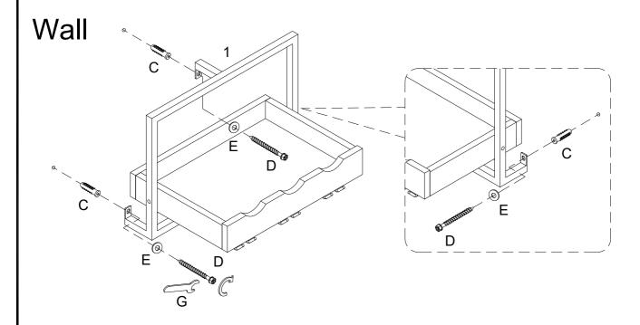
Using Screw (D) attach Flat Washer (E) into part (1) and Anchor (C) to Wall with Wrench (G) as per diagram.
