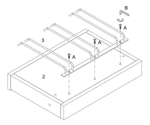
Using Bolt (A) part (3) to part (2) with Hex key (B) as per diagram.
