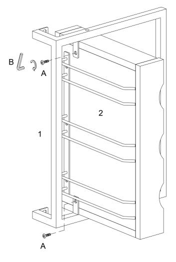
Using Bolt (A) attach part (1) to part (2) with Hex Key (B) as per diagram.
