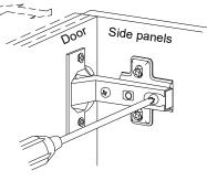
In-and-Out by loosening the hinge-arm mounting screw or via cam adjustment
