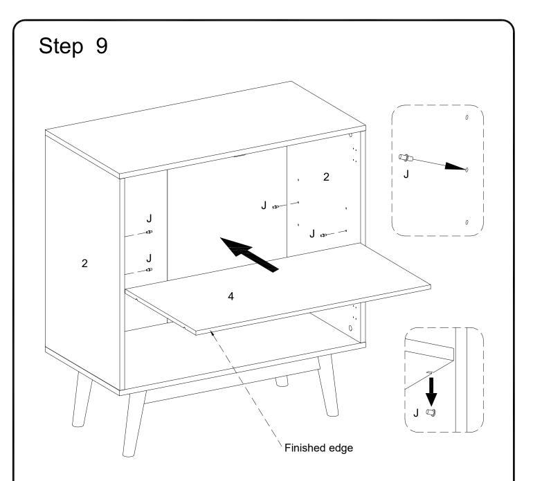
Insert shelf support pin (J) into part (2) as per diagram. Make sure you place the four shelf support pins (J) in the same level. So the shelf is not titled .Put part (4) into unit as per diagram. Tilt and rest the adjustable shelf(4) onto the shelf support pins .
