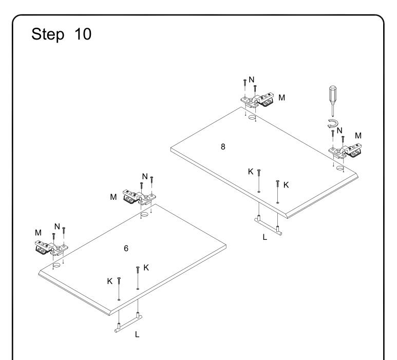
Using screw (N) attach Europe hinge (M) to parts (6,8) , then using handle bolt (K) secure handle (L) to parts (6,8) with Philips head screwdriver as per diagram.
