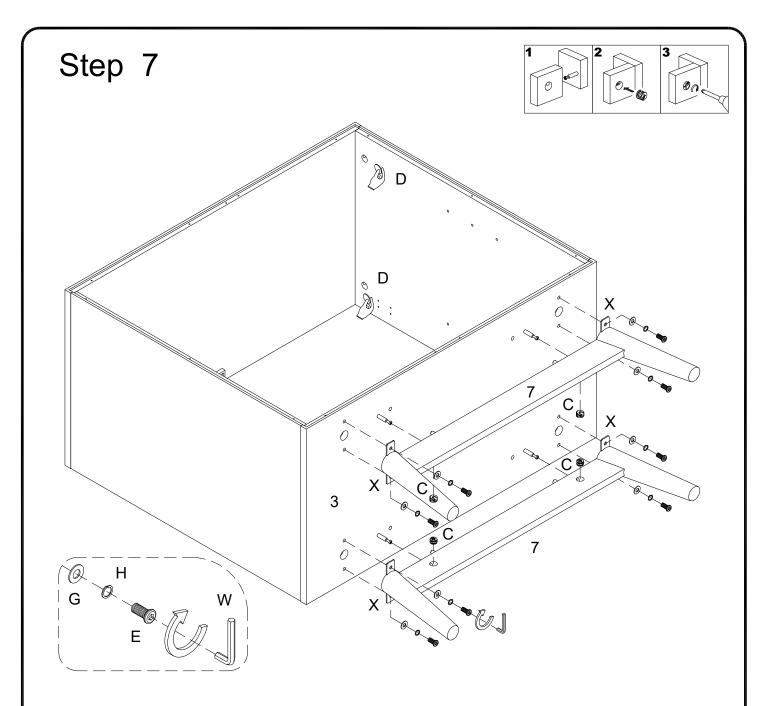
Using cam lock(C) secure part (7) to part (3) with Philips head screwdriver .and using bolt (E) with lock washer (H),flat washer (G) secure plate (X) to part (3) with hex key (W) as per diagram. Place sticker (D) cover the holes as per diagram finally.
