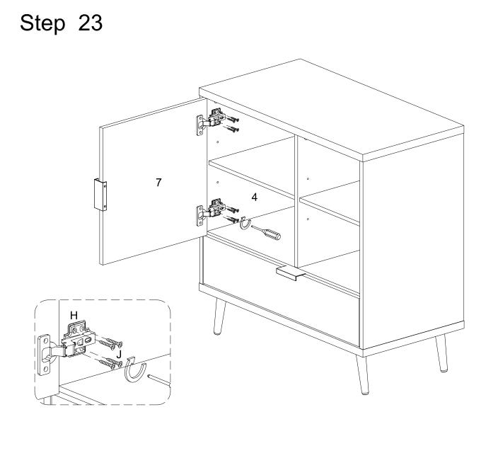
using screw (J) attach Europe hinge(H) to part (4) with Philips head screwdriver as per diagram.
