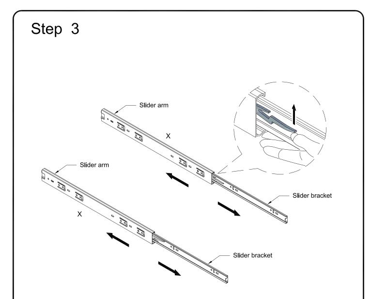
Pick up the slider arm (X) and separate the slide Runner for the following steps. Extend the Slide .Runner all the way forward, press the plastic release lever of the slider arm up and pull the Slide Runner Complete out .
