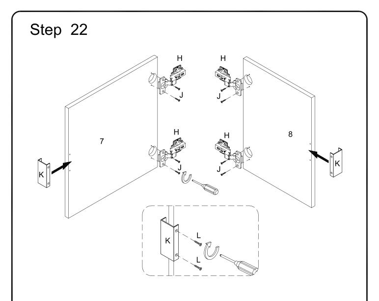
Using screw (L) attach handle (K) to parts (7,8) ,and using screw (J) attach Europe hinge(H) to parts(7,8) with Philips head screwdriver as per diagram.
