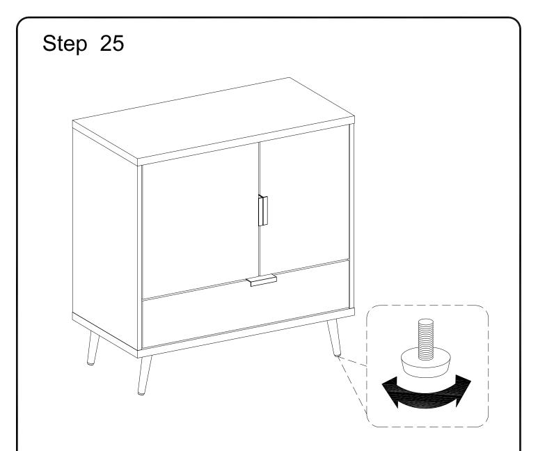
Position the assembled unit at the desired location ,if necessary adjust the floor leveler at the bottom of the legs to level the unit .
