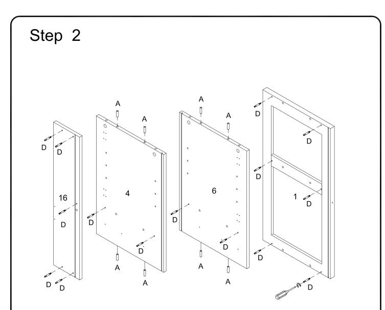
Insert wooden dowel (A) into parts (4,6), secure cam bolt (D) into parts (1,16) with Philips head screwdrivers per diagram.
