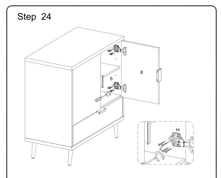
using screw (J) attach Europe hinge(H) to part (6) with Philips head screwdriver as per diagram. Open and close the doors ,if necessary adjust the screws for a good fit.
