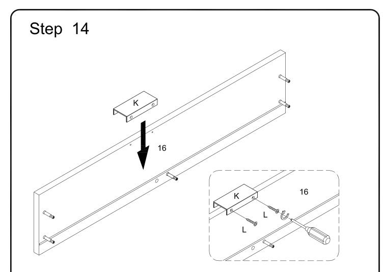
Using screw (L) attach handle (K) to part (16) with Philips head screwdriver as per diagram.
