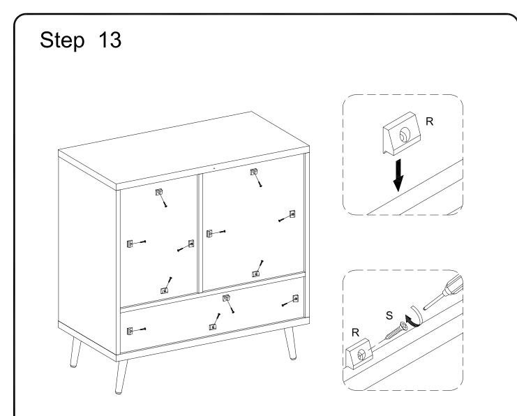
Using screw (S) secure plastic wedge (R) with Philips head screwdriver as per diagram.
