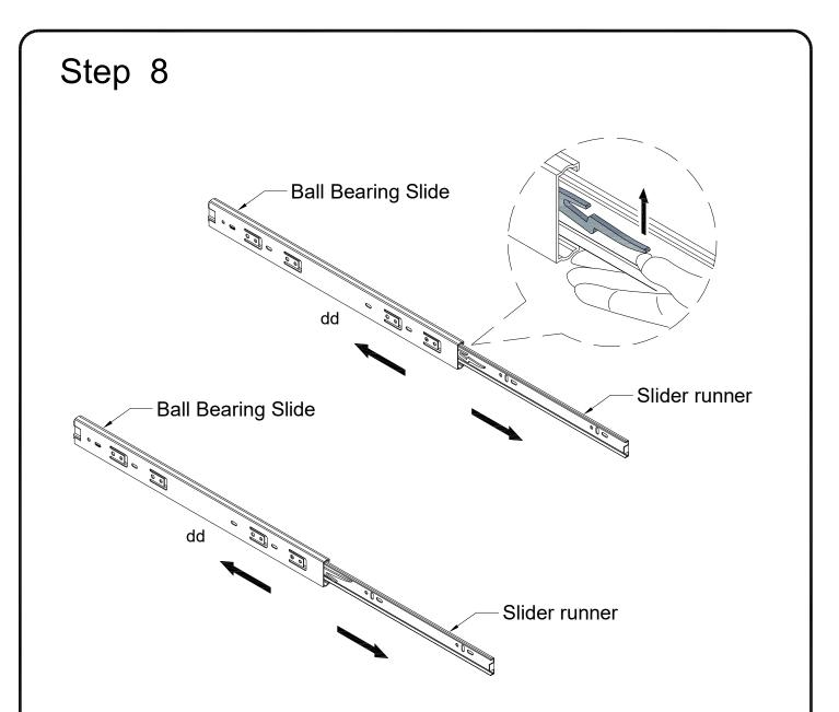
Pick up the Ball Bearing Slides (dd) and separate the slide Runner for the following Steps. Extend the Slide Runner all the way forward, press the plastic release lever of the ball bearing Slides up and pull the Slide Runner Complete out .
