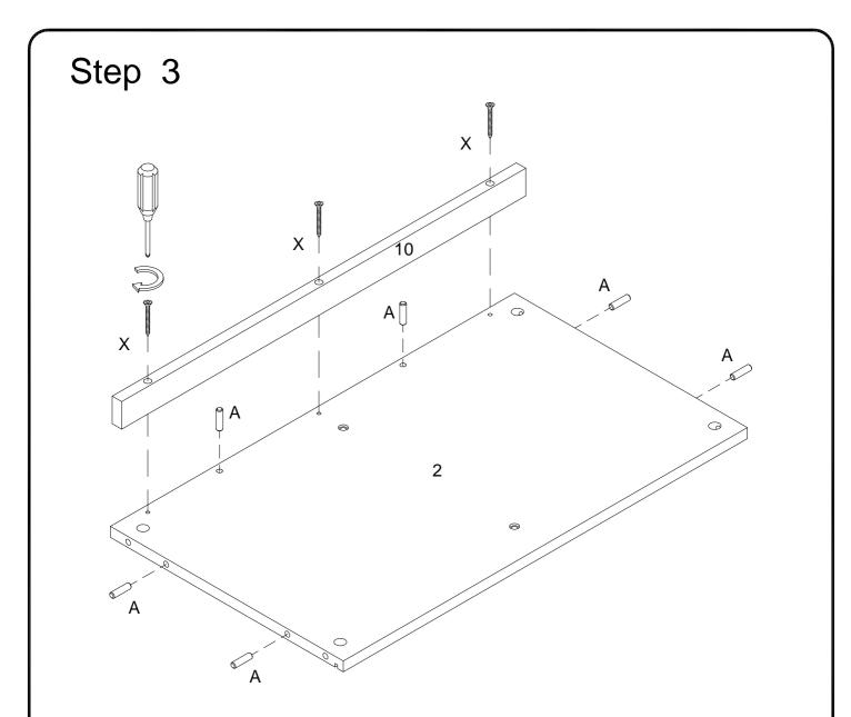
Insert wooden dowel (A) into part (2) ,then using screw (X) secure part (10) into part (2) with Philips head screwdriver as per diagram.
