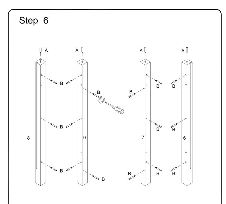
Insert wooden dowel (A) into parts (6,7,8,9) ,then using cam bolt (B) secure parts (6,7,8,9) with Philips head screwdriver as per diagram.
