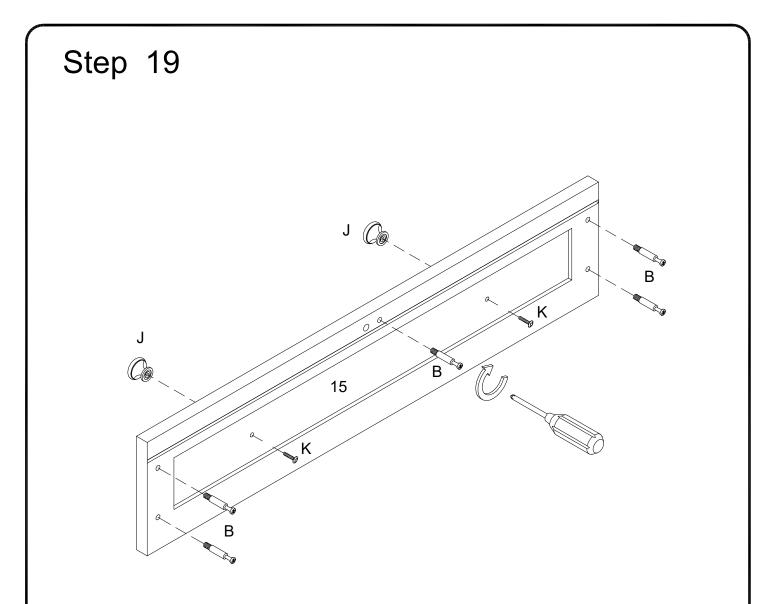
Using cam bolt (B) secure part (15) ,then using handle bolt (K) secure handle (J) into part (15) with Philips head screwdriver as per diagram.
