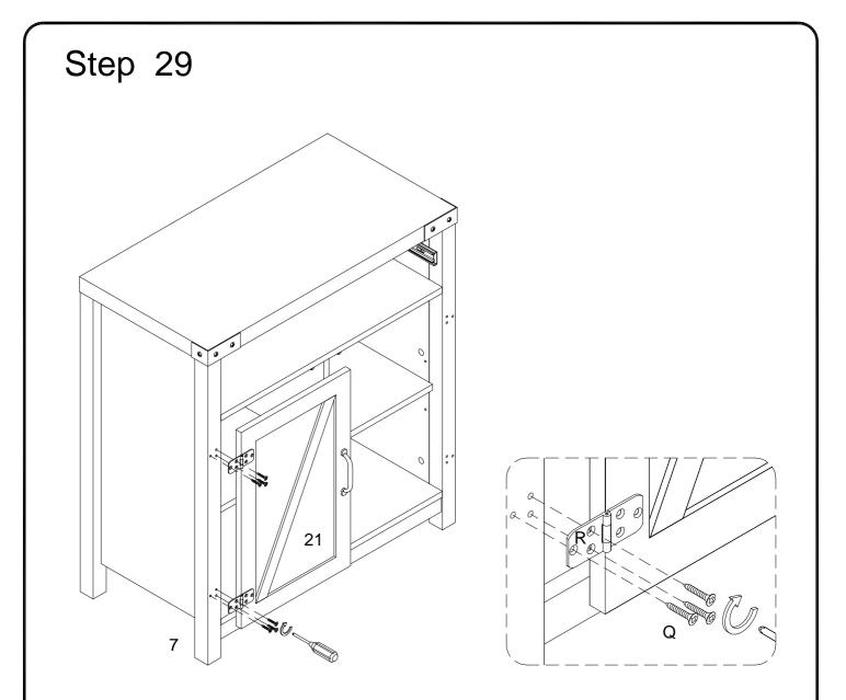
Using screw (Q) secure hinge (R) into part (7) with Philips head screwdriver as per diagram.
