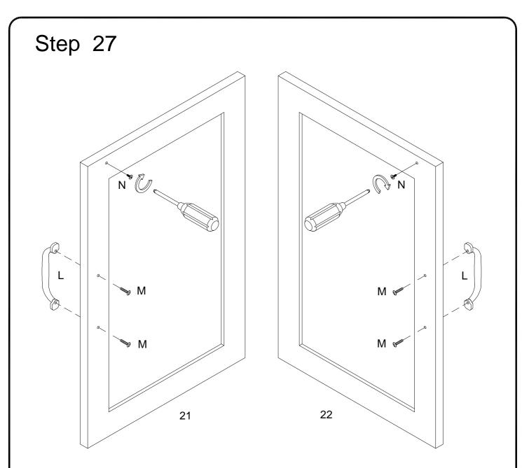
Using bolt (N) secure part(21,22), then using handle bolt (M) secure part(21,22) into handle (L) with Philips head screwdriver as per diagram.
