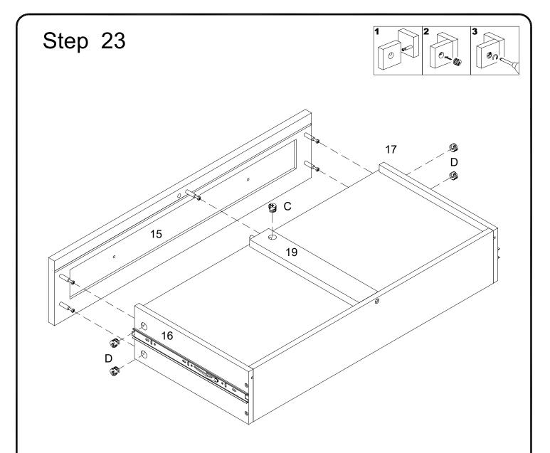
Using cam lock (C) secure part (15) into part (19), then using cam lock (D) secure part (15) into parts (16,17) with Philips head screwdriver as per diagram.
