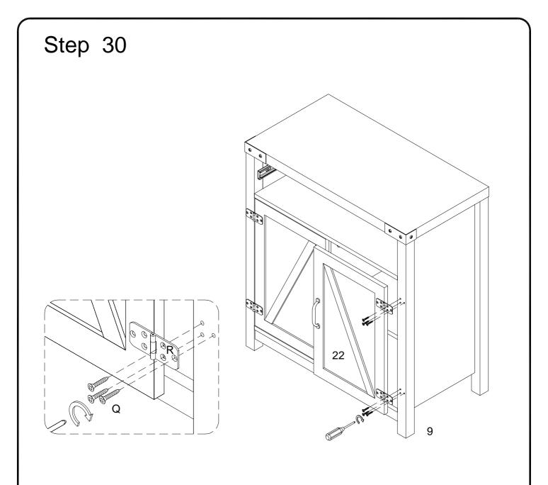
Using screw (Q) secure hinge (R) into parts (9) with Philips head screwdriver as per diagram.
