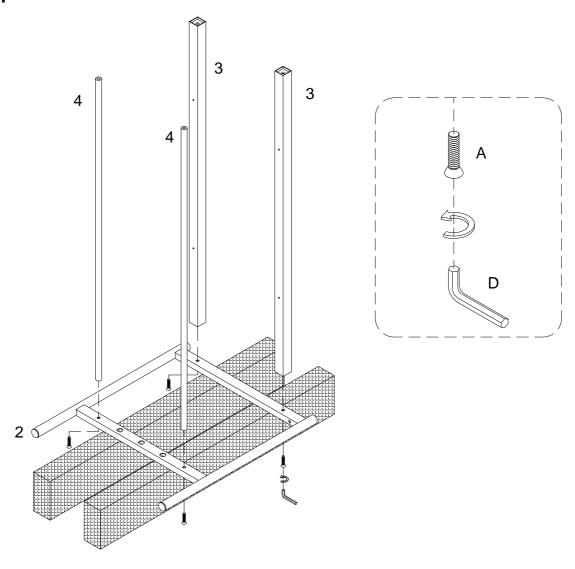
Using bolt (A) attach part (2) to parts (3,4) with Hex key (D) as per diagram. Note: Do not fully tighten all bolts.
