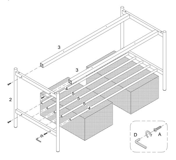
Insert part (5) to part (2),then using bolt (A) attach part (2) to parts (3,4) with Hex key (D) as per diagram.
