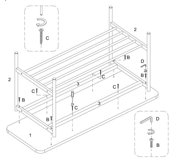
Using bolt (B) attach part (2) to part (1) with Hex key (D) ,then using screw (C) secure part (3) to part (1) with Philips head screwdriver as per diagram.
