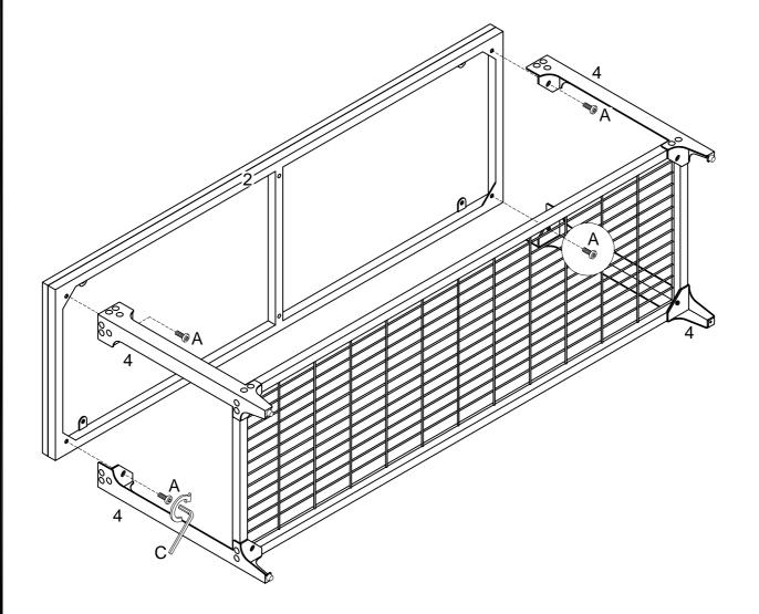
Using bolt (A) secure part (4) into part (2) with hex key (C) as per diagram. Then fully tighten all the bolts.
