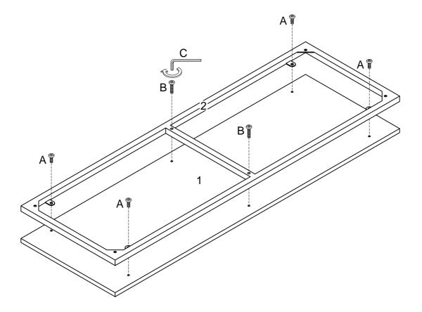
Using bolts (A,B) secure part (2) into part (1) with hex key (C)as per diagram.
