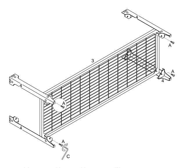
Using bolt (A) secure part (4) into part (3) with hex key (C)as per diagram.
