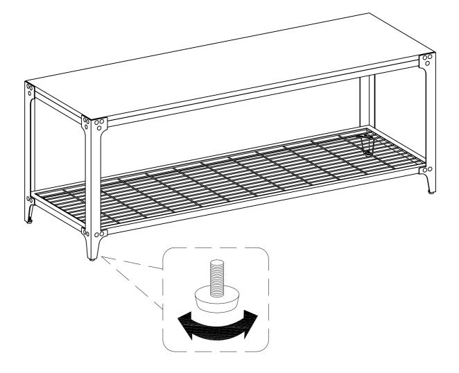
Position the assembled unit at the desired location .If necessary, adjust the floor levelers at the bottom of the legs (4) to the level the unit .
