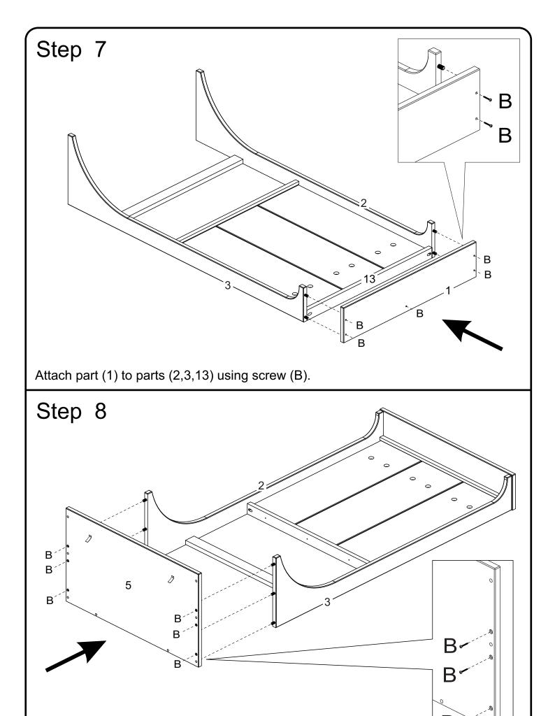
Attach part (5) to parts (2,3) using screw (B).
