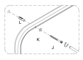
Using screw (J) attach Flat washer (K) into part (1) to nut (L) to wall with Philips head screwdriver as per diagram.
