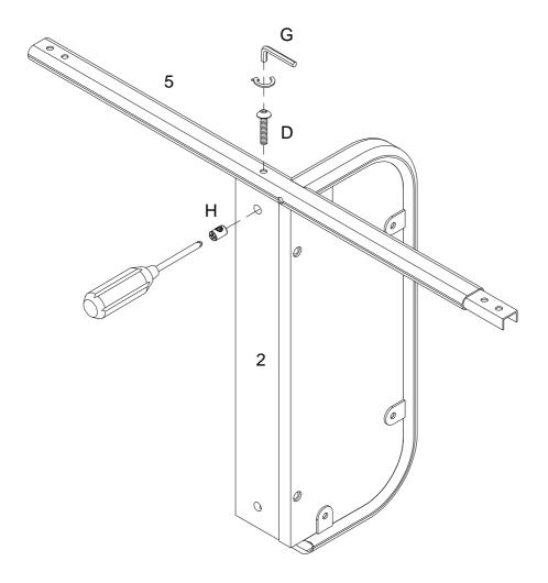
Secure Nut (H) into part (2) with Philips head screwdriver, then using bolt (D) attach part (5) to part (2) with Hex key (G) as per diagram.
