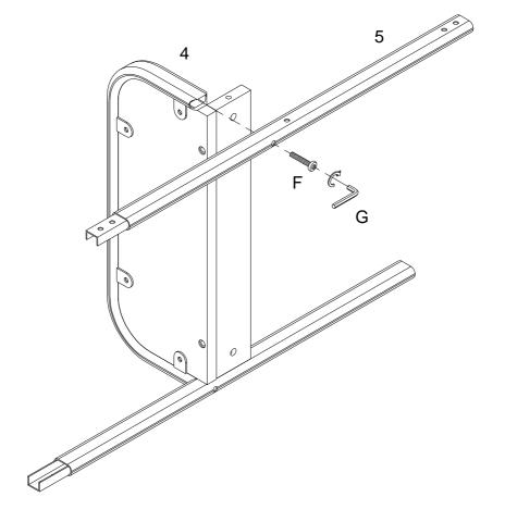
using Bolt (F) attach part (5) to part (4) with Hex key (G) as per diagram.
