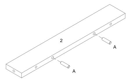
Insert wooden dowel (A) into part (2) as per diagram.
