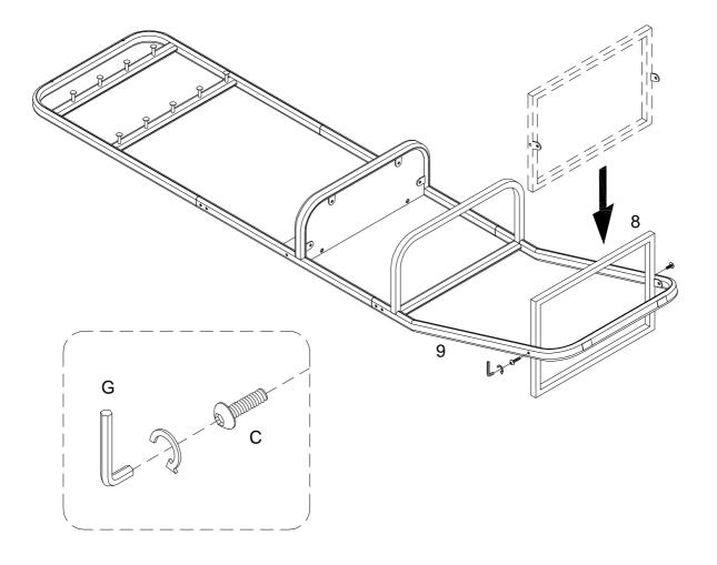
Using bolt (C) attach part (9) to part (8) with Hex key (G) as per diagram. Note: Do not fully tighten bolts .
