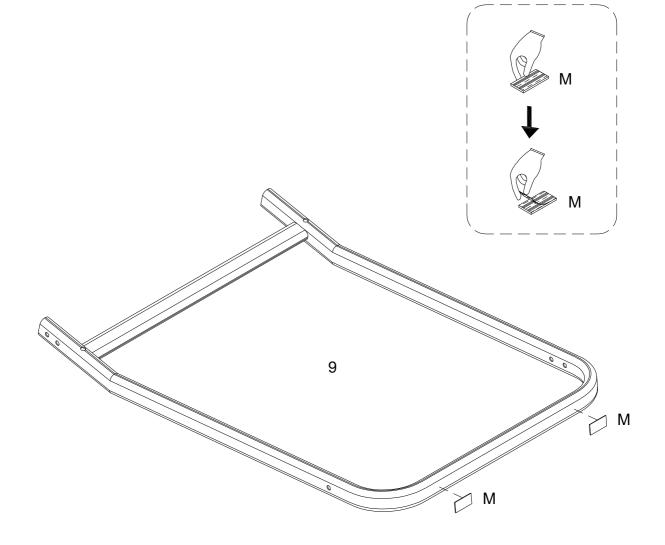
Tear off the EVA pad (M) and place the pad on part (9) as per diagram.
