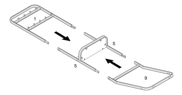
Attach parts(1,9) to part (5) as per diagram.
