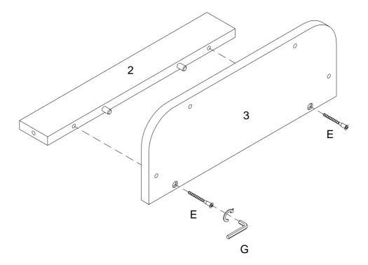
Using screw (E) attach part (3) into part (2) with Hex key (G) as per diagram.
