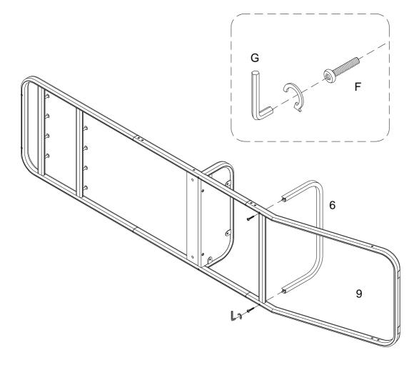
Using bolt (F) attach part (9) to part (6) with Hex key (G) as per diagram.
