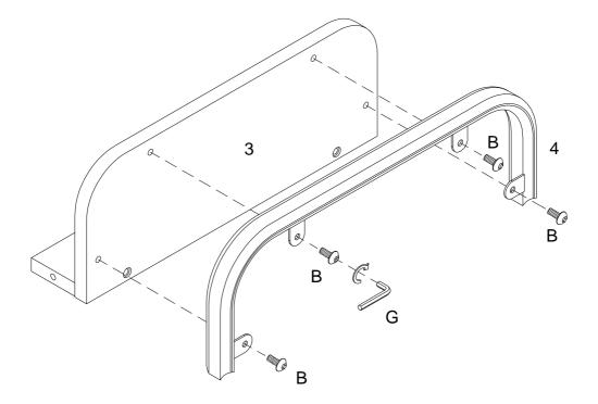
Using Bolt (B) attach part (4) to part (3) with Hex key (G) as per diagram.
