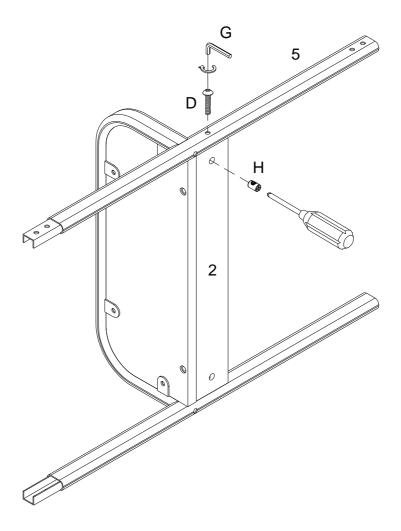
Secure Nut (H) into part (2) with Philips head screwdriver , then using bolt (D) attach part (5) to part (2) with Hex key (G) as per diagram.
