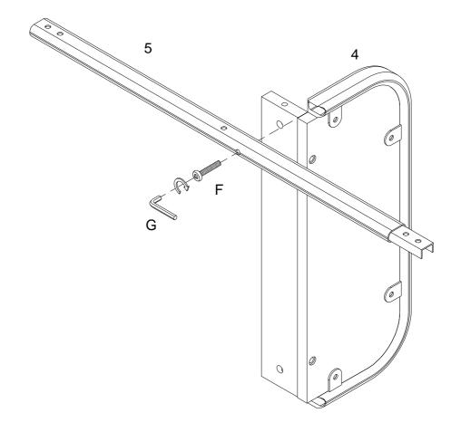
Using Bolt (F) attach part (5) to part (4) with Hex key (G) as per diagram. Note: Please do not fully tighten all bolts .
