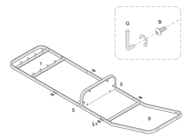
Using bolt (B) attach parts (1,9) to part (5) with Hex key (G) as per diagram.
