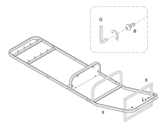
Using bolt (B) attach part (8) to part (9) with Hex key (G) as per diagram. Note: Fully tighten all bolts.
