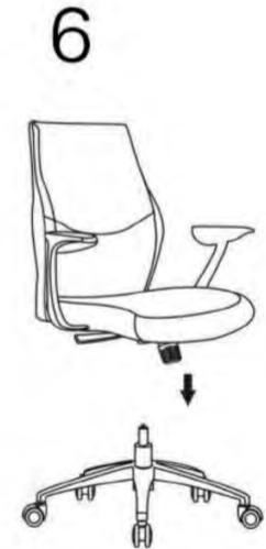
During assembly, hand tighten screws only. When the screws are in place, tighten completely.
