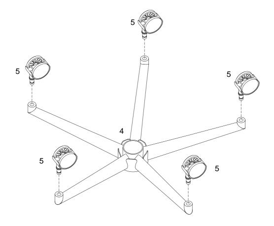
Place parts (5) to the bottom of part (4) as per diagram.
