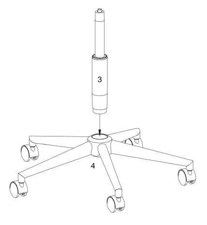
Insert part (3) into part (4) as per diagram.
