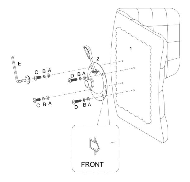
Using bolts (C,D) insert Lock washer (B) ,Flat Washer (A) into part (2) to part (1) with Hex Key (E) as per diagram.
