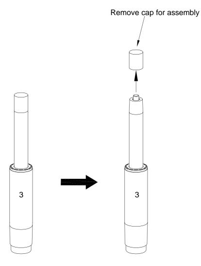
Remove cap at the top of part (3) as per diagram.
