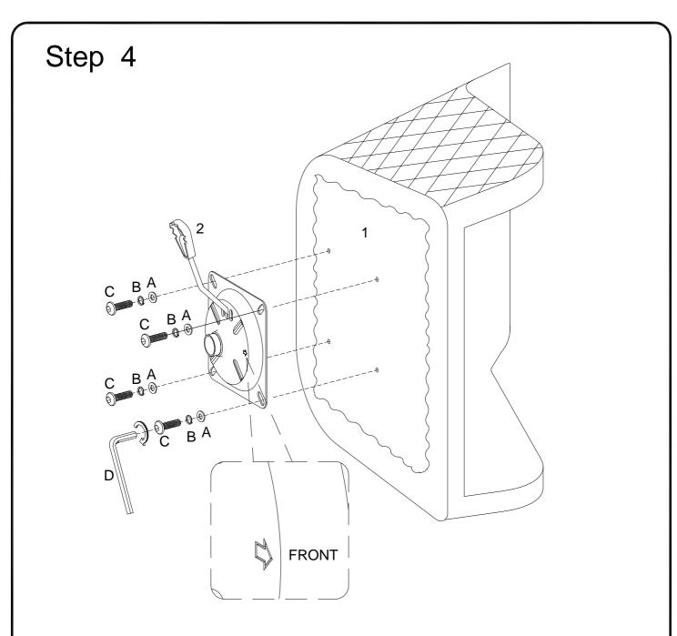
Using bolt (C) insert Lock washer (B) ,Flat Washer (A) into part (2) to part (1) with Hex Key (D) as per diagram.
