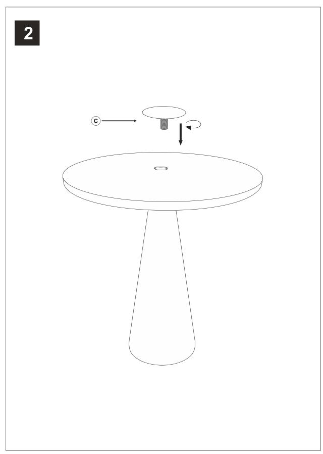
Attach the top to the base using the screw ( c ) and rotating it clockwise
