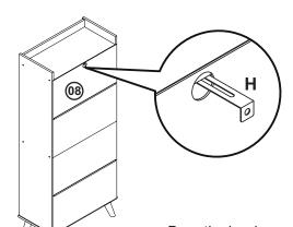
Pass the hardware (**H**) through the hole of the part (**08**) as shown in the figure.
