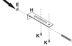
Connect the hardware (**H**) onto the wall with hardware (**B**). Then fasten with the hardware (**K**) the hardware (**H**) on the part (**01**).
