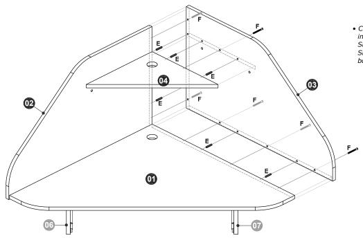
• Connect the Right Side Panel (03) into the Top Panel (01), the Left Side Panel (02) and the Upper Shelf (04) with dowels (E) and bolts (F).
