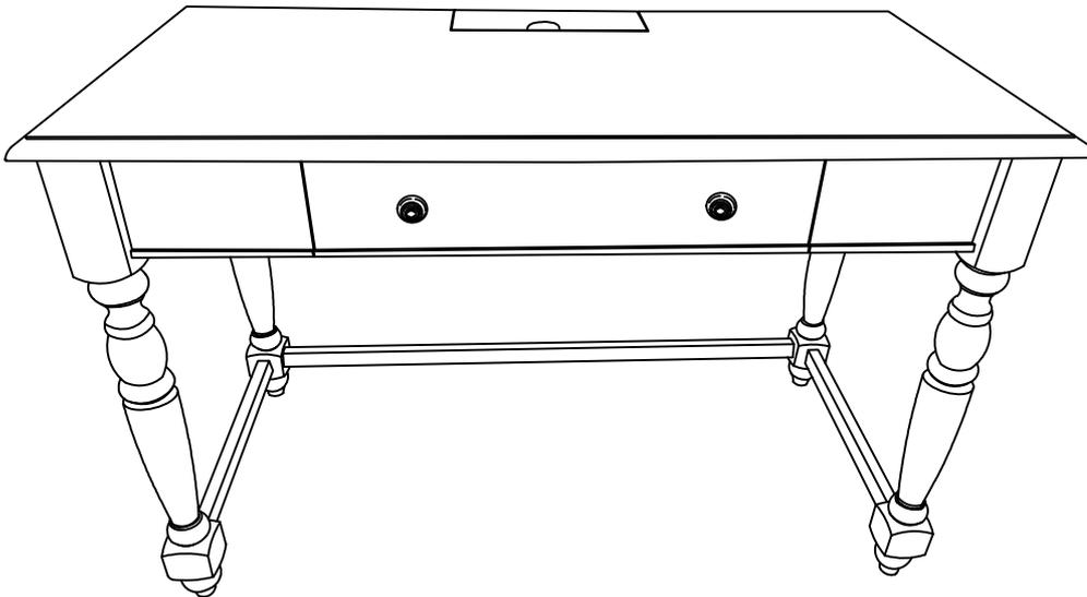
Stand Table up on an even surface and check that it is balanced. If there is a slight wobble, apply downward pressure in the corner where a leg is uneven. Keeping pressure in that corner, tighten all bolts. If balanced, apply downward pressure evenly in the center and tighten all bolts. Do not over-tighten beyond hole depth.
