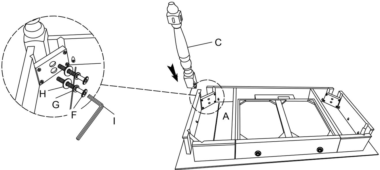
Take the Allen Key, and turn the bolts until the legs are secured.
