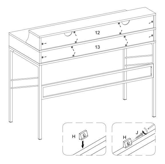
Using screw (J) secure plastic wedge (H) to parts (12,13) with Philips head screwdriver as per diagram.
