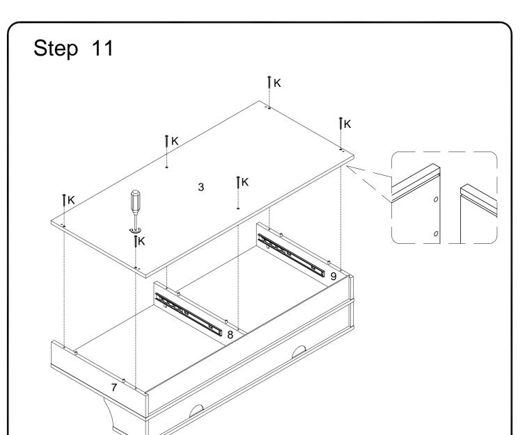
Using screw (K) attach part (3) to parts (7,8,9) with Philips head screwdriver as per diagram.
