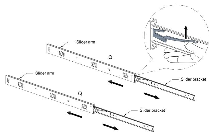
Pick up the slider arm (Q) and separate the slide runner for the following Steps. Extend the slide runner all the way forward,press the plastic release lever of the slider arm up and pull the slide runner complete out .
