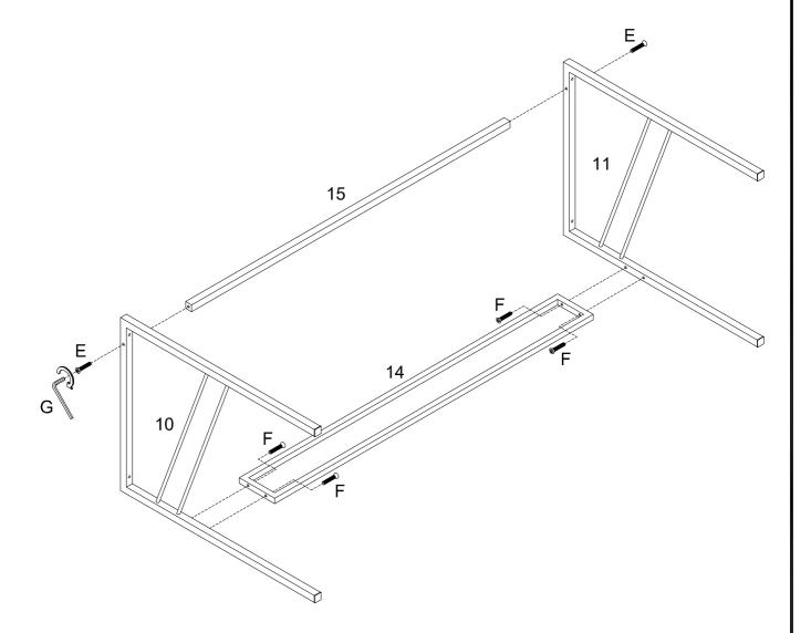
Using Bolt (E) attach parts (10,11) into part (15), then using bolt (F) attach part (14) to parts (10,11) with Hex key (G) as per diagram.
