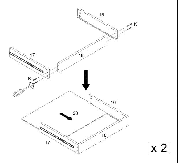
Using screw (K) attach parts (16,17) to part (18) with Philips head screwdriver ,then insert part (20) as per diagram.
