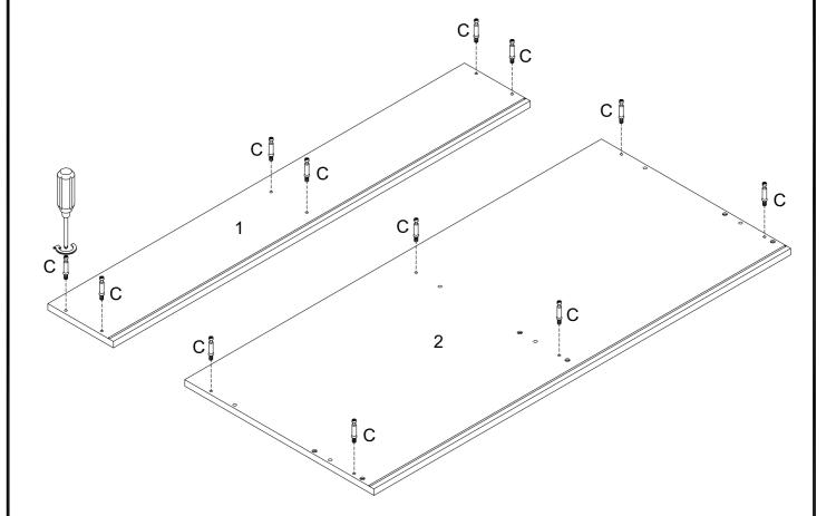
Secure cam bolt (C) into parts (1,2) with Philips head screwdriver as per diagram.
