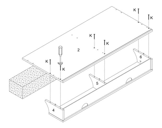
Using screw (K) attach part (2) to parts (4,5,6) with Philips head screwdriver as per diagram.
