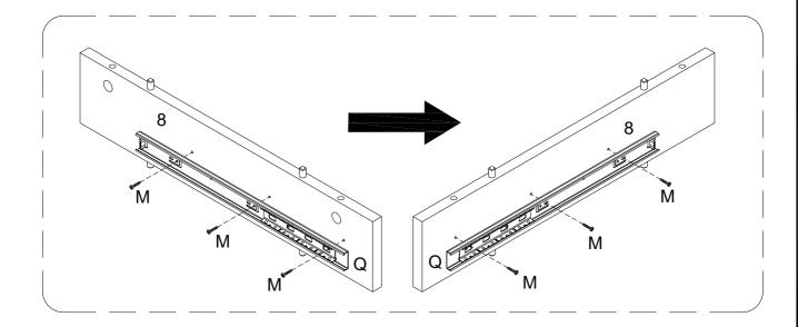
Using screw (M) attach drawer slider (Q) to parts (7,8,9) with Philips head screwdriver as per diagram.
