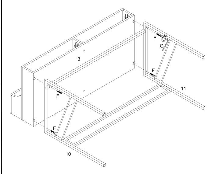
Using Bolt (F) attach parts (10,11) into part (3) with Hex key (G) as per diagram.
