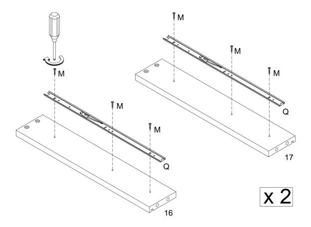
Using screw (M) attach drawer slider (Q) to parts (16,17) with Philips head screwdriver as per diagram.
