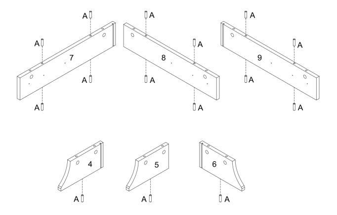
Insert wooden dowel (A) into parts (4,5,6,7,8,9) as per diagram.
