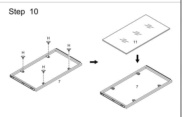
Insert rubber suction cups (H) into keyboard tray frame (7) .Carefully lay keyboard tray glass (11) in place
