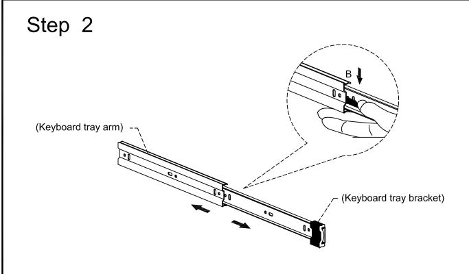
Disassemble keyboard tray slider (B) by sliding the tray arm and tray bracket apart. Depress the small lever of the tray bracket and carefully pull the two pieces apart. Repeat this process for both keyboard tray sliders (B).
