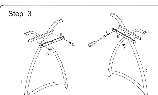
Attach the tray arms of keyboard tray sliders (B) to legs (1,2) using screws (C). Ensure that the open end of each tray arm is near the front of each leg. Tighten screws (C) with a screwdriver.
