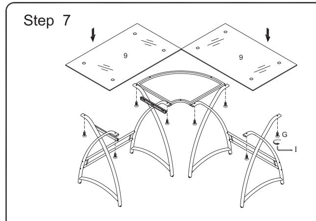
Attach glass (9) to the desk frame using medium bolts (G). Tighten medium bolts (G) with wrench (I).
