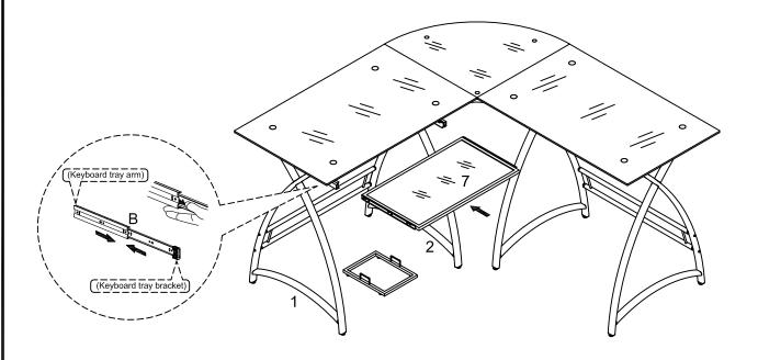
Carefully slide keyboard tray frame (7) into place. The tray brackets attached to keyboard tray frame (7) will slide into the tray arms attached to legs (1, 2).
