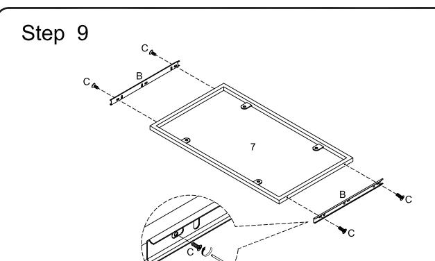
Attach the tray brackets of keyboard tray sliders (B) to keyboard tray frame (7) using screws (C). Ensure that the open end tray bracket is near the back of keyboard tray frame (7). Tighter screws (C) with a screwdriver.
