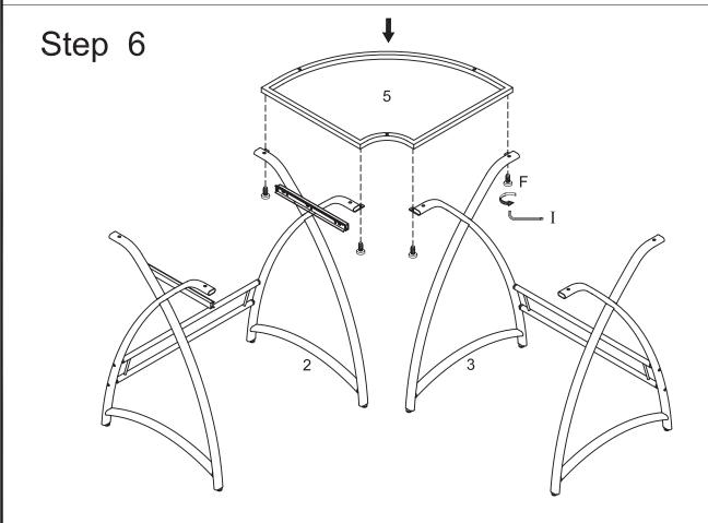
Attach corner frame (5) to legs (2,3) using short bolts (F). Tighten short bolts (F) with wrench (I).
