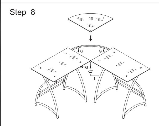
Attach middle glass (10) to the desk frame using medium bolts (G). Tighten medium bolts (G) with wrench (I).
