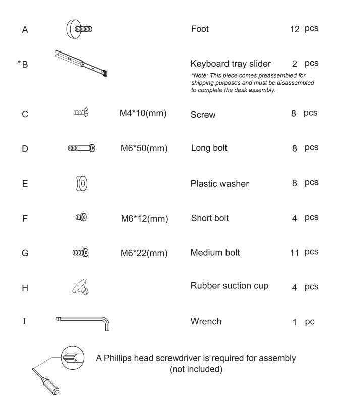
The hardware quantities listed above are required for proper assembly.
