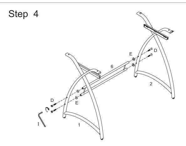
Attach crossbar (6) to legs (1,2) using long bolts (D) and plastic washers (E). Tighten long bolts (D) with wrench (I).
