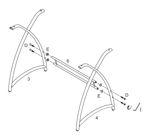
Attach crossbar (6) to legs (3,4) using long bolts (D) and plastic washers (E). Tighten long bolts (D) with wrench (I).
