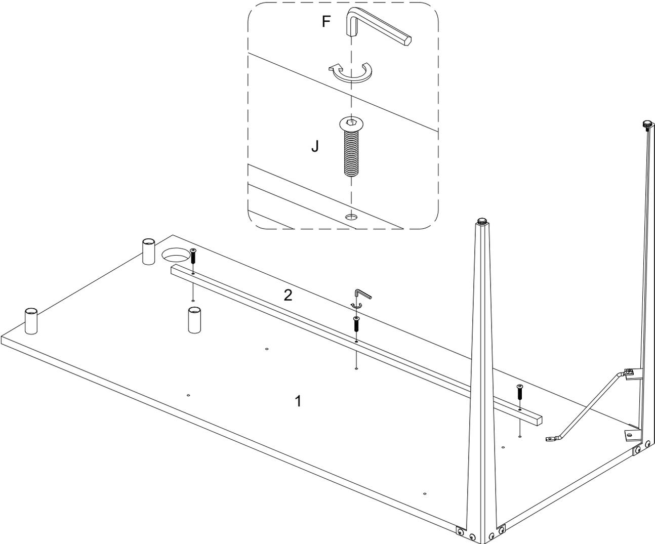
Using bolt (J) attach part (2) to part (1) with hex key (F) as per diagram.
