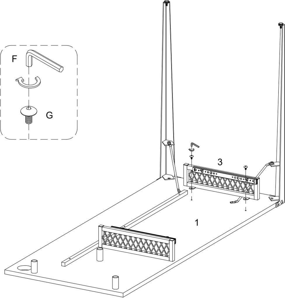
Using bolt (G) attach part (3) to part (1) with hex key (F) as per diagram.
