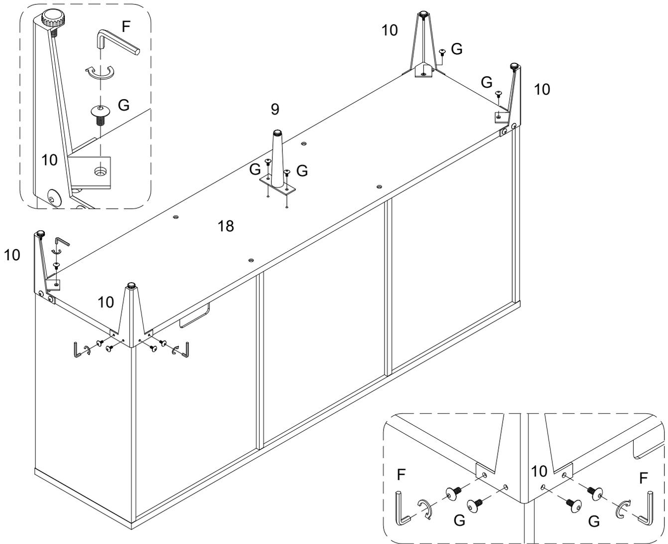
Using bolt (G) attach parts (9,10) to part (18) with hex key (F) as per diagram.
