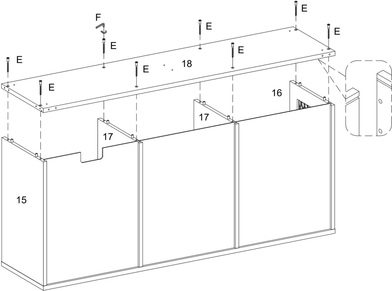
Using screw (E) attach part (18) into parts (15,16,17) with hex key (F) as per diagram.
