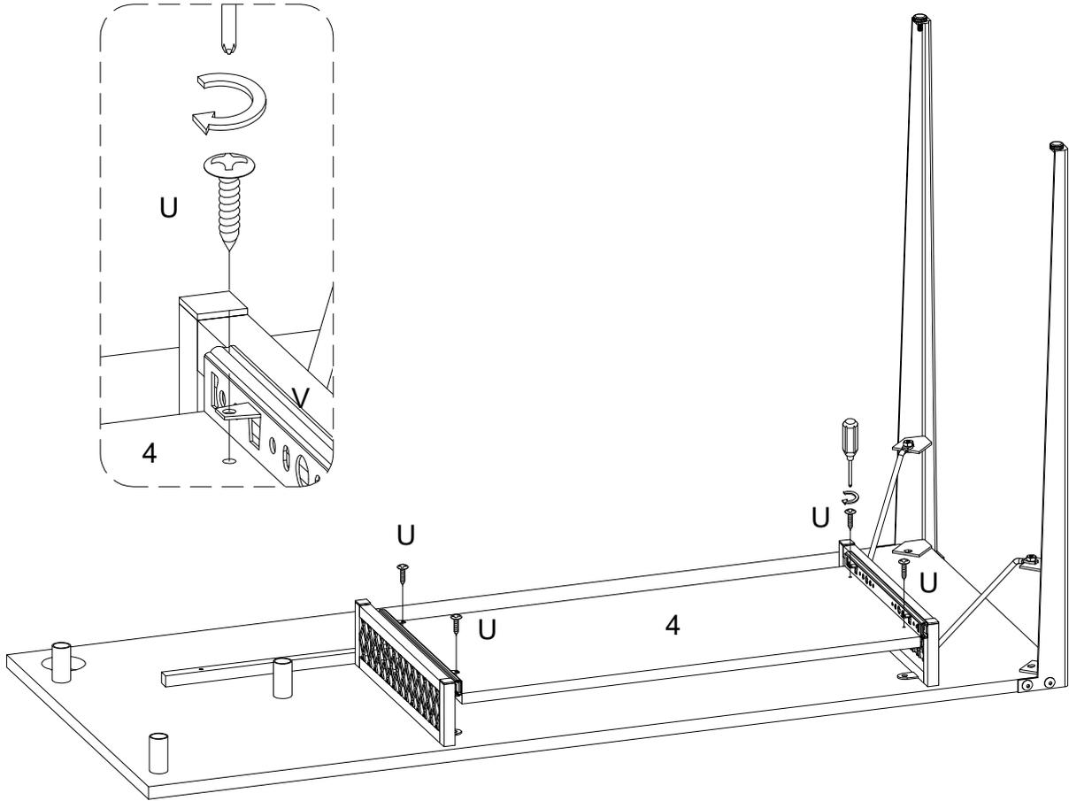
Using screw (U) attach slider drawer bracket (V) into part (4) with Philips head screwdriver as per diagram.
