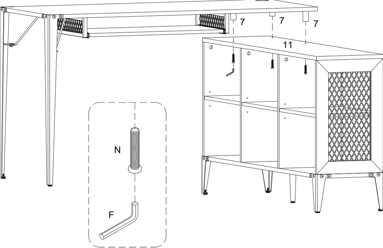
Using bolt (N) attach part (11) into part (7) with hex key (F) as per diagram.
