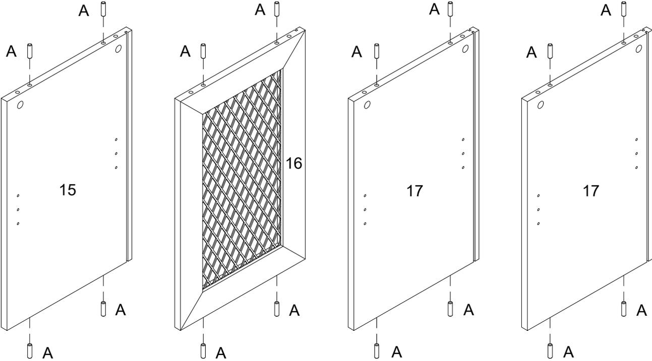
Insert wooden dowel (A) into parts (15,16,17) as per diagram.
