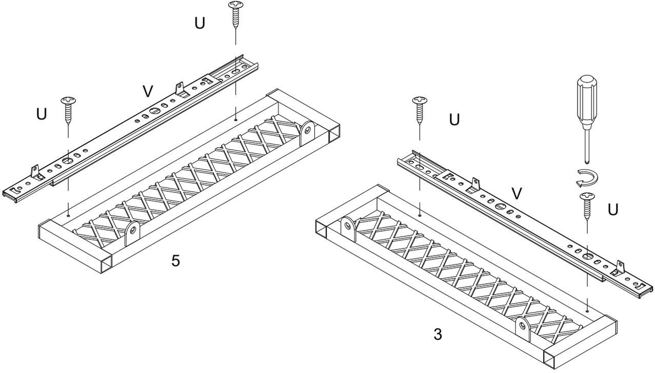
Using screw (U) attach drawer slider (V) to parts (3,5) with Philips head screwdriver as per diagram.
