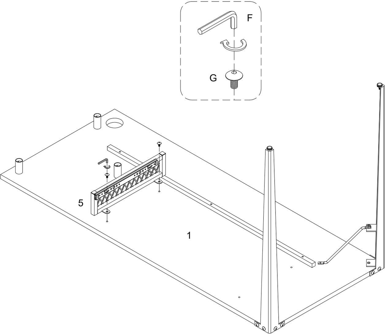
Using bolt (G) attach part (5) to part (1) with hex key (F) as per diagram.
