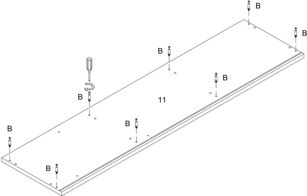
Secure cam bolt (B) into part (11) with Philips head screwdriver as per diagram.
