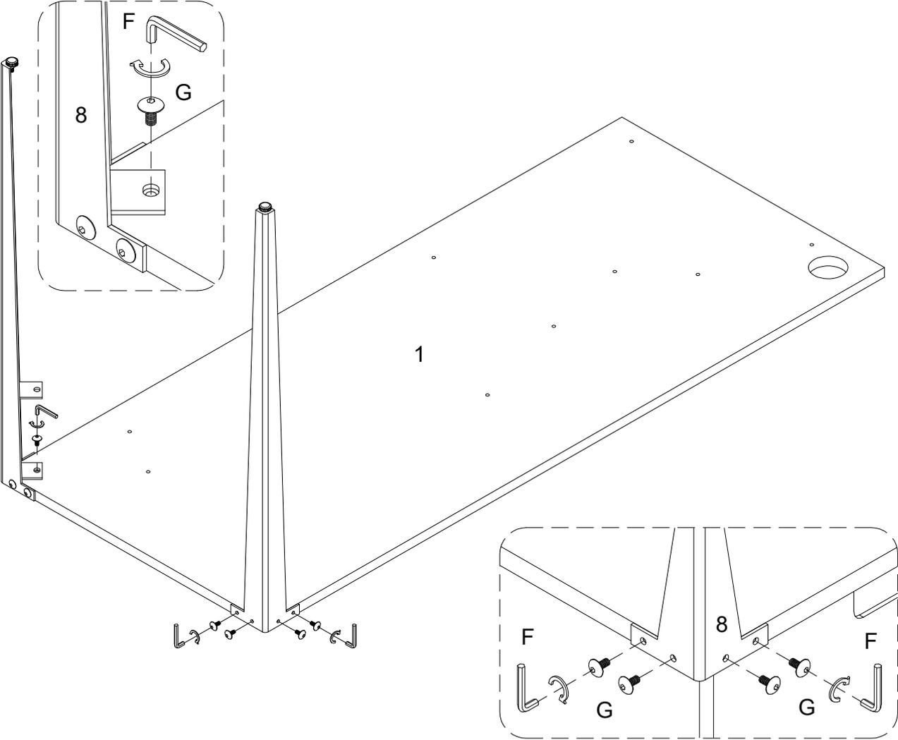
Using bolt (G) attach part (8) into part (1) with hex key (F) as per diagram.
