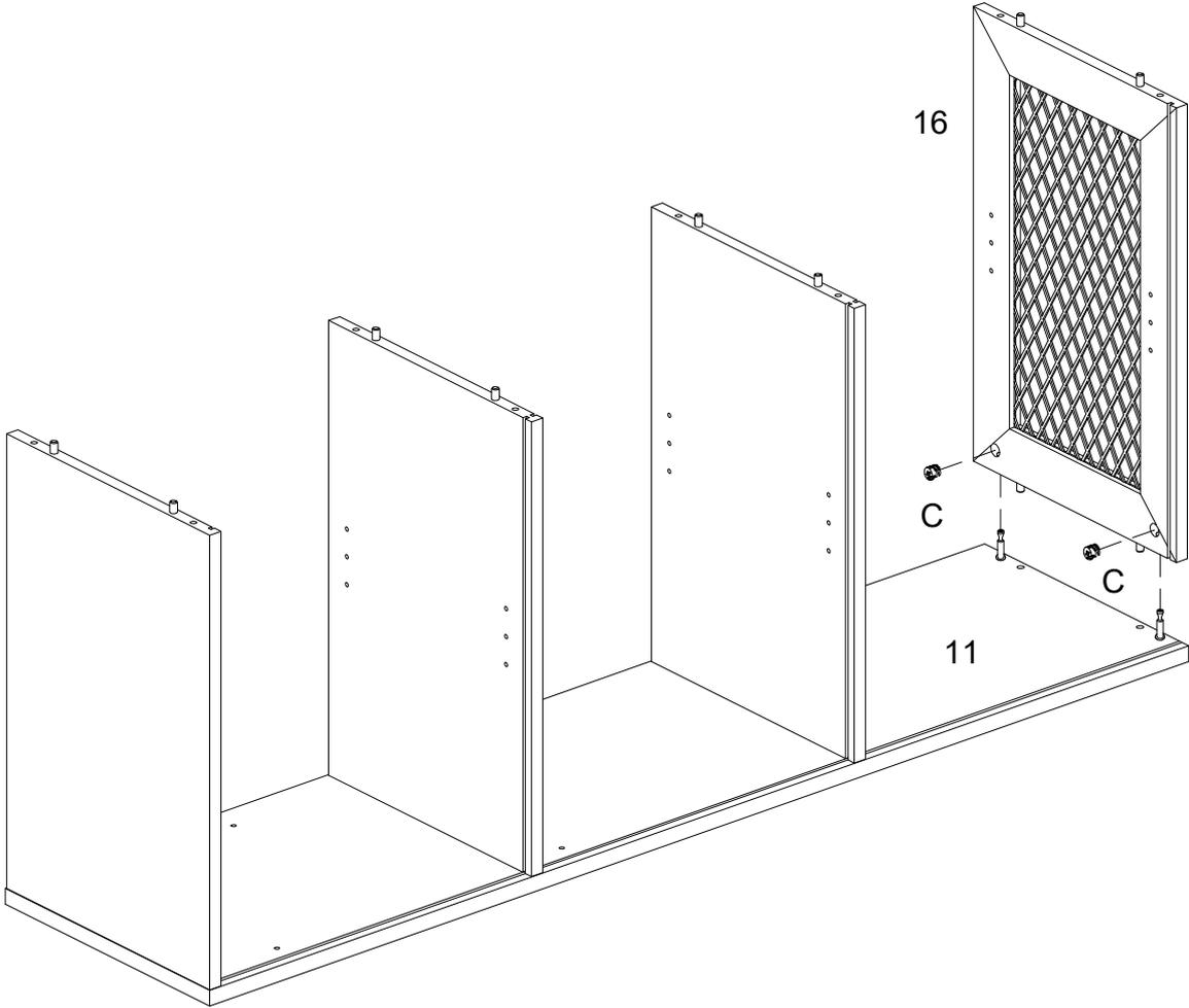
Using cam lock(C) secure part (16) to part (11) with Philips head screwdriver as per diagram.
