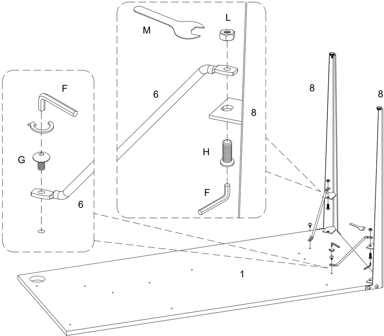
Using bolt (G) attach part (6) into part (1) with hex key (F) ,then using bolt (H) and Nut (L) attach part (8) into part (6) with wrench (M) and Hex Key (F) as per diagram.
