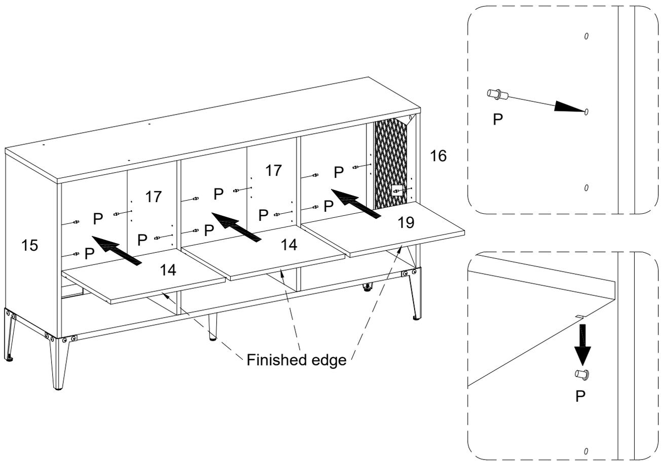
Insert shelf support pin (P) into parts (15,16,17) as per diagram. Make sure you place the four shelf support pins (P) in the same level. So the shelf is not titled .Put parts(14,19) into unit as per diagram Tilt and rest the adjustable shelf onto the shelf support pins .
