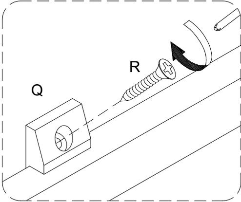
Using screw (R) secure plastic wedge (Q) with Philips head screwdriver as per diagram.
