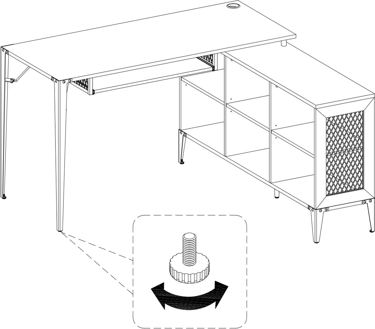
Position the assembled unit at the desired location ,if necessary adjust the floor leveler at the bottom of the support leg to level the unit .
