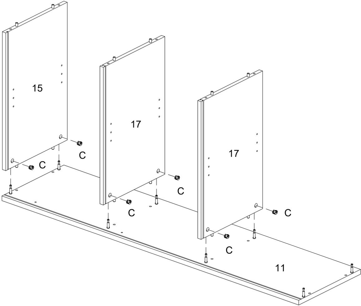
Using cam lock(C) secure parts (15,17) to part (11) with Philips head screwdriver as per diagram.
