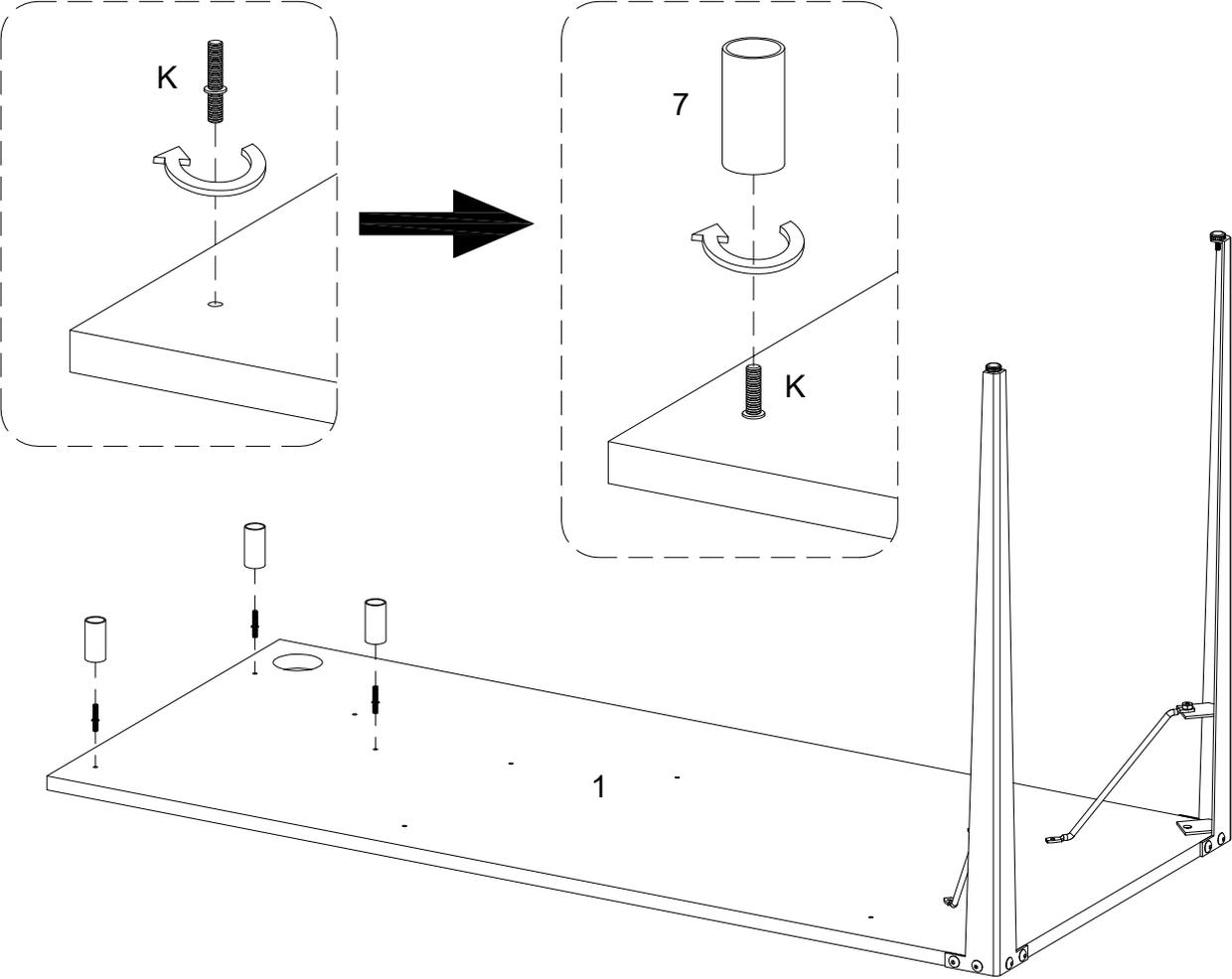
Insert bolt (K) into part (1), then secure part (7) as per diagram.
