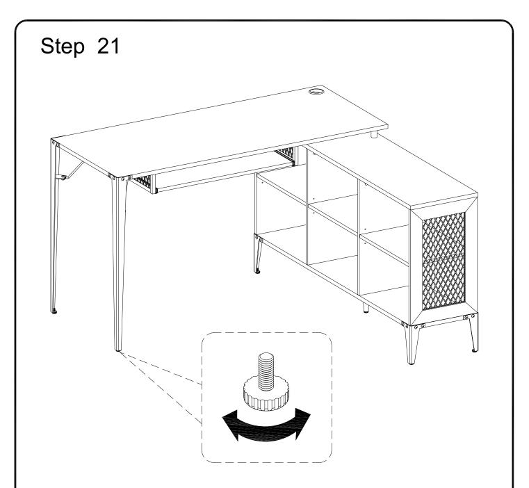
Position the assembled unit at the desired location ,if necessary adjust the floor leveler at the bottom of the support leg to level the unit .
