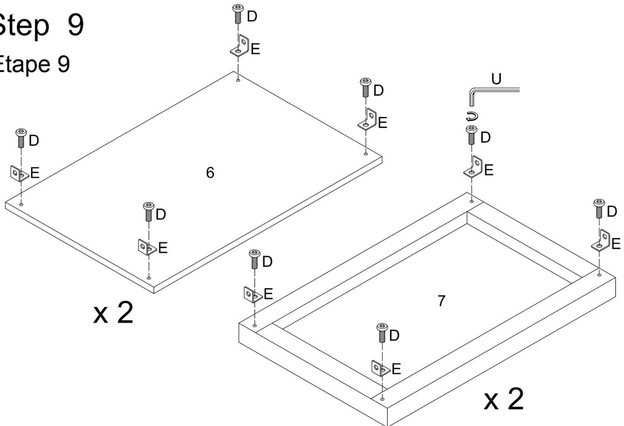
Use wrench (U) and bolts (D) to secure the L shape bracket (E) to the shelving board (6, 7).
