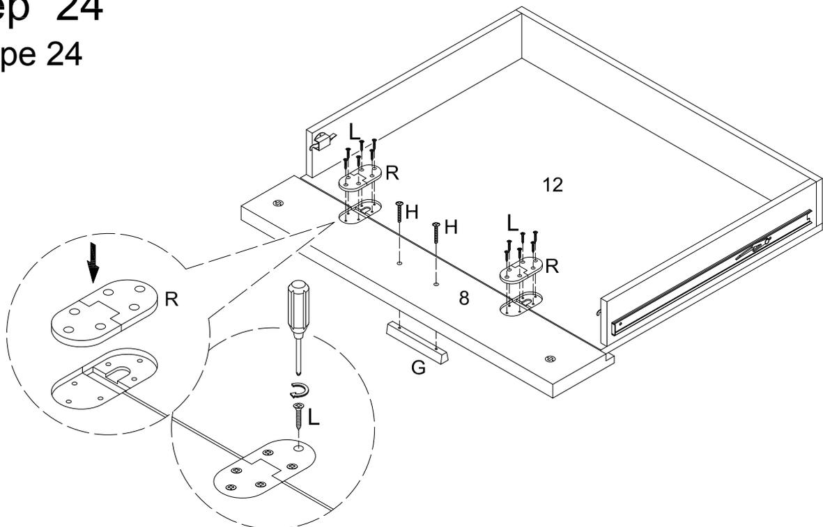
Use screws (L) to secure Hinge (R) to drawer front panel (8) and drawer bottom panel (12).
