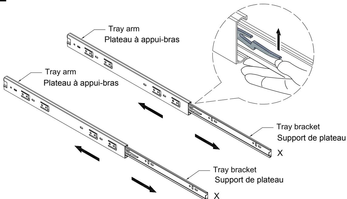
Disassemble keyboard tray slider (X) by sliding the tray arm and tray bracket apart. Depress the small lever of the tray bracket and carefully pull the two pieces apart. Repeat this process for both keyboard tray sliders (X).
