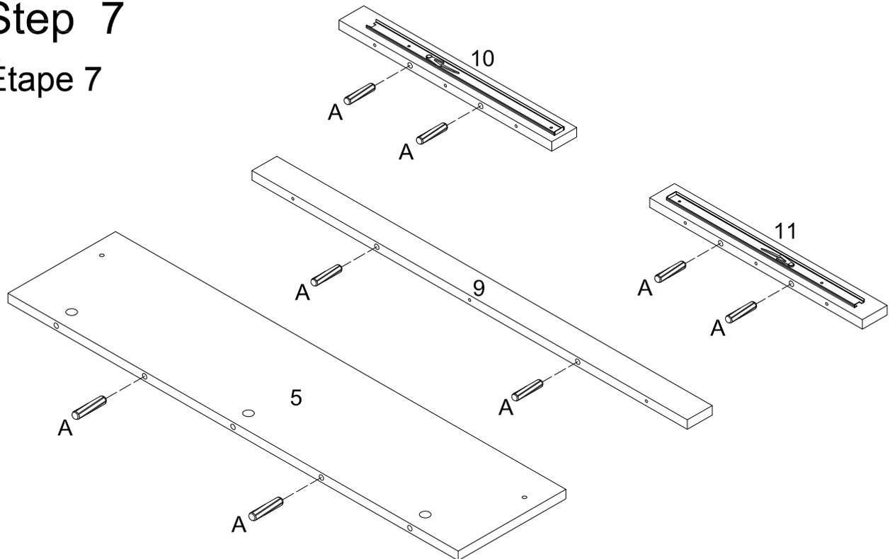
Insert wooden dowels (A) into back panel (5) and drawer panels (9, 10, 11).
