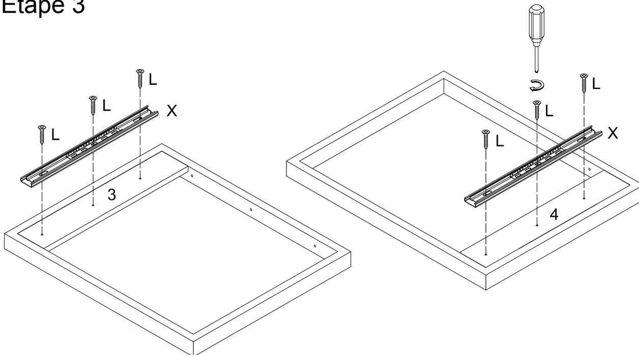
Secure screw (L) to the tray arm of keyboard tray slider (X) to the middle side panel (3,4).
