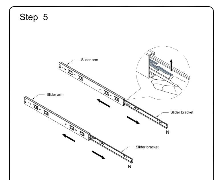
Pick up the slider arm (N) and separate the slide Runner for the following Steps. Extend the Slide .Runner all the way forward, press the plastic release lever of the slider arm up and pull the Slide Runner Complete out .
