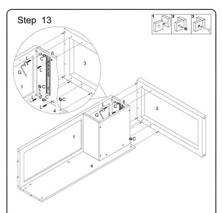
Using cam lock(C) secure part (3) to parts (1,4) with Philips head screwdriver, then using bolt (L) attach part (6) to part (3) with Hex key (G) as per diagram.
