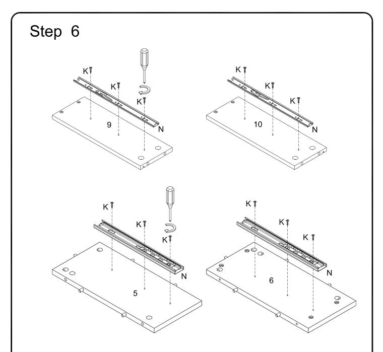
Using screw (K) attach slider (N) to parts (5,6,9,10) with Philips head screwdriver as per diagram.
