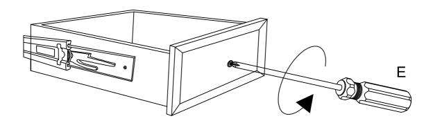
Open the drawer and remove the handle and accessories with a screwdriver.
