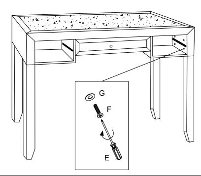
Place the table 1 and the table 2 in the correct position. Use the screwdriver F and the Bolt G and the gasket H to fix the table.
