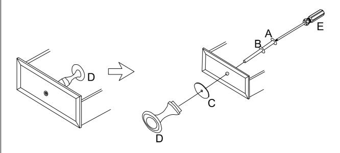
Place the accessories in the order shown above. Use a screwdriver to secure the handle to the outside of the drawer.
