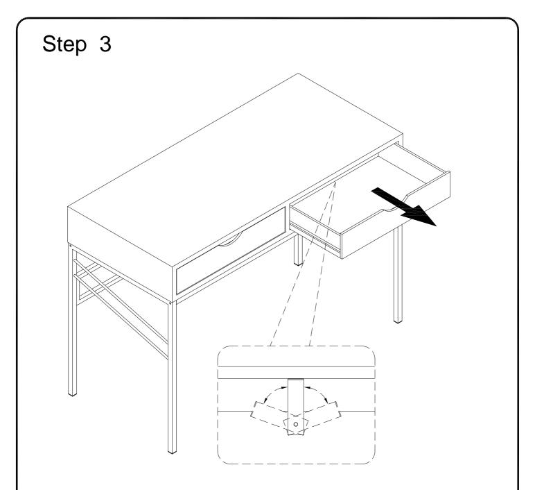
If you need to remove the drawer, please pull the drawer forward and turn the plastic stopper to left or right side ,then you can take drawer out easily as per diagram.
