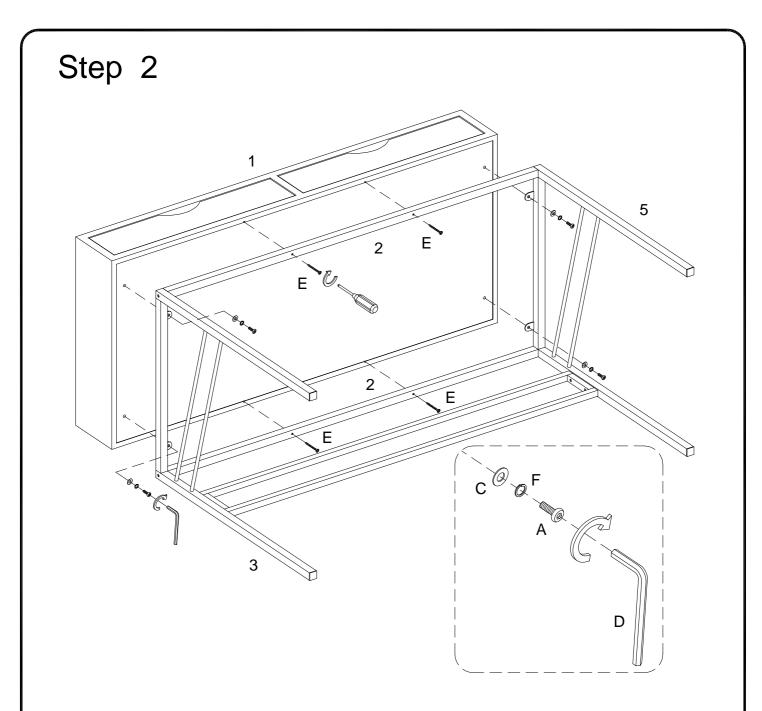
Using bolt (A) attach lock washer (F) and flat washer (C) into parts (3,5) to part (1) with Hex key (D) ,then using screw (E) secure part (2) to part (1) with Philips head screwdriver as per diagram.
