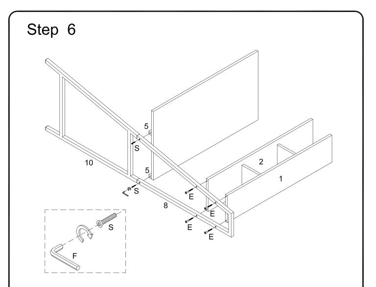
Using screw (S) attach parts (8,10) to part (5), then using screw (E) attach parts (8) to parts (1,2), with hex key (F) as per diagram.
