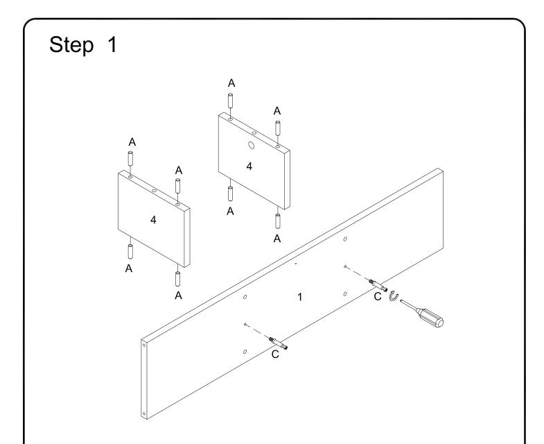
Insert wooden dowel (A) into part (4) ,then secure cam bolt (C) into part (1) with Philips head screwdriver as per diagram.
