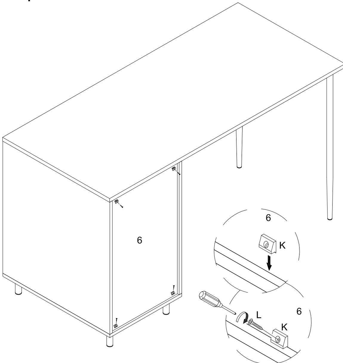
Using screw (L) secure plastic wedge (K) to part (6) with Philips head screwdriver as per diagram.
