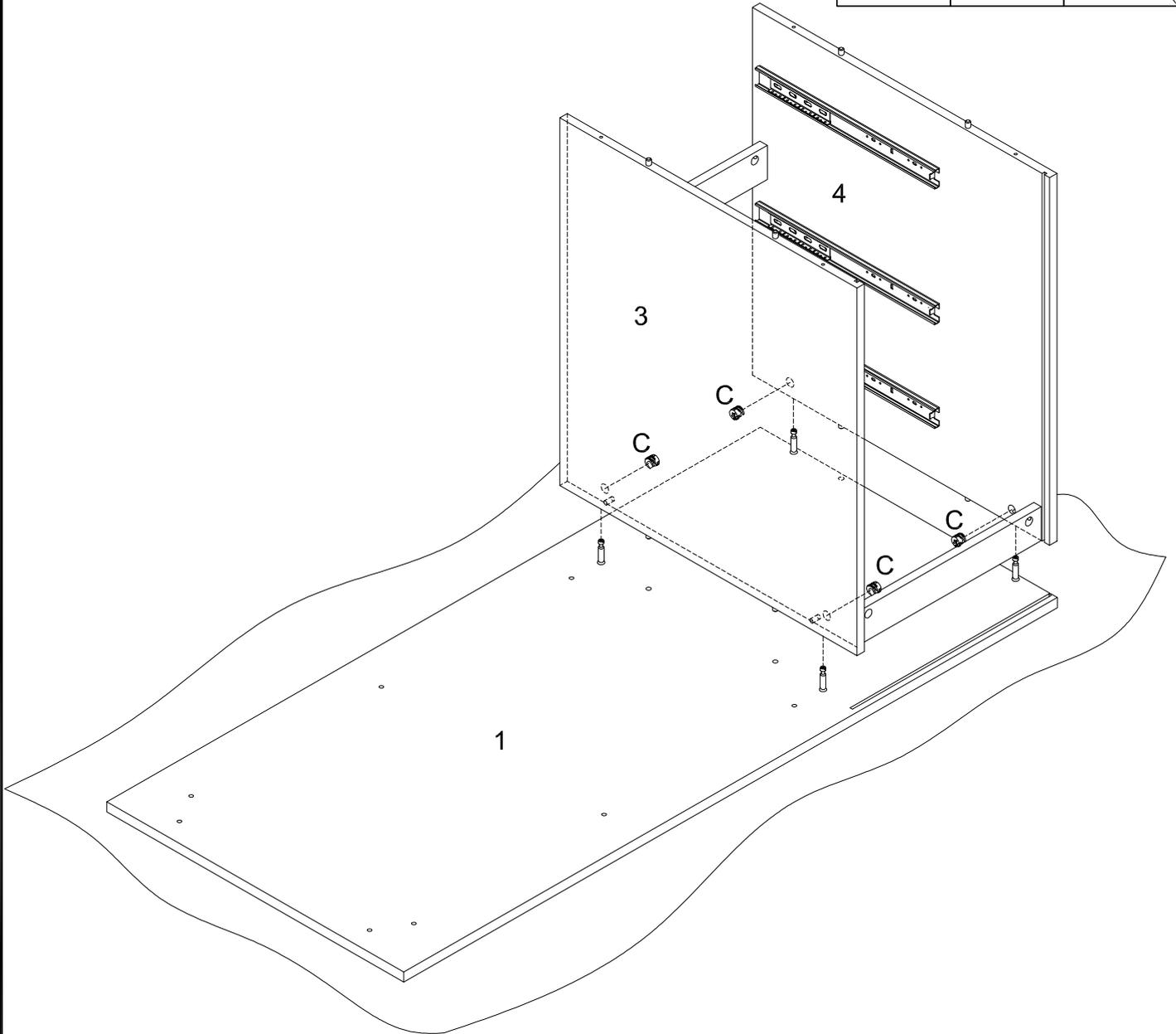
Using cam lock(C) secure parts (3,4) to part (1) with Philips head screwdriver as per diagram.
