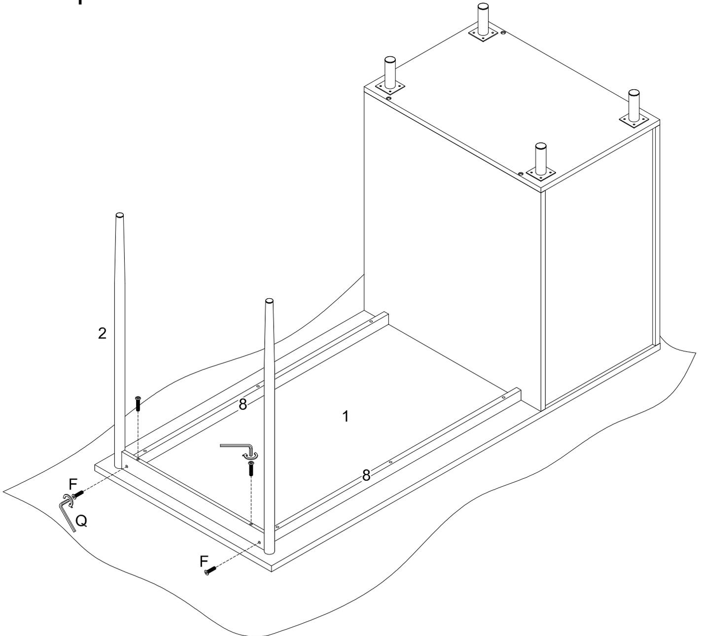
Using bolt (F) attach part (2) into parts (1,8) with Hex key (Q) as per diagram.
