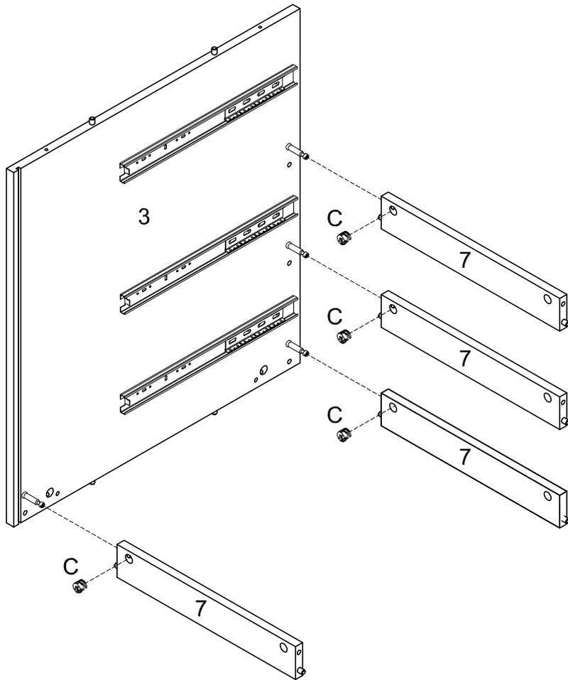
Using cam lock(C) secure part (3) to parts (7) with Philips head screwdriver as per diagram.
