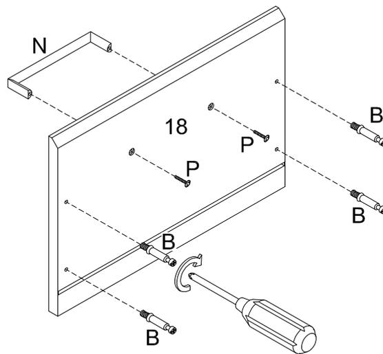
Secure cam bolt (B) into parts (13,18) and using bolt (P) attach parts (13,18) to handle (N) with Philips head screwdriver as per diagram.
