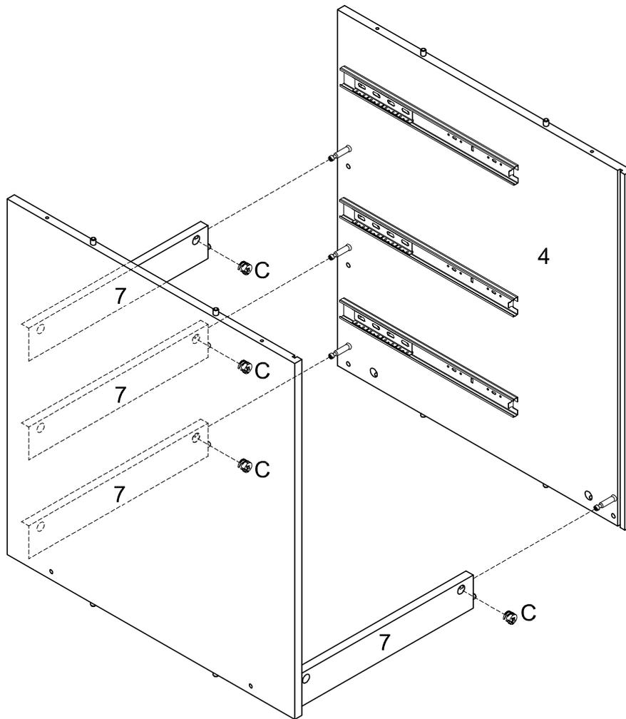
Using cam lock(C) secure part (4) to parts (7) with Philips head screwdriver as per diagram.
