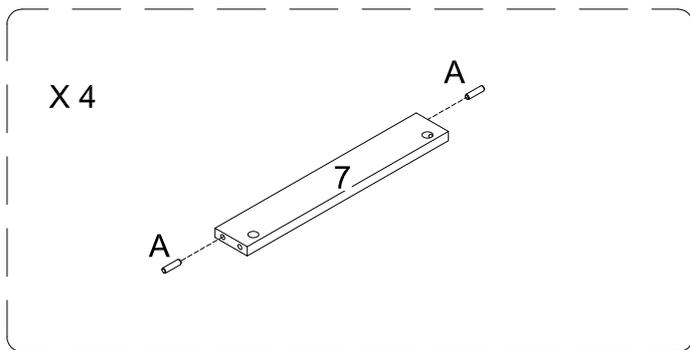
Insert wooden dowel (A) into parts (3,4,7) as per diagram.
