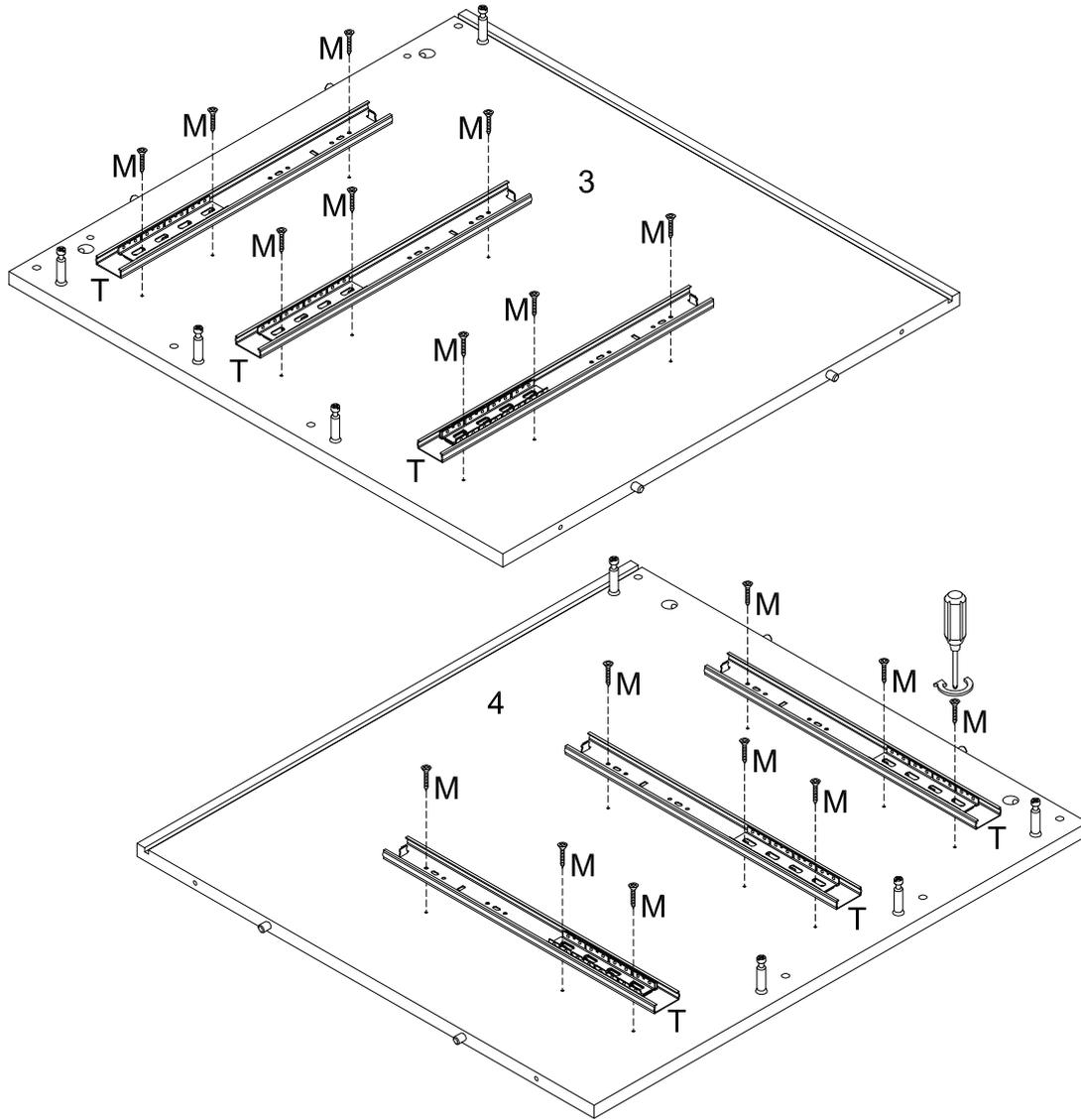
Using screw (M) attach drawer slider (T) to parts (3,4) with Philips head screwdriver as per diagram.
