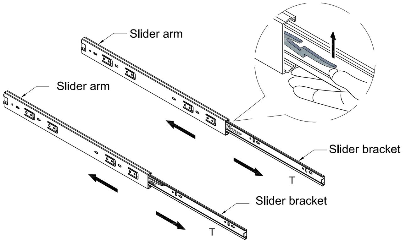
Pick up the slider arm (T) and separate the slide Runner for the following Steps. Extend the Slide .Runner all the way forward,press the plastic release lever of the slider arm up and pull the Slide Runner Complete out .
