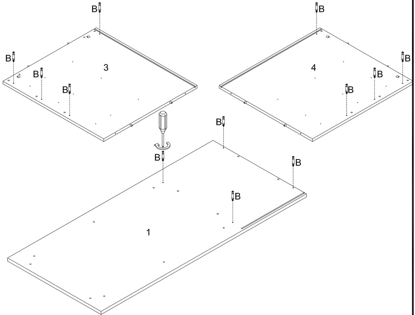
Secure cam bolt (B) into parts (1,3,4,) with Philips head screwdriver as per diagram.
