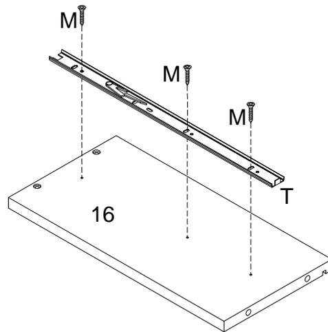
Using screw (M) attach drawer slider (T) to parts (10,11,15,16) with Philips head screwdriver as per diagram.
