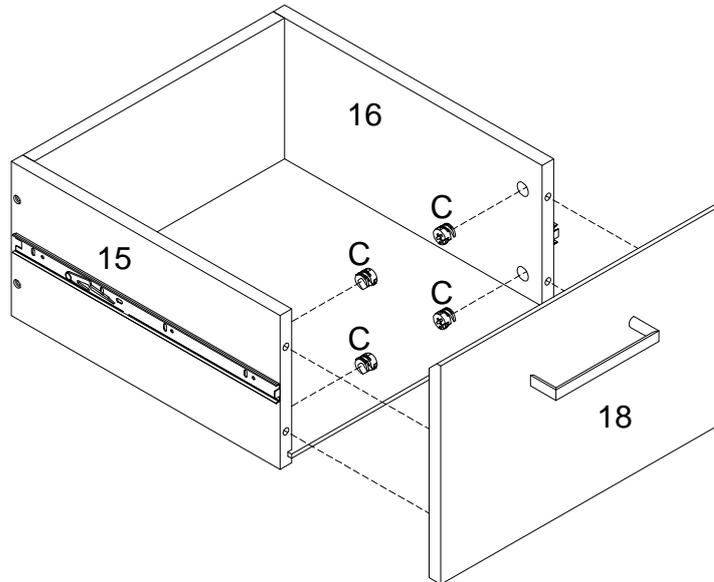
Using cam lock(C) secure part (13) to parts (10,11) ,part (18) to parts (15,16) with Philips head screwdriver as per diagram.
