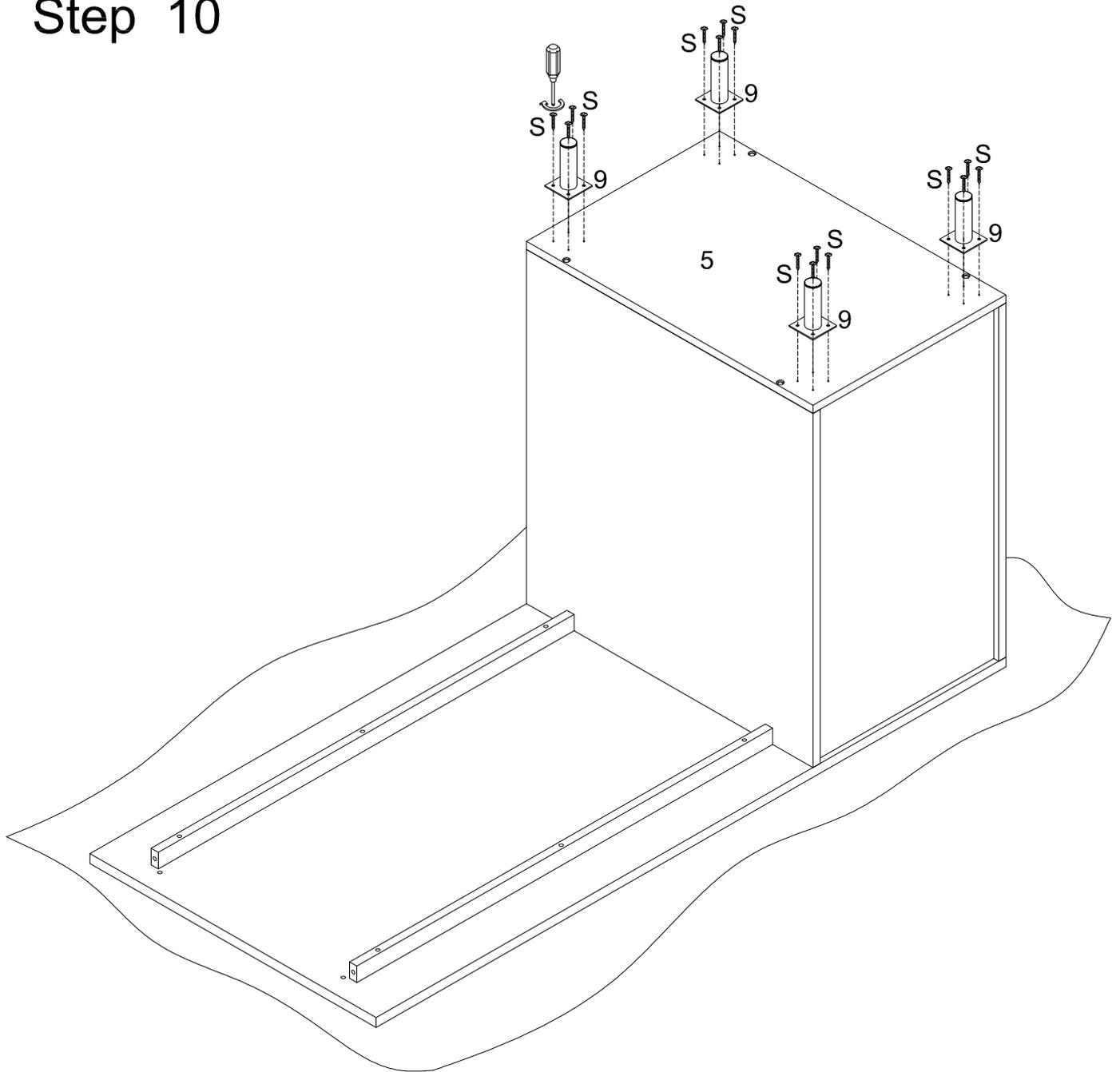
Using screw (S) attach parts (9) to part (5) with Philips head screwdriver as per diagram.
