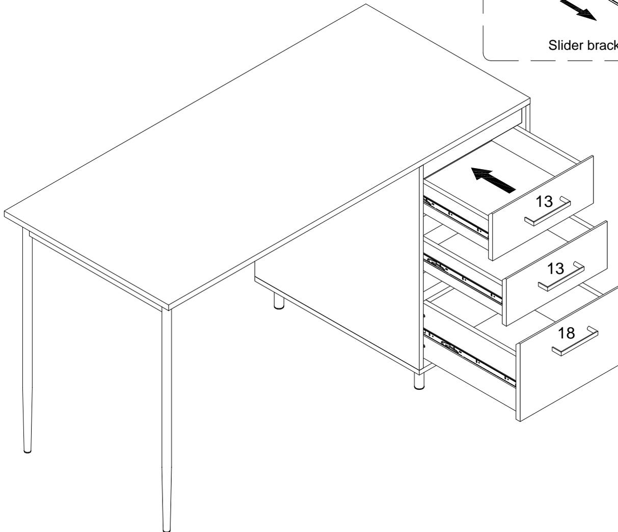
Insert the assembled drawers into the unit frame, extend the Ball Bearing Slide Tracks (T) on the pedestal Side Panel all the way forward .Then align the Slide Runners on the assembled drawers with the Slide Tracks and push the drawer carefully inside until it stops.
