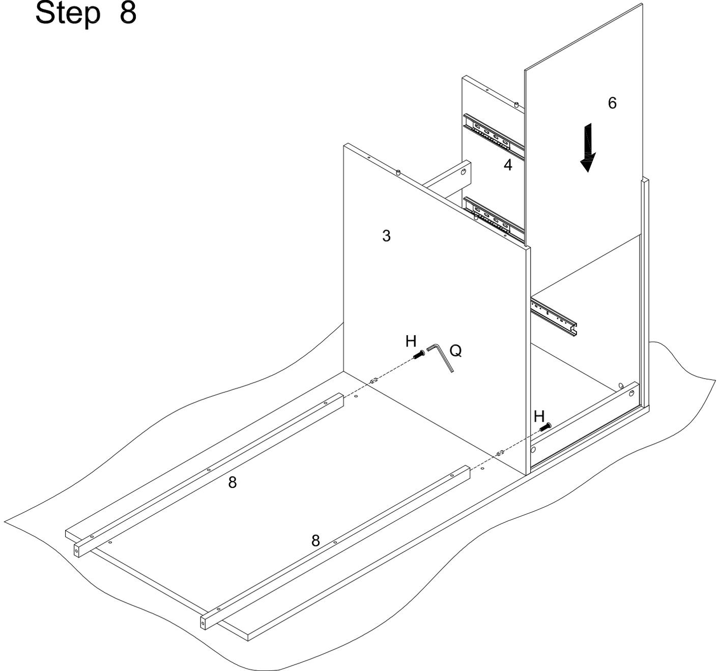
Using bolt (H) attach part (3) to part (8) with Hex key (Q) , then put part (6) as per diagram.
