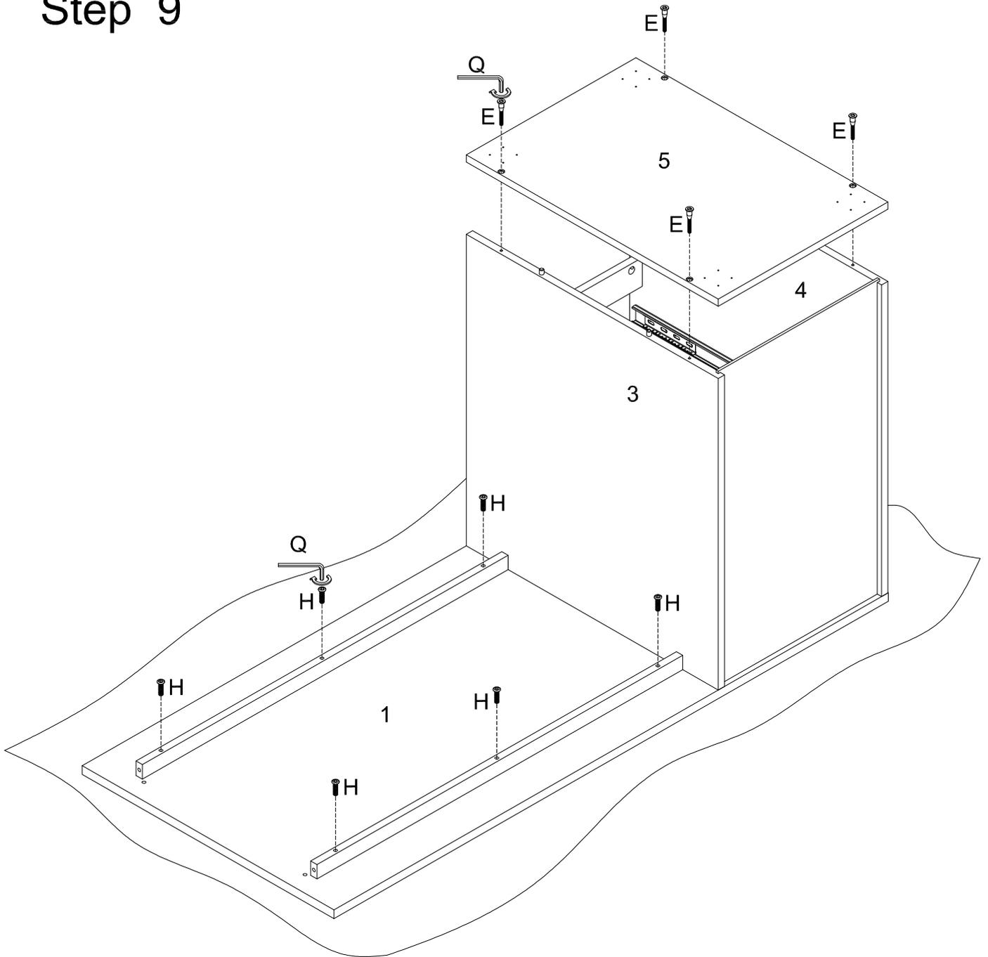
Using bolt (H) attach part (8) to part (1) , bolt (E) attach part (5) to parts (3,4) with Hex key (Q) , then put part (6) as per diagram.
