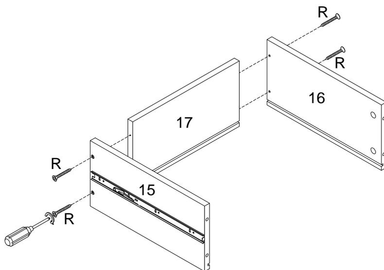
Using screw (R) attach parts (10,11) to part (12), parts (15,16) to part (17) with Philips head screwdriver as per diagram.
