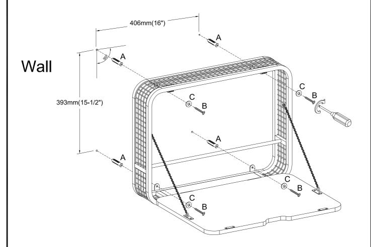
Using screw (B) attach Flat washer (C) to unit into Anchor (A) to wall with Philips head screwdriver as per diagram.
