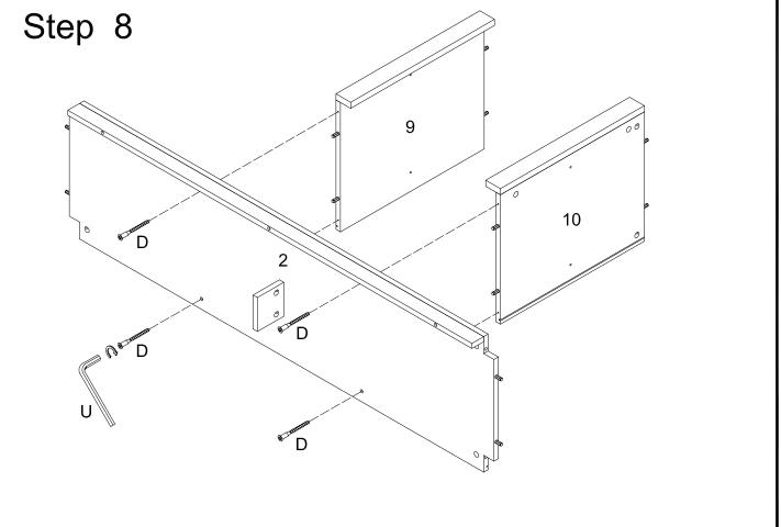
Use the wrench (U) to use bolts (D) to connect parts (9) and (10) to part (2).
