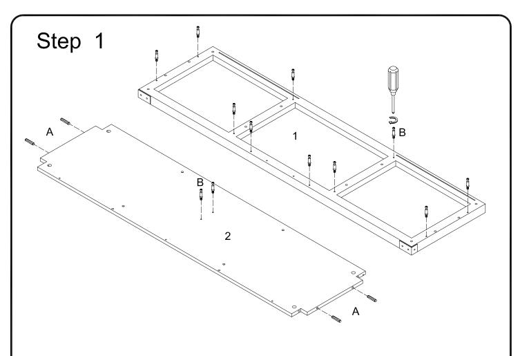
Attach cam bolts (B) to parts (1) and (2). Insert wooden dowels (A) to part (2).
