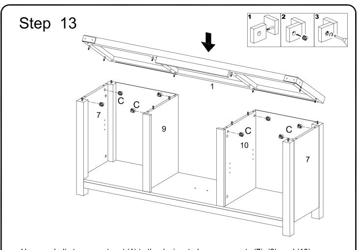
Use cam bolts to connect part (1) to the designated areas on parts (7), (8), and (10).
