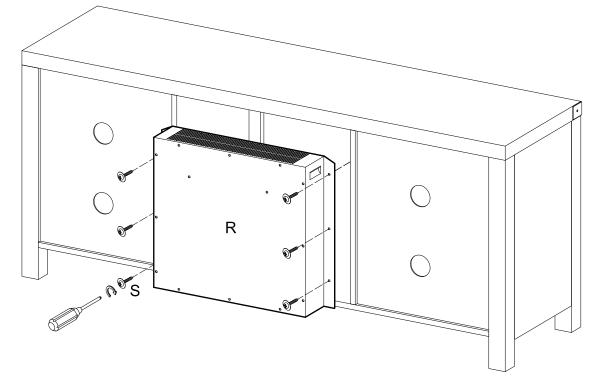
Insert fireplace (R) to the front by sliding it through the back of the unit and attach by using screws (S).
