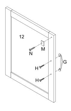
Attach handles (G) to the doors (11,12) by using bolts (H). Attach metal part (M) to the doors (11,12) by using screw (N).
