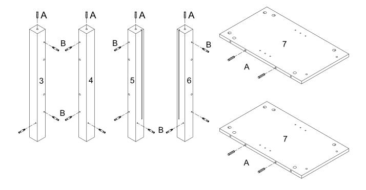
Insert wooden dowels (A) into designated areas in parts (3, 4, 5, 6, 7). Attach cam bolts (B) to parts (3, 4, 5, 6).
