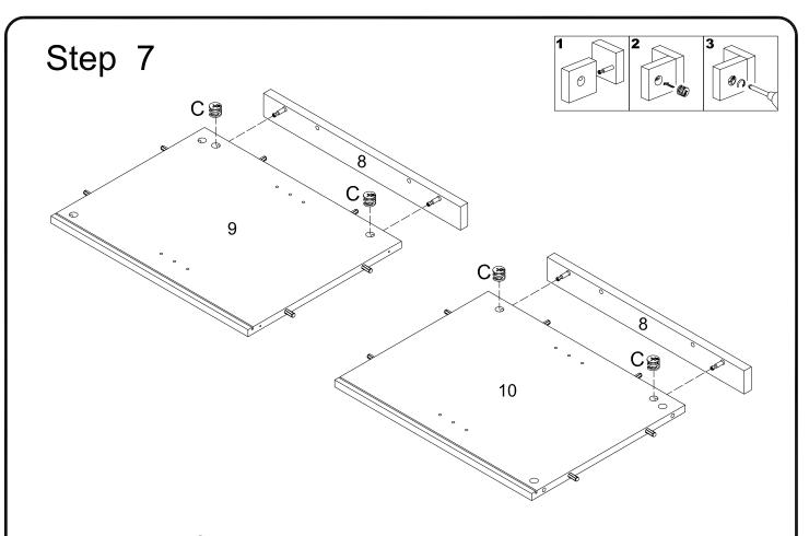
Attach cam locks (C) to part (8) to connect part (9), and to part (10) to connect to the other part (9).
