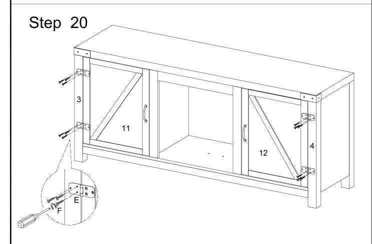
Attach hinges (E) by using screws (F).
