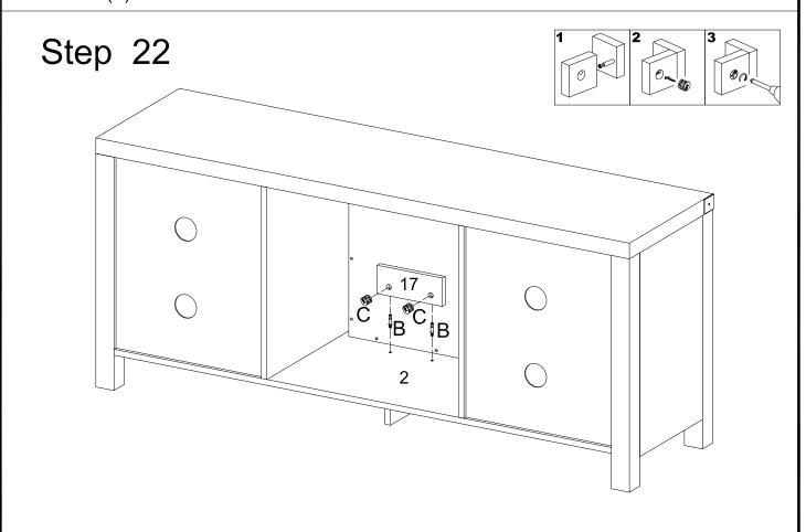
Attach part (17) above part (2) behind the fireplace unit by using cam bolts (C) and bolts (B).
