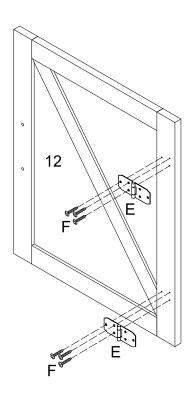
Attach hinges (E) to the doors (11,12) by using screws (F).
