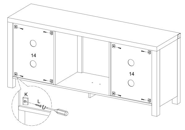
Attach the plastic wedges (K) by using the screws (L) onto the corners of parts (14).
