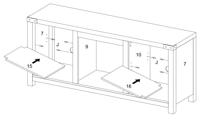
Slide part (15) between parts (7) and (9). Slide part (16) between parts (10) and (7). Attach shelf support pins (J).
